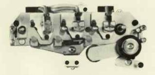
**REMOVABLE CROWN HEAD ASSEMBLIES** Rugged long life head assemblies featuring hardened, plated steel guide posts, exclusive swing arm glass tape rods, and hyperbolic heads solid precision three point, shock absorbing head mounting. CROWN uses no springs or levers to control head alignment. Also used are molded cables and a long-life nylon bristle pressure brush.
