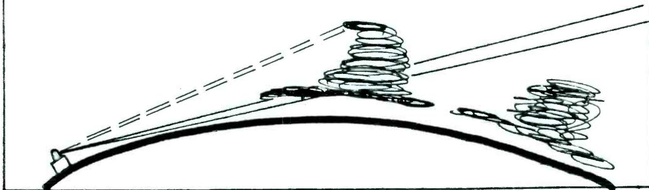
In this example you can see that low altitude clouds will not show on the radar scope until they are within the line of sight that the radar must have. These are typical formations in the fall and winter months. Most clouds that produce snow are low altitude clouds.
