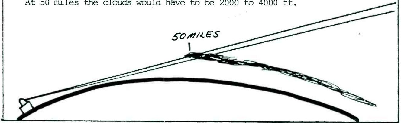
Line of sight distance from radar antenna.
