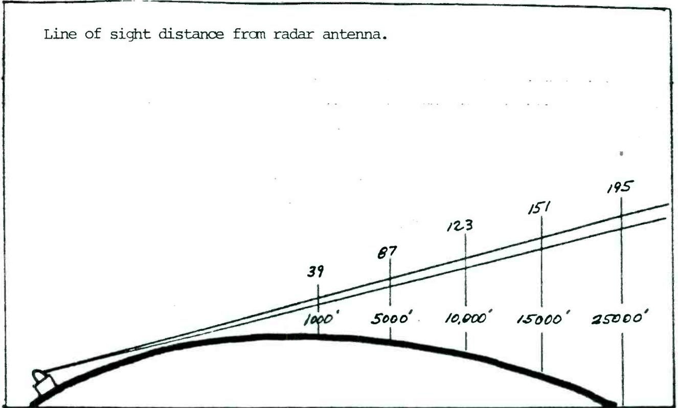
"Ducting" or SUPER REFRACTION of radar beam.
