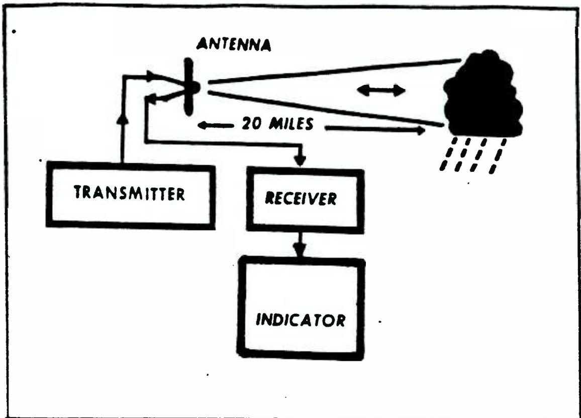
FUNDAMENTAL OF HOW WEATHER RADAR WORKS.
