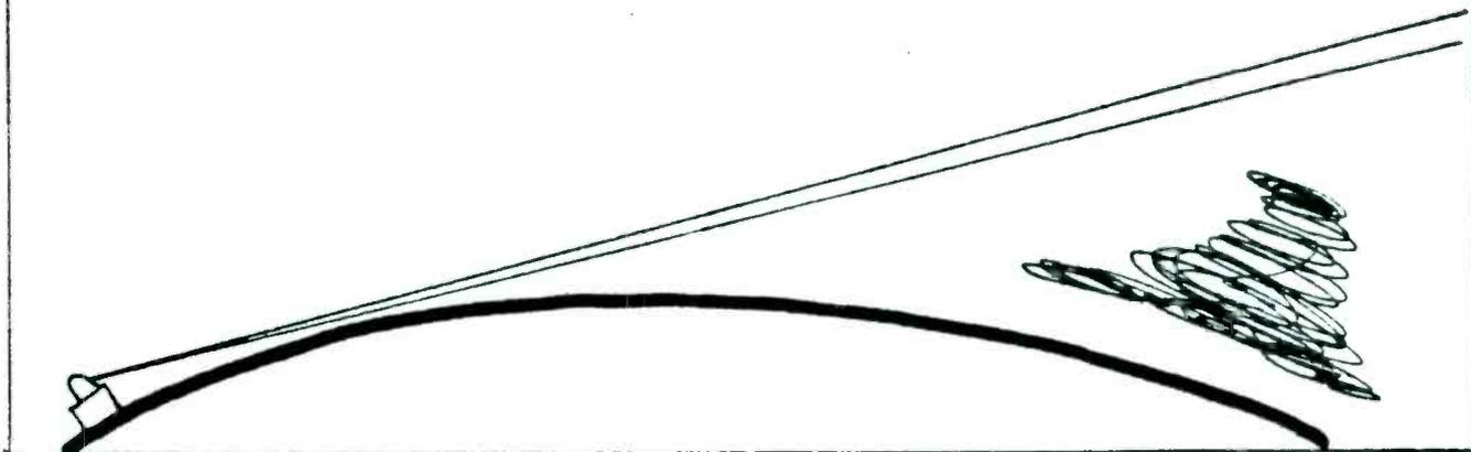
The storm cell and the leading edge of low altitude clouds are within view of the radar. However, the cell following the first one can not be seen because it is not tall enough. The dash lines indicate the radar beam when it is tilted to find the top of the cell.
