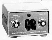
Your CW transmissions will be 100% copy with the HD-1410, because sending code is easy. whether you're operating base or portable. The dot and dash paddles travel and tension are easily adjustable. When the two paddles are treated as one, the HD-1410 operates like a singlepaddle keyer with dot and dash memories, lambic operation forms most characters with reduced wrist movement. Dots and dashes are self-completing and always in proper propor-
