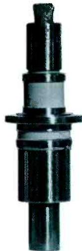
Figure 2 — Machlett ML-471, planar triode, achieves life increase of 50%, or more, operating at an E_f of 5.9 \pm .2 volts in Type 149-S Beacon employing the ACF Model 331 cavity. Excellent cathode activity permits pulsed power emission of 11 amps cm^2 .
