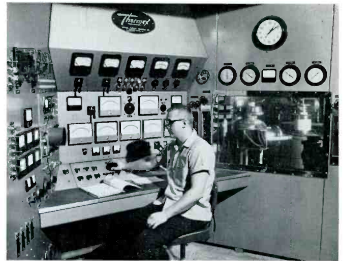
Figure 4 — Control panel area showing ease with which test operator can view both tube under test and control panel metering.
