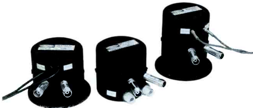
Figure 1 — Three Raytheon CW Amplitrons developed for communications. Shown (left to right) are the QKS997A, QKS1051, and the QKS1119.
