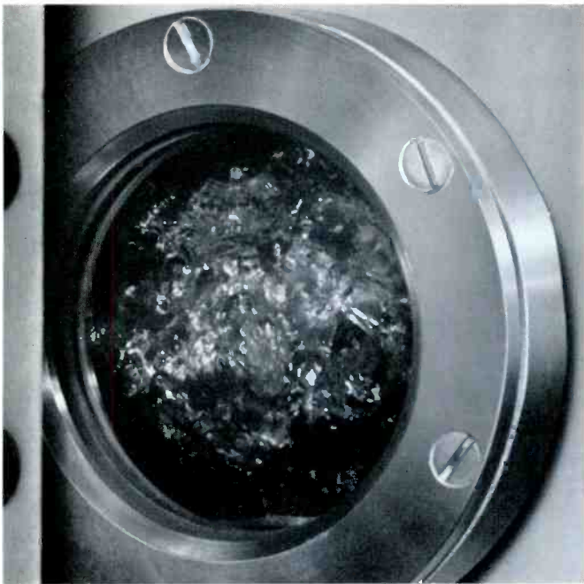
Figure 3 — Closeup of porthole shown in Figure 1 with tube operating at 200 Kw plate dissipation.
