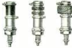
This series of variable inductors offers a higher Q coil with a slightly larger inductance range than can be obtained in either of the two smaller series. The same high grade silicone-impregnated ceramic forms are used in their construction to insure a product of high quality. These coils mount by means of a bushing that requires a 1/4" diameter mounting hole. Hardware consisting of nut, lock washer, and spring clip is supplied.
