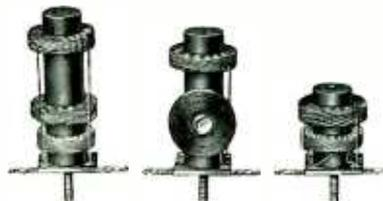
Single section, duo-lateral wound, Litz wire secondary. High impedance primaries. Wound on impregnated ceramic dowels and provided with a bakelite terminal plate. For use with a .000365 mfd. variable condenser. ABP type combines antenna and
