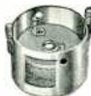
Series 800 shielded iron core chokes are similar in construction to the type 900 unshielded chokes. The shielded chokes are enclosed in round aluminum shields provided with two #6-32 spade bolts for easy assembly to the chassis. Shields have a satin finish. Inductances are accurate to within five per cent.
