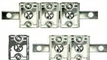
Ideal for trimming the high frequency end of multi-band circuits, these trimmers are available in single to quadruple section types. Ceramic insulation and mica plate spacer insures low-loss operation. The dimensions per section are 3/8" wide by 3/4" long. Terminals are plated for easy soldering.
