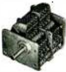
These midget variable condensers have the same precision construction as our standard series and will find ready application in the construction of portable and compact receivers of all types. Split outer plates on the rotors permit accurate alignment. High frequency trimmers are provided on the short side of the condenser. Mounting is provided by tapped holes in the frame of the condenser. Maximum rotor swing is 1". Counter-clock rotation for capacity increase. Shaft is 1/4".
