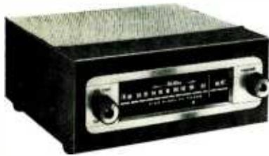
A carefully designed high quality tuner featuring excellent performance and distinctive styling at a moderate price. Many features of the Miller 560 FM tuner are found only in more expensive units. The circuit consists of a grounded grid R.F. amplifier, two I.F. stages, one limiter stage, and a Foster-
