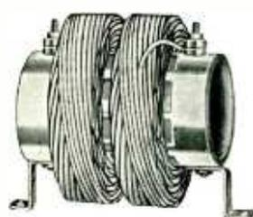
Duo-lateral wound chokes designed for use in the tower lighting circuits of broadcast and commercial transmitter antenna towers. These chokes offer high impedance to radio frequency and have extremely low distributed capacity. Low power-frequency reactance and DC resistance insure minimum lighting power loss. The chokes are wound on ceramic forms and the windings are of the two-pi sectional type and are protected by a baked glyptal varnish. One
