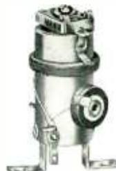
This coil may be used for almost all types of capacity operated electronic devices such as alarm systems, show windows, counter displays, novelties, etc. The coil is a center-tapped oscillator winding with an adjustable grid coupling condenser and an r.f. choke, all assembled on a bakelite form. A typical wiring diagram is supplied.
