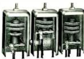
A compact series of radio frequency and oscillator coils well suited to the needs of the constructor of aircraft, marine and midget broadcast receivers. The coils are of the iron core type and are enclosed in satin finished aluminum shields. Standard antenna coil primaries are of the low impedance close coupled type for use on short vertical or
