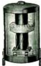
These untuned antenna and radio frequency coils are broadly self-resonant throughout the standard broadcast band from 540 to 1700 KC. They are used mostly in AM High-Fidelity Tuners. They may be used for increasing the sensitivity of small receivers by merely adding the coil and a radio frequency amplifier tube. The coils are shielded in aluminum cans and are provided with the #6-32 spade bolts for assembly to the chassis.
