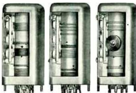
Three band all-wave coils similar in construction to our Series 628 and for use with a 455 KC intermediate frequency amplifier. High frequency trimmers are provided for each band and are accessible for adjustment through holes in the side of the shield. All windings are thoroughly impregnated for protection under all climatic conditions.
