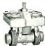
A compact double tuned, unshielded intermediate frequency transformer which will find wide application as a replacement for many receiver types using odd shaped transformers which may not be readily available. Particularly useful in compact and midget AC-DC receivers. Since the windings are mounted in a horizontal axis, considerable space is saved. Overall dimensions only 1 3/8" square by 1 1/2" high. Single #6/32 machine screw mounting.
