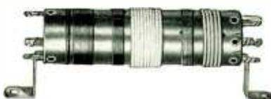
A series of compact unshielded three band coils for use by experimenters in constructing custom-built short wave receivers to satisfy individual requirements. When used with a 365 mmfd. variable condenser, the frequency range is as follows:
