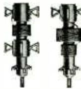
Their small physical size and the fact that they can be adjusted to the inductance required, make these coils ideally suited for replacement in broadcast band receivers. Antenna and R.F. coils have high impedance primaries and high-Q Litz wire wound secondaries for use with any variable condenser having a maximum capacity between 250 and 450 mmf.
