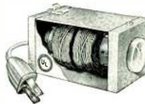
Designed to eliminate radio noises caused by small household appliances such as food mixers, sewing machines, vacuum cleaners, etc. When connected between the radio receiver and the power outlet, the filter will prevent pick-up of interference and unwanted signals through the house wiring system. When used with household appliances the filter prevents the interference energy from getting into the house wiring circuit and disturbing receivers throughout the neighborhood.
