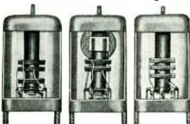
To meet the needs of the serviceman and experimenter, we have developed a series of small iron core variable inductance coils for the broadcast band. These coils are well suited for general replacement use in receivers where manufacturers' coils are no longer available. The inductance may be adjusted
