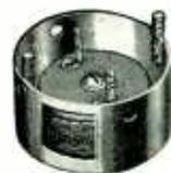
Miller Series 700 radio frequency chokes are similar in construction to the Series 600 and are assembled in aluminum shields. They are particularly useful for use in stage-isolating circuits, where coupling between chokes would be detrimental. The round shields are finished in satin okite and inductance tolerances are maintained to within five per cent. Two #6-32 spade bolts provide for simple mounting. Schematic No. 2.
