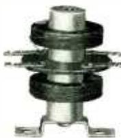
These chokes are similar to those listed above except that two duo-lateral wound coils are assembled on a single ceramic form with a bakelite terminal plate. They are for use with full wave mercury vapor rectifier tubes or with separate tubes having a maximum plate current of less than 300 MA. A two-hole mounting clip is provided. Insulation is adequate for peak voltages up to 2500. The entire assembly is thoroughly impregnated in tropicalized Q-Max lacquer.
