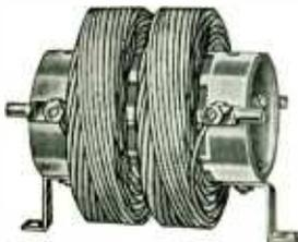
Miller Dual Duo-Lateral Line Filter Chokes are wound with two coils on one form, giving the advantage of small physical size in cases where space requirements are stringent and two single coils would occupy too much area. Identical in specifications, except for dimensions, to our single type Duo-Lateral chokes. They are wound on white ceramic forms 2" in diameter by 4½" long.
