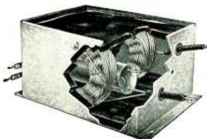
Miller industrial filters are designed for all types of radio interference producing devices and are highly effective at broadcast and short wave frequencies. The unique filter circuit, consisting of two duo-lateral wound chokes and two single layer solenoid chokes combined with two 2. mfd. non-inductive wound paper dielectric condensers.
