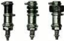
A new series of small adjustable coils designed for the most exacting requirements. Wound on silicone impregnated high grade ceramic forms. Tuning is by means of a powdered iron core. These coils require little space and are for mounting in a 3/16" diameter hole.
