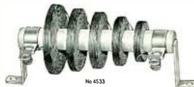
Miller Heavy Duty Navy Type chokes are recommended for use in the high power amateur transmitter and in commercial installations. They are sectional wound on ceramic forms with rigid terminal clips.
