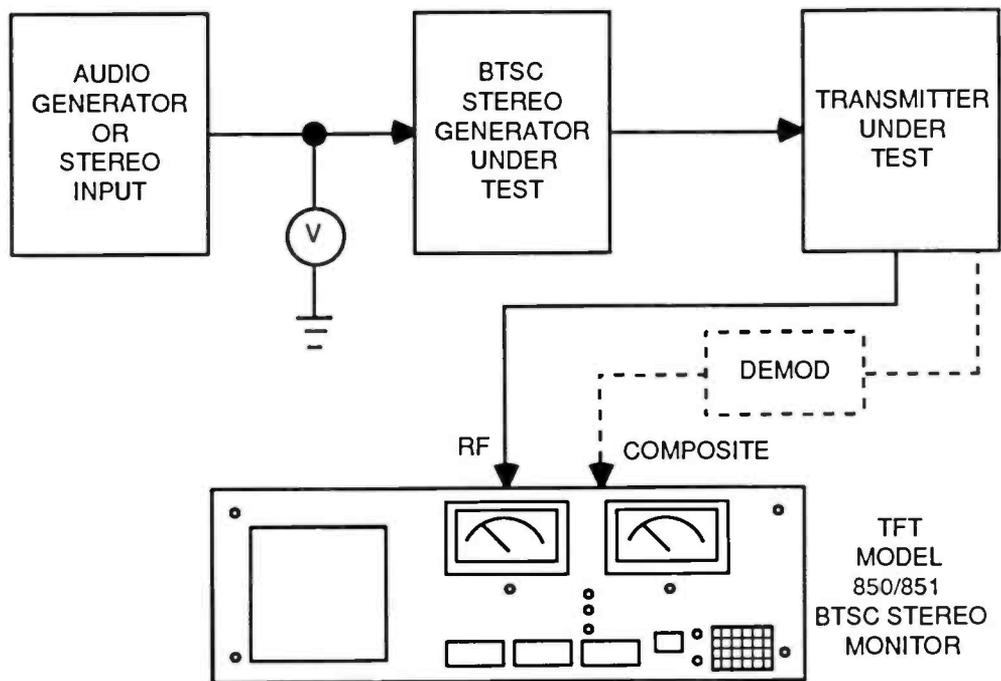
Figure 4-4: Example of Equipment Interconnections
