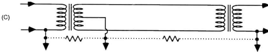
Figure 5-1C: Multiple ground connections open the door for "ground loops" that could render the measurements invalid.
