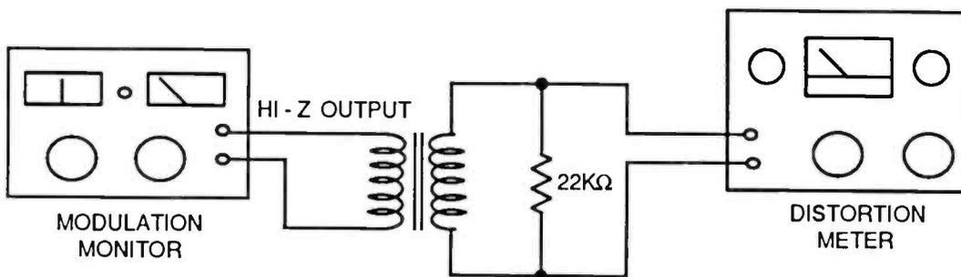
Figure 5.2: A Ground Isolation Method
