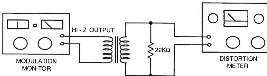
Figure 5.2: A Ground Isolation Method
