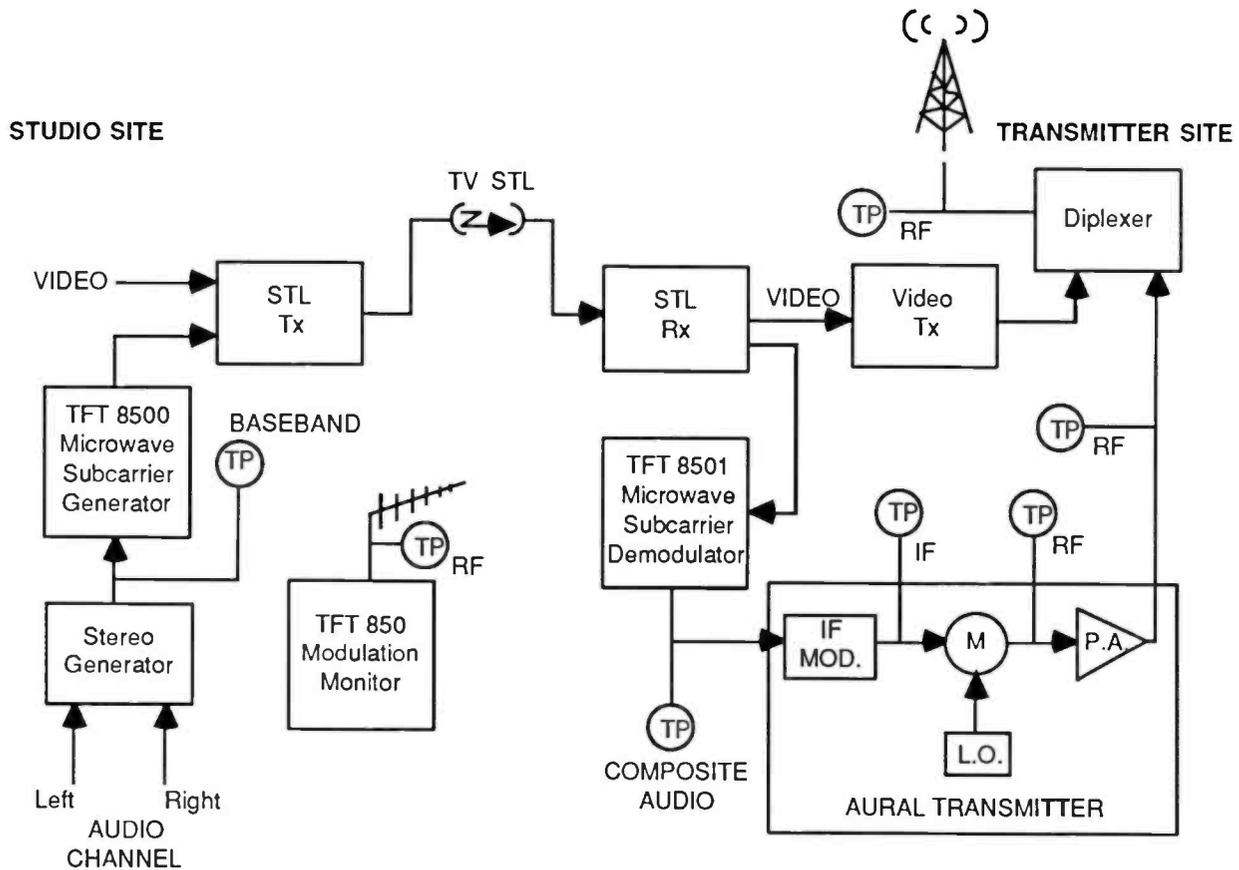
Figure 4-3: Test Points where Measurement can be Made
