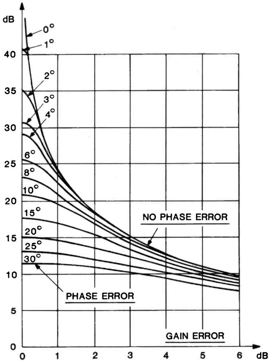
Figure 3-2: Stereo separation as a function of gain and phase errors in the L-R versus the L+R paths.
