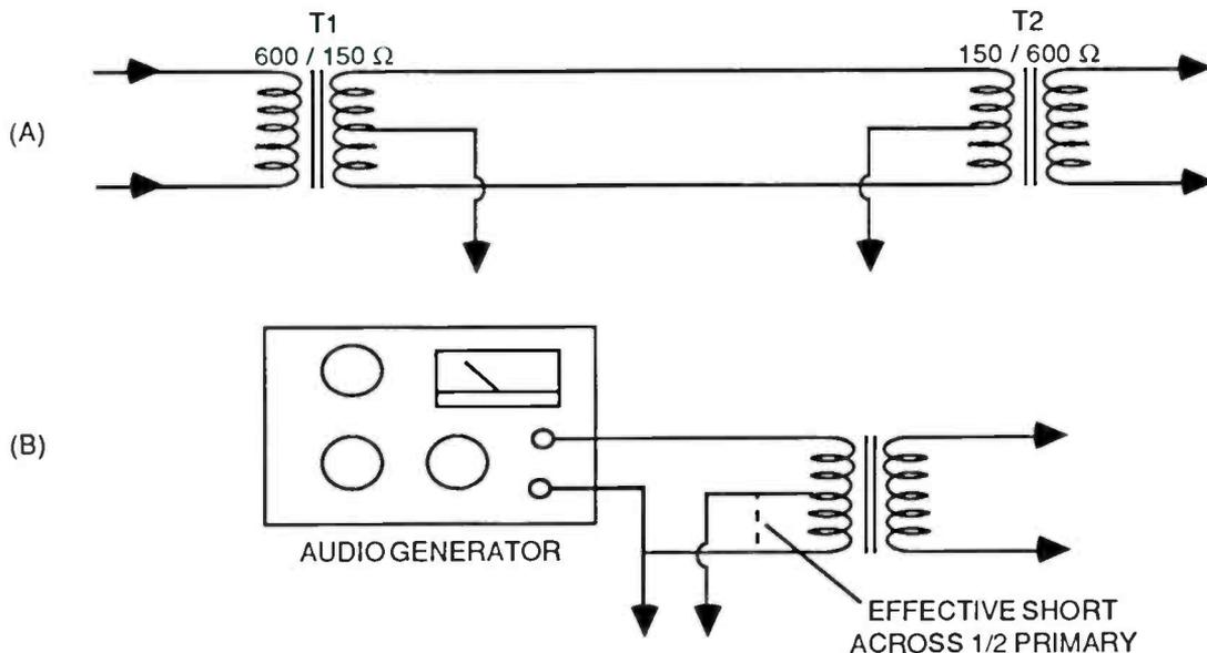
Figure 5-1A and 5-1B: Direct connection across a truly balanced input can result in severe mismatching and test conditions not simulating normal operation of the input circuit.
