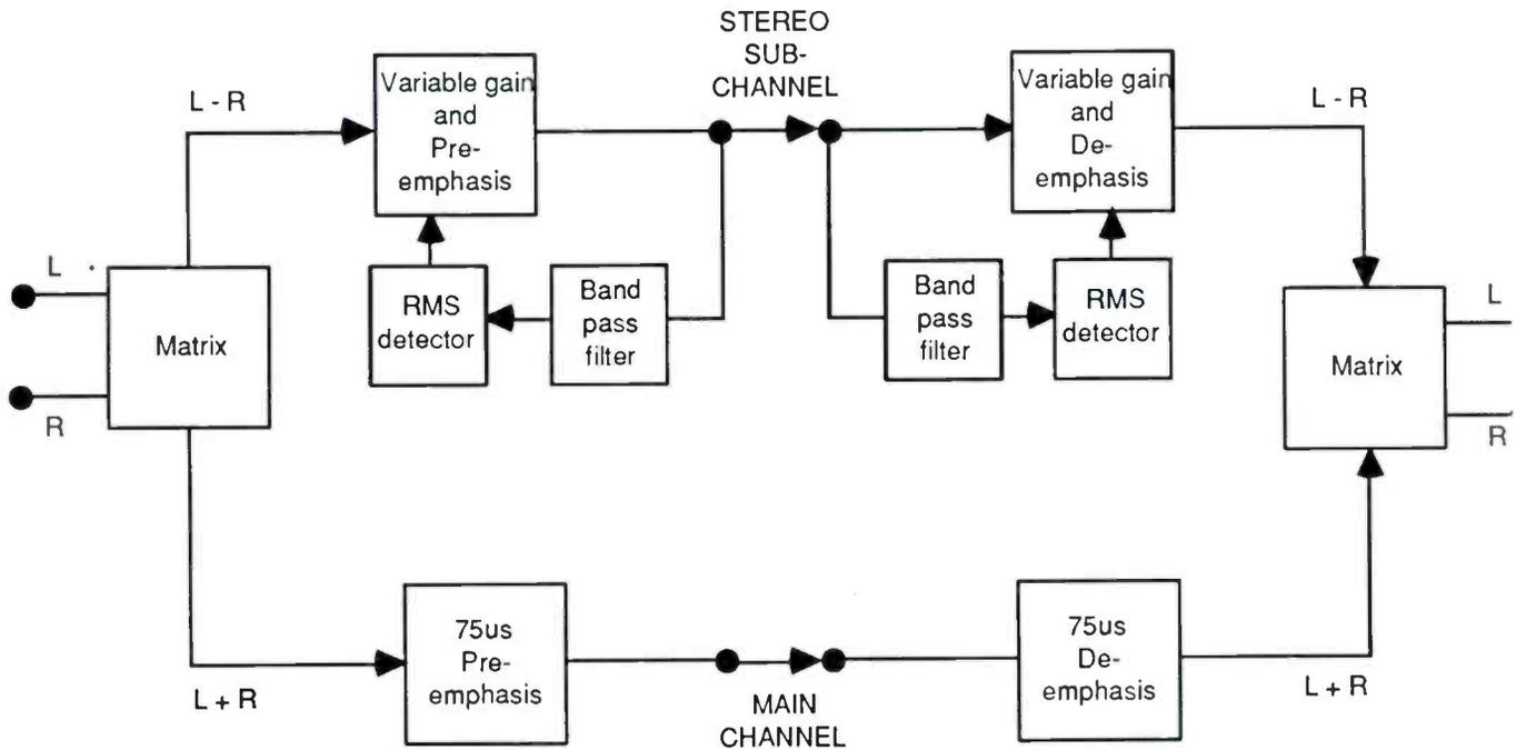
Figure 3.1: Block Diagram of the BTSC Companding System
