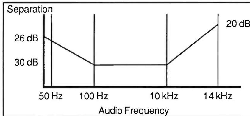
Figure 2-3: Minimum Stereo Requirement with Encoding of L-R
