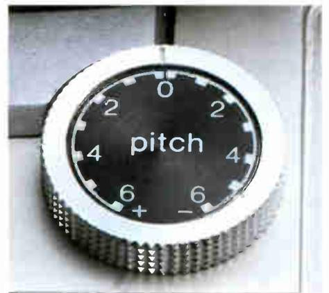
With this precision system you can match the pitch of a record to that of a musical instrument, or expand and compress playing times to fit a given broadcasting time slot.
