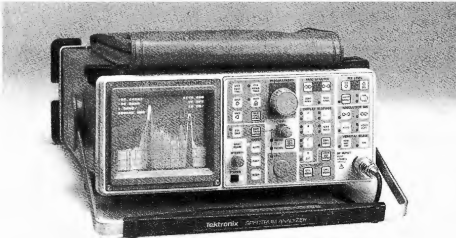
2710 Economy Portable Spectrum Analyzer.
