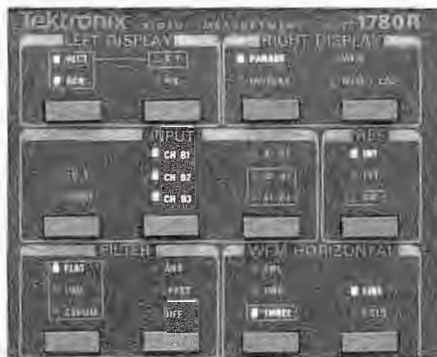
Multiple inputs and parade display mode facilitate component signal measurements.
