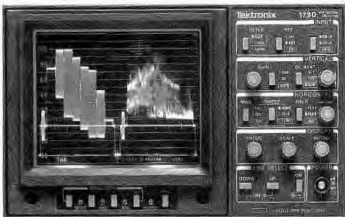
1730 Waveform Monitor — Simultaneous Channel A and B Display.
