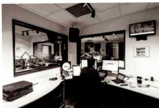
Operator at an Axia Radius 8-fader console looks into the WB AP talk studio. Telos VSet12 phone stands ready to the left
