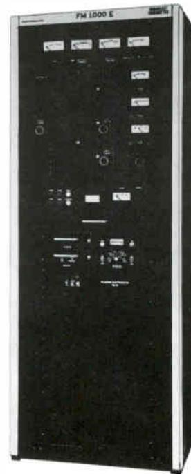
The upper meter panel indicates plate current, plate
