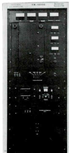
Full and complete metering is provided. To the right of the power amplifier two multimeters measure screen and control grid voltage and current. A third meter measures the incident and reflected power of the exciter output.
