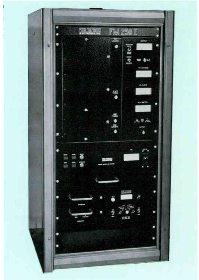
An additional drawer which houses the exciter and where required, the stereo generator is the next vertical component beneath the control circuit drawer. In addition there are two slide-out compartments in the exciter itself which facilitates exciter adjustments, but for service or maintenance on the exciter power supply, opening of the main drawer provides complete accessibility.
