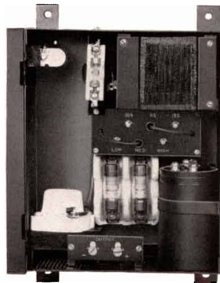
INTERIOR OF THE RECTIFIER UNIT
