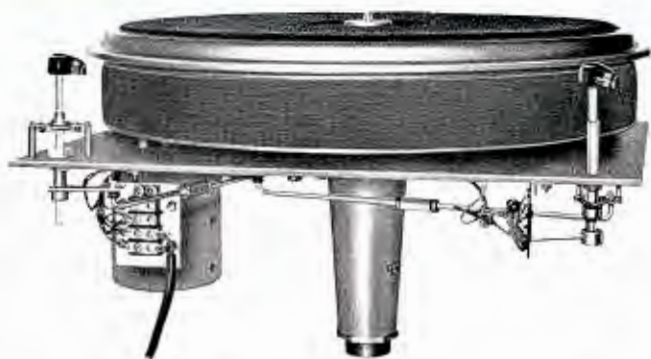
Sturdy 16-inch turntable platter with large spindle accurately machined to give many years of service. Quiet operation is provided by the cushion-mounted motor operated by a silent mercury switch.
