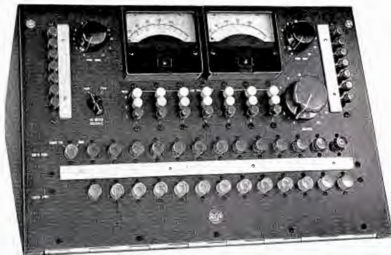
This master control panel with auxiliary microphone inputs and master and monitor gain controls, etc. was designed by RCA for Station WBNS. The console cabinet is designed for desk top mounting next to a standard BC-6B Consolette. The front panel swings out affording complete accessibility.
