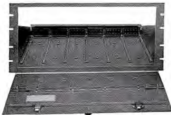
Panel removed showing guide bars and receptacles.
