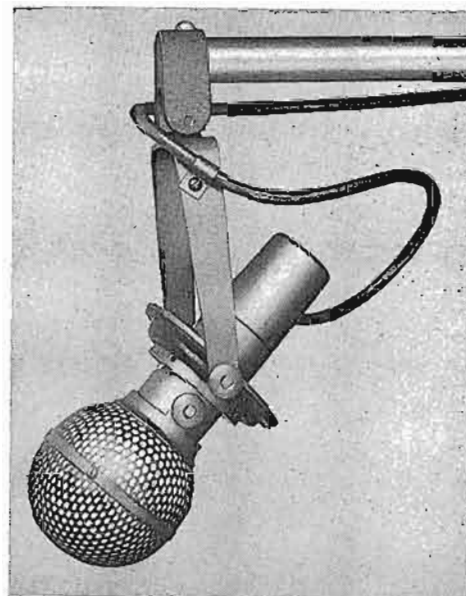
BK-5B Microphone with Wind Screen, MI-11011, and Boom Unit, MI-11012.
