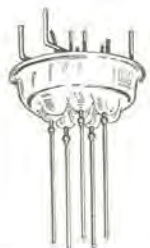
Moulded glass stem assembly showing individual lead seals.
