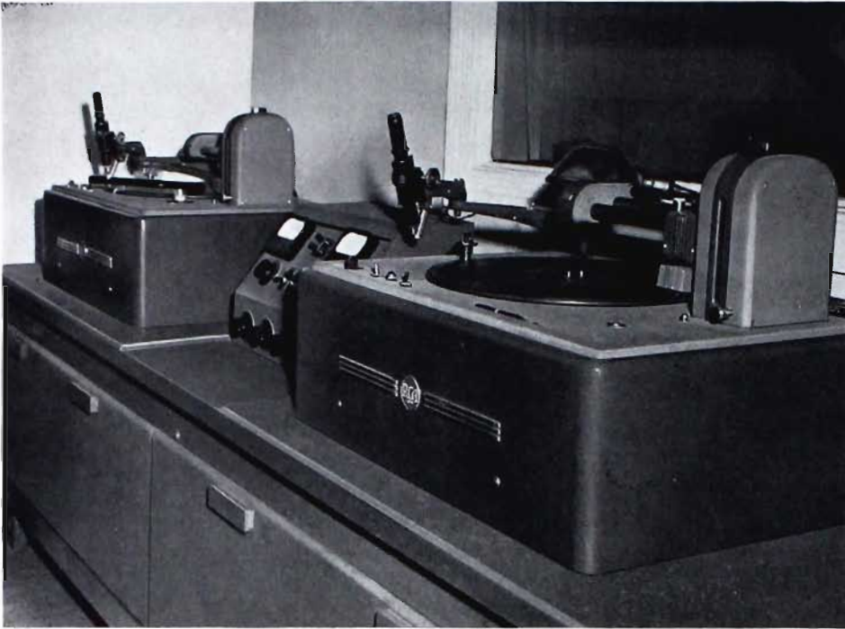
◀ Studio recording installation at KUTA, Salt Lake Cty, Utah, showing two bench-mounted RCA 73-B Professional Recorders.
