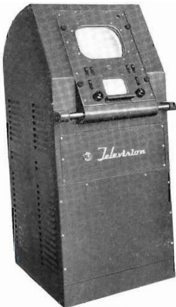
Photo above shows how TM-5A may be mounted in a special housing for portable uses
