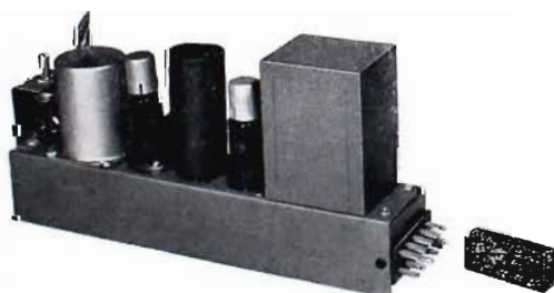
Rear view of BA-11A showing multi-contact, plug-in connection
