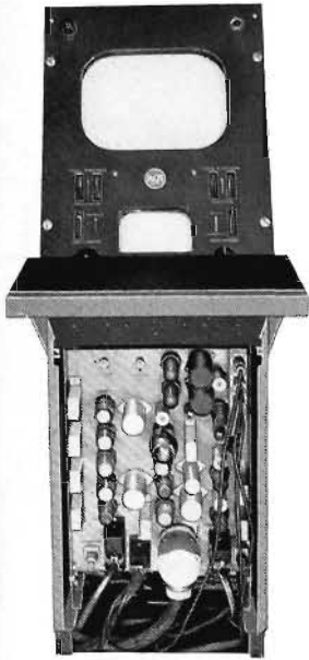
Studio Camera Control Unit consisting of TM-5A Monitor and Camera Control Chassis (MI-26055) mounted in console housing (MI-26266B)
