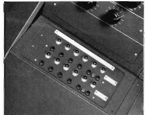
MI-26222 Master Control Panel shown mounted in sloping desk portion of TV console section.
