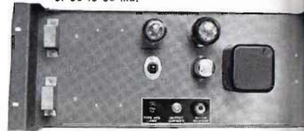
Current Regulator, MI-26090. Maintains constant current in focus coil of Studio Camera TK-10A. Current can be adjusted over a range of 65 to 85 ma.
