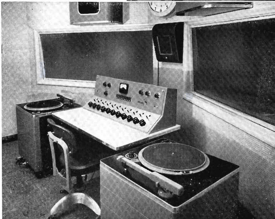
WJPG-FM, Green Bay. One of the specially-built studio-control consoles in WJPG-FM's 4-studio arrangement. Complete two-channel operation (AM and FM), simultaneous audition and broadcast from any combination of studios, remote lines, cueing and talkback are provided.
