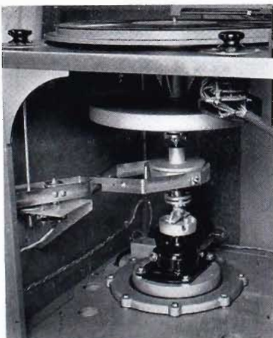
Interior view of the 70-D Turntable with 45 R.P.M. Kit installed
