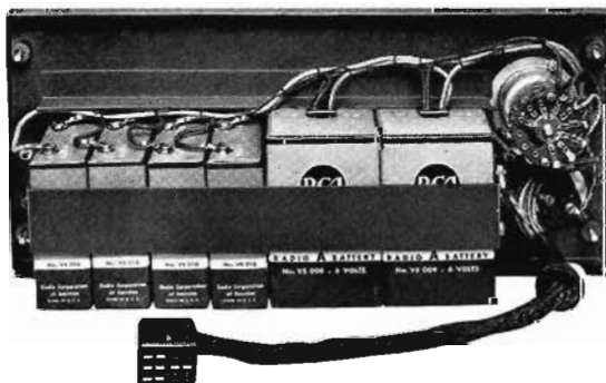
Rear view of Battery Cover showing batteries mounted in place
