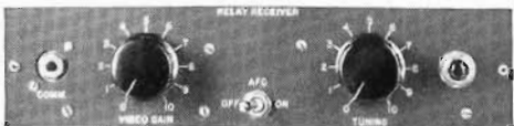
Relay Receiver Control, MI-26247. Controls video gain and receiver tuning. Includes 2 potentiometers, AFC "on-off" switch, tally light, and telephone jack.
