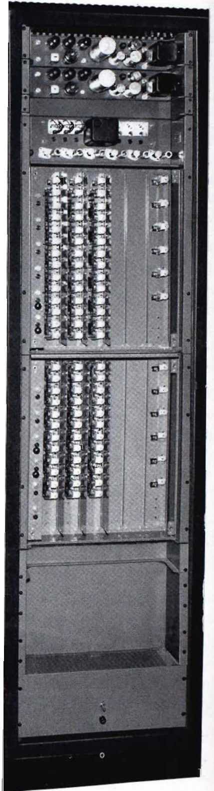
Standard rack containing relay chassis, amplifiers and power supplies.
