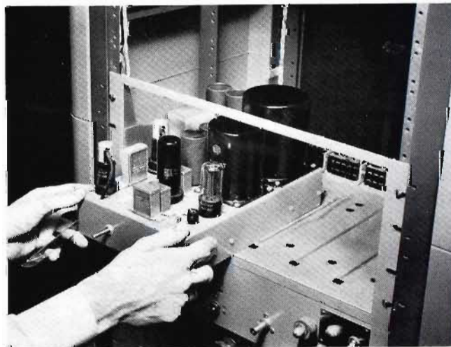
Plug-in amplifier permits quick and easy removal or interchange of units
