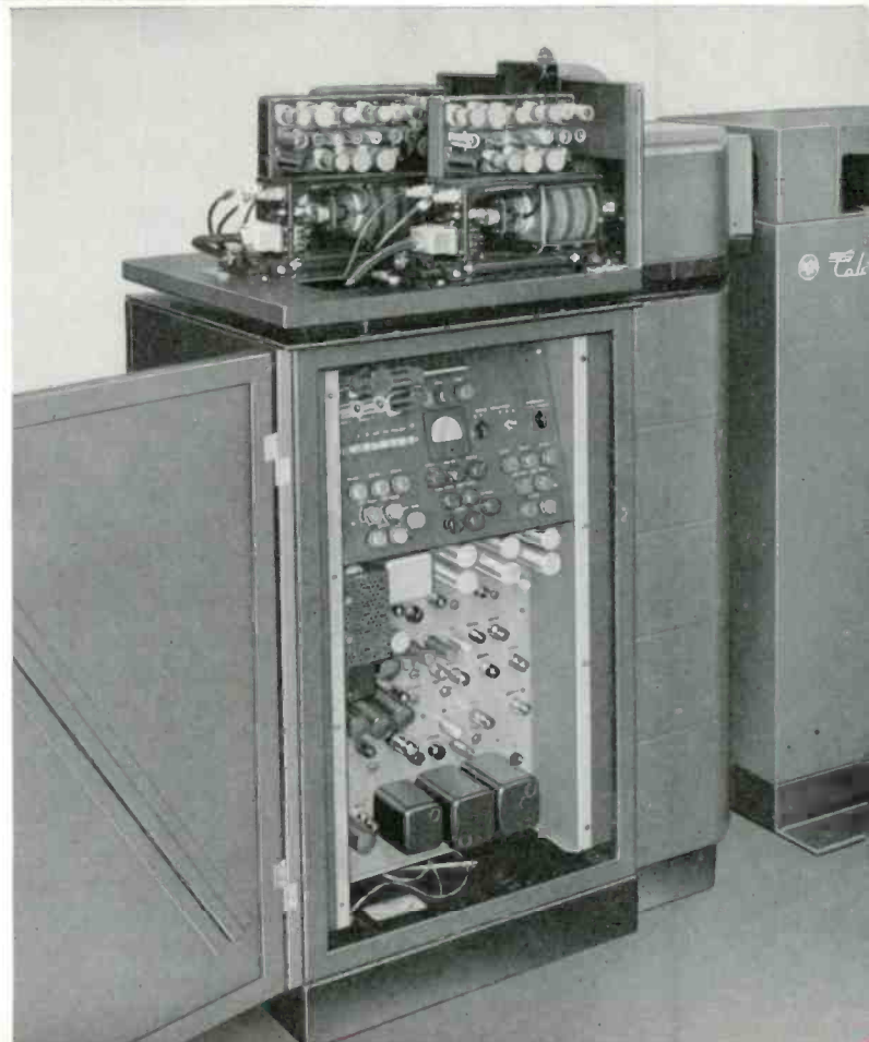
View of 3-Vidicon Camera pedestal showing location of major elements—camera sub-chassis atop pedestal and camera auxiliary including local control panel mounted in the rack-like base. The camera auxiliary may be mounted on either side of the camera pedestal. The local control panel essentially duplicates the setup controls of the camera control panel. This is of convenience to the operator in the initial setup of the camera chain, after which the control functions are switched to the console or rack mounted camera control panel position.
