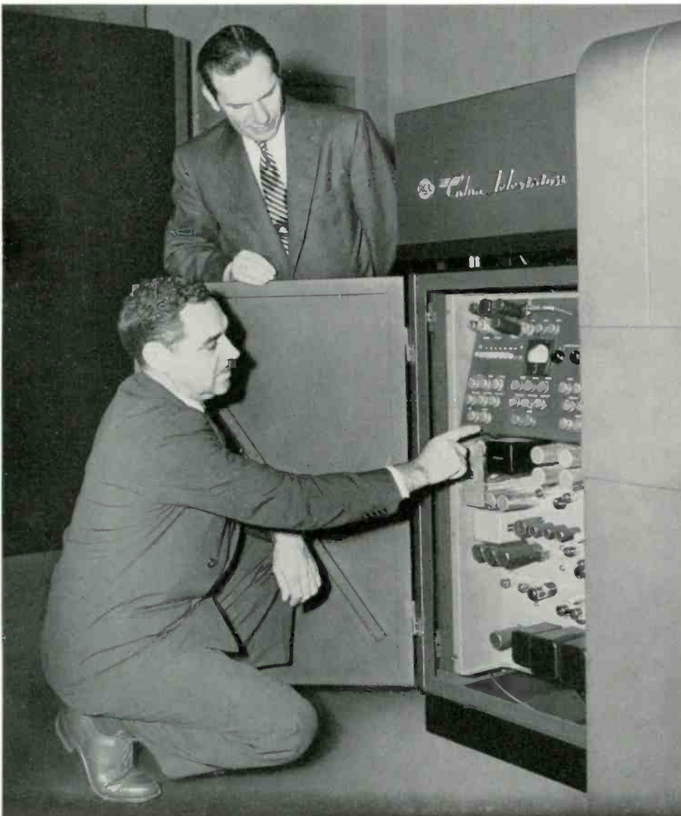
FIG. 18. A. R. Hopkins, Manager of RCA Broadcast Equipment Marketing and C. G. Nopper, Chief Engineer of WMAR-TV, Baltimore, are inspecting the control panel of the "3-V" Color Film Camera. This view of the 3-Vidicon Camera pedestal shows the location of vidicon enclosure atop pedestal, local control panel, and camera auxiliary panel.
