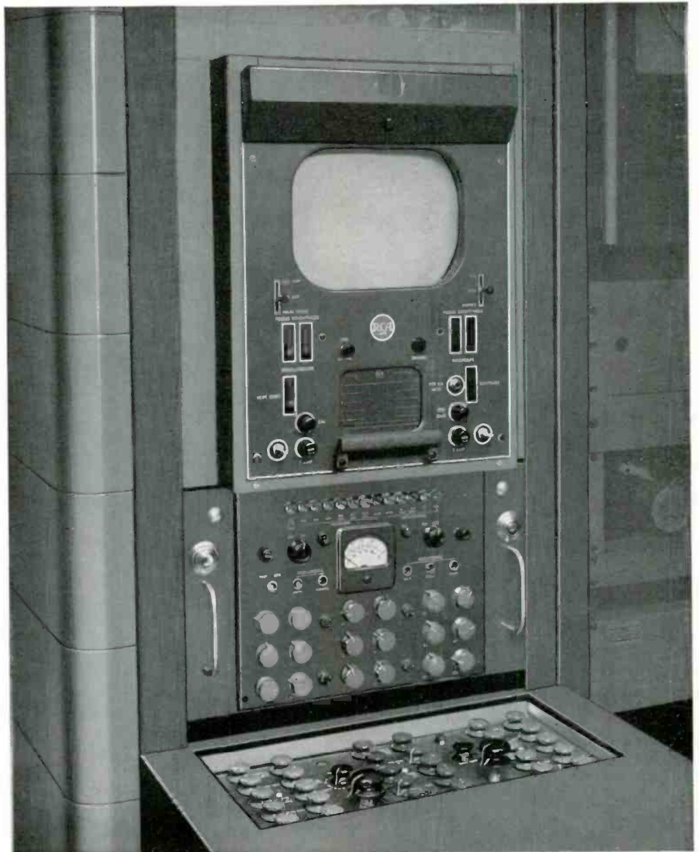
FIG. 28. Either the film or studio camera controls may be mounted in a standard rack shelf as shown here. When this is done the monochrome monitor is usually mounted directly above the camera control position and the color monitor in the adjacent rack at about the same eye-level. An arrangement of this kind saves floor space and is convenient for setup and maintenance. It is particularly useful in installations where the camera control position is in a room separate from the studio control room.
