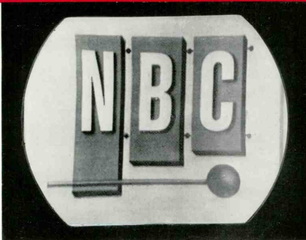
Station test pattern revealing how WA-8A Color Stripe Generator enables any TV station which is equipped to transmit network color to add a narrow color stripe to its regular black and white television signal. On color home receiver tube a thin vertical stripe of greenish yellow color appears at the right edge of the picture as shown here.
