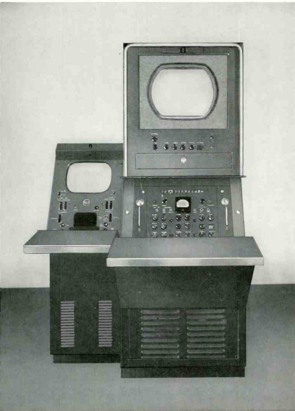
FIG. 16 (left). The complete 3-V Camera Control equipment includes a TM-6C Monochrome Monitor, a 19-inch Console containing the camera control panel and processing amplifier and a Type TM-10B Color Monitor. These three units may be grouped together as shown here. Or the color monitor may be suspended from the wall or ceiling for better visibility (by producer, technical director, etc.). The two console units can be located separate from the monochrome control units or mounted in line with them. When desired the control panels can be furnished for rack mounting as shown in Fig. 28, page 101.
