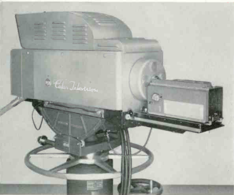
Telephoto or zoom-type lenses can be accompanied on the TK-41 rotatable lens turret when desired.
