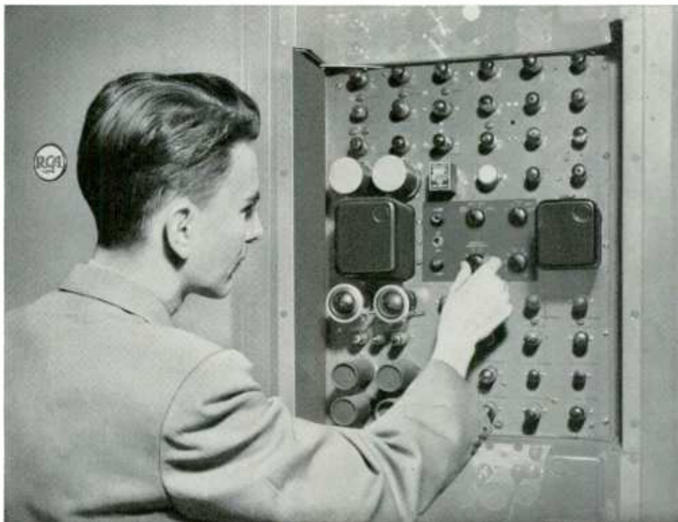
FIG. 9. View of the advanced design Sync Generator which has reduced the rack space to one-third that occupied by former designs. Providing extra stability, small size and combining all sync functions in a single chassis, it is ideal for color TV applications. It includes a built-in Genlock, dot generator, gating generator and regulated power supply.
