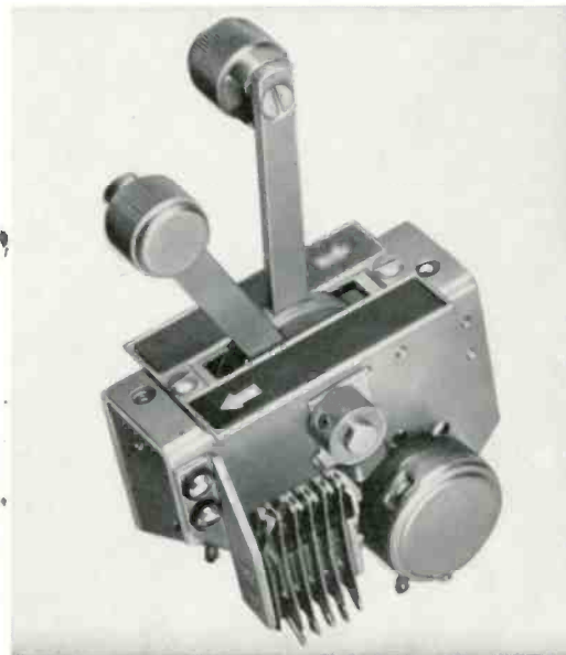
Close-up view of the fader mechanism located in the control panel of the TS-5A.
