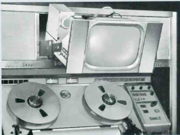
Slide and tilt mounted monitoring — accessibility plus.
