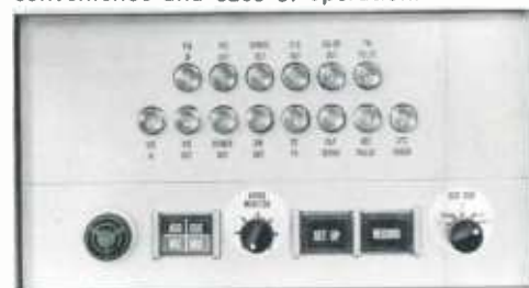
Record functions in TR-4 are grouped for convenience and ease of operation.
