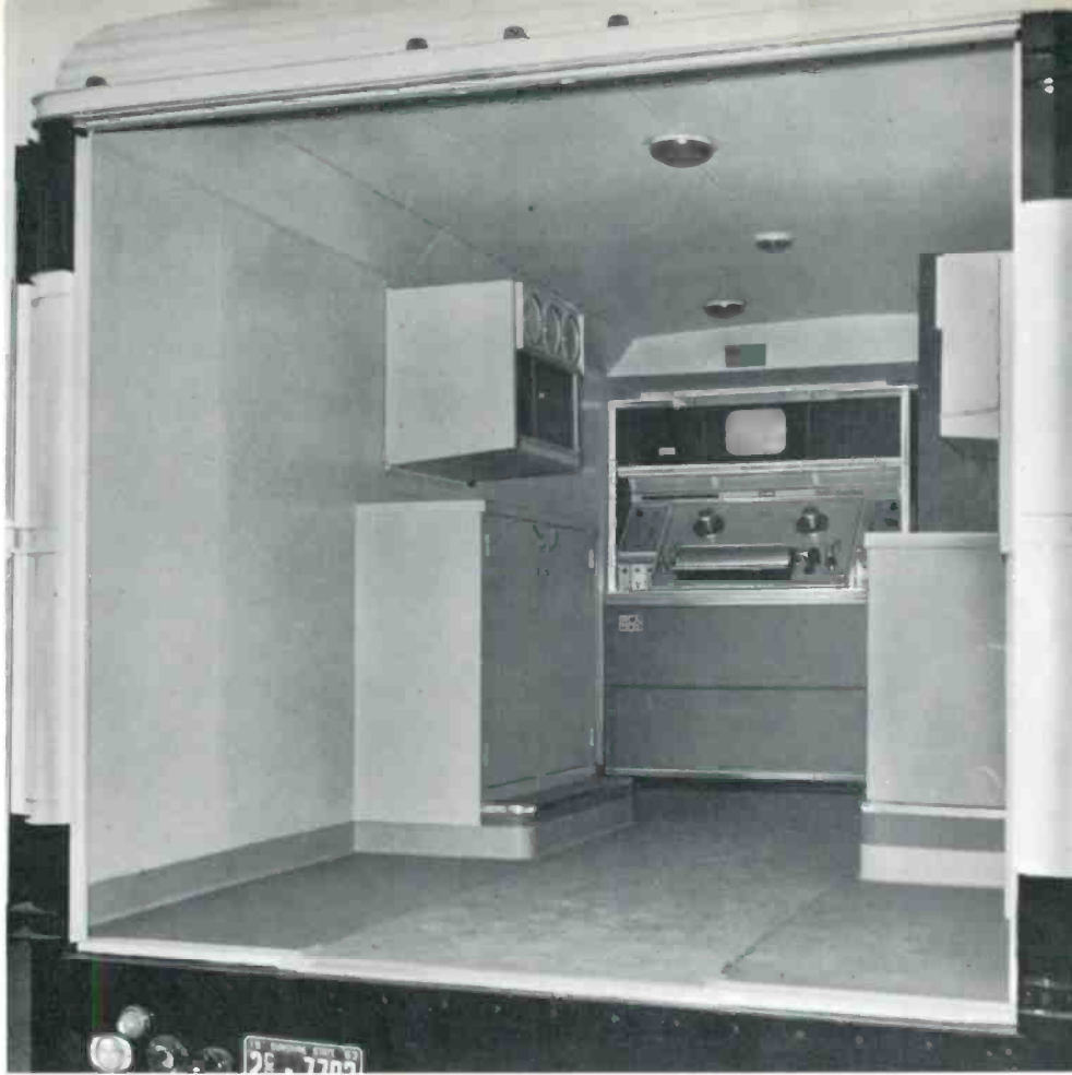
MOBILE TV TAPE RECORDING CENTER —Interior view of TJ-72 showing roomy interior with mounted TR-22 Tape Recorder together with audio facilities, cabinets, and compartments for tape storage, etc. More than 5½ feet of extra space at rear can accommodate field camera chain or other needed equipment for on-location tape recordings.
