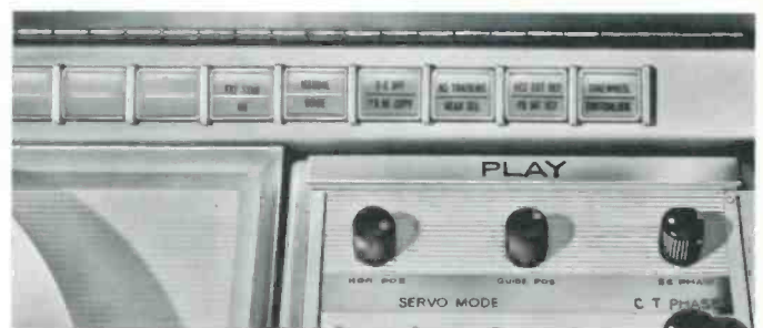
Non-standard mode indicator panel.
