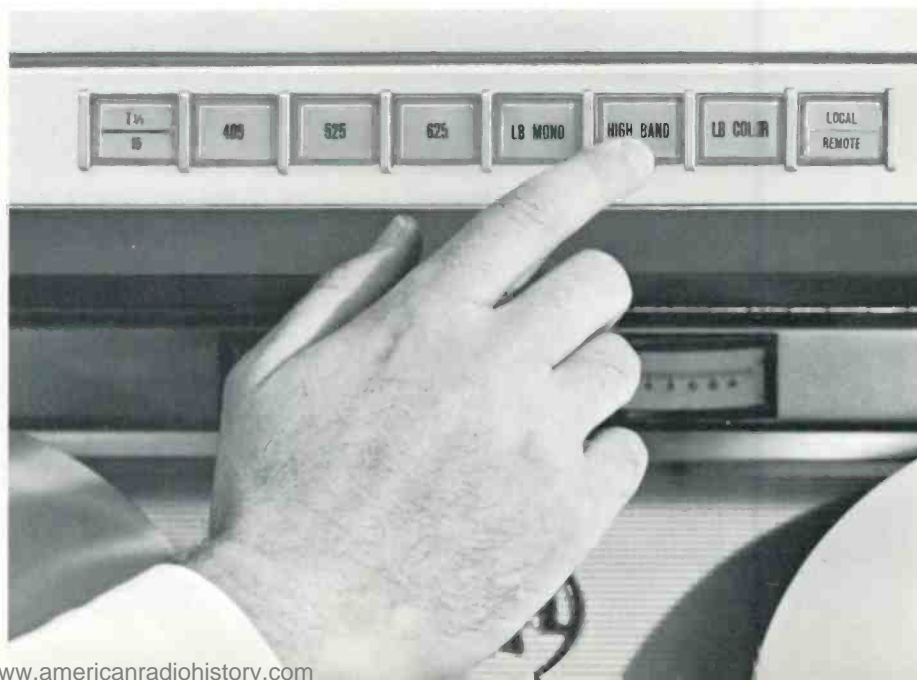
Switchable deviation standards for world wide use. International model provides choice of 405/525/625 (809 optional) line standards.
