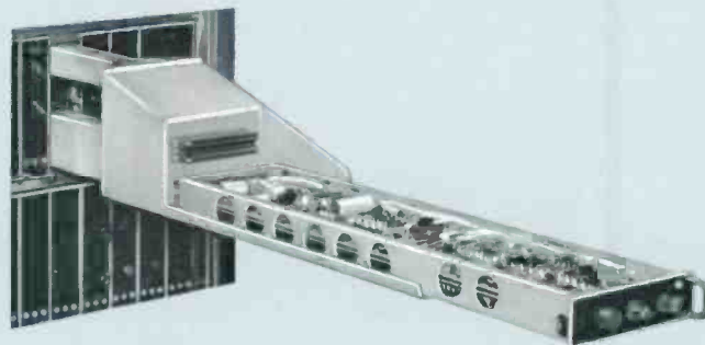
Similar module layout and construction — module extender for servicing — easy to maintain.
