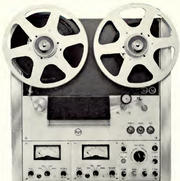
Type RT-21A Stereo Audio Tape Recorder, ES-41921-AS showing single module for manual at left, a second module for stereo, center, and control unit on right below tape transport chassis.
