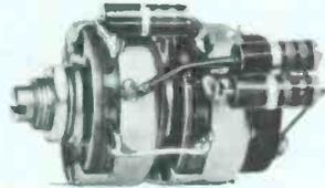
Dual-ganged composition potentiometers wired as volume controls for bridging 600- or 150-ohm balanced lines. The output matches a 600- or 150-ohm balanced line. MI-11278E includes a 1¾-inch knob while MI-11278F has a short, slotted shaft for screwdriver adjustment. Bushing fits ⅜-inch (10 mm) hole in panels up to ⅛-inch thick. Nuts included.
