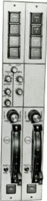
Includes a 30-step, tapered-to-infinity fader, provisions for a plug-in booster amplifier, an echo-select (pre- or post-) and -level control, four submaster-select pushbuttons, a cue on-off switch, channel on-off switch, and a foldback- select switch. Wired to accommodate a Type BE-100 Equalizer Module (see below). Two modules illustrated: one at left has equalizer installed; other is without equalizer.
