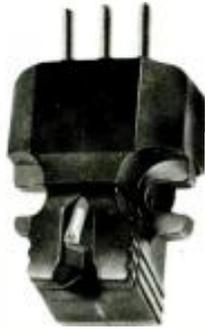
The Universal Pickup Cartridge and Replaceable Stylus provide a fully compatible unit for reproducing stereophonic and monophonic phonograph records. The cartridge utilizes a moving-magnet system for superior performance and simplified stylus replacement. It is completely housed in a molded plastic case. The stylus replaces without use of tools.
