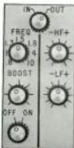
Designed as a plug-in for the Type BMM-100 Master-Mixer Module, the equalizer submodule is a zero-loss device which provides separate low-, high- and peaking-frequency (presence) equalization. Maximum equalization exceeds 19 dB boost or cut at 40 Hz; 15 dB boost or cut at 10 kHz and 16 dB boost at any frequency between 800 and 10,000 Hz (see curves). Added to the mixer module at anytime.
