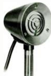
The Type SK-39 Aerodynamic Microphone has excellent response for close talking announce purposes. Its light weight and small size make it ideal for remote pickup and mobile use. It is used for paging and announcing in areas of high noise level because its rising high frequency characteristic gives excellent intelligibility.
