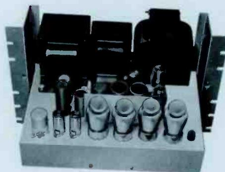
The 200-watt Power Amplifier is a bridging type amplifier using four Type 6550 beam tetrodes in a push-pull, Class AB<sub>1</sub> circuit. Its exceptional frequency response and low distortion make it ideal for wide-range reproduction of music. When more than one amplifier is used in a system the inputs are paralleled. With 16 decibels of inverse feedback for frequency stabilization, it produces 200 watts of clean audio power.
