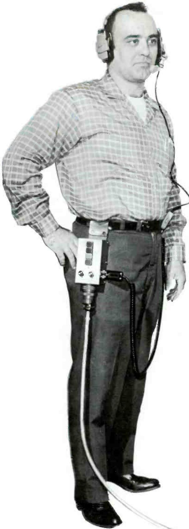
Unique "belt box" station for studio floormen. The box hangs on his trousers belt and connects him with the intercom system without restricting mobility. Four pushbuttons give him two-way communication with as many stations on the intercom system.
