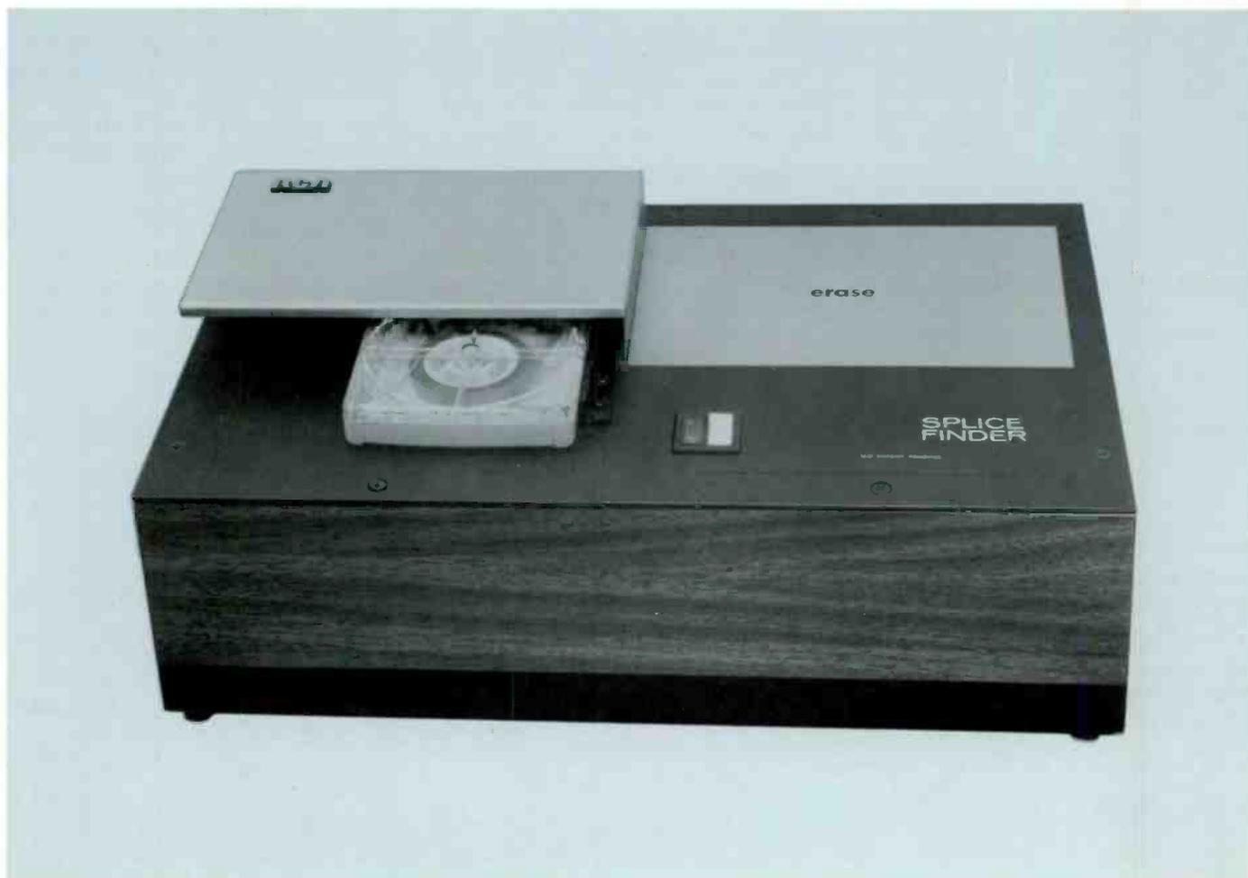
The Type SFE-1 and SFE-2 are devices most useful wherever NAB-type cartridges are recorded. It searches out and locates the tape splice at a point downstream of the capstan. With the splice so located, it is essentially impossible to record on the splice. This, in turn, eliminates the familiar program discontinuity a recorded splice almost always causes.
