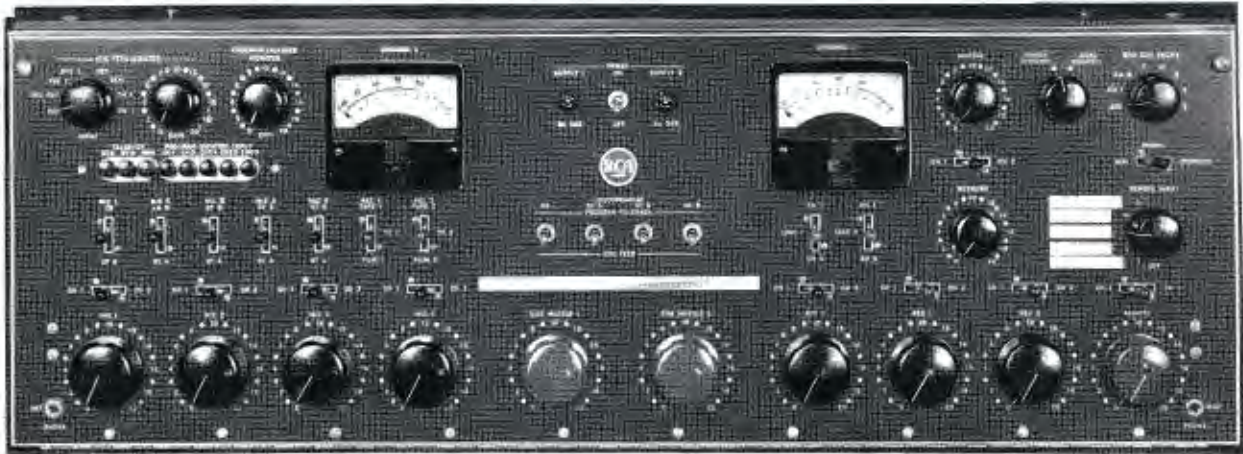
Etched front panel of the BC-6A Consolette showing entire operating facilities.
