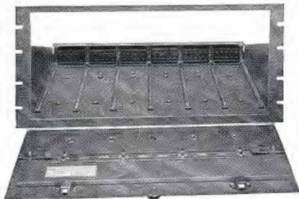
Panel removed showing guide bars and receptacles.
