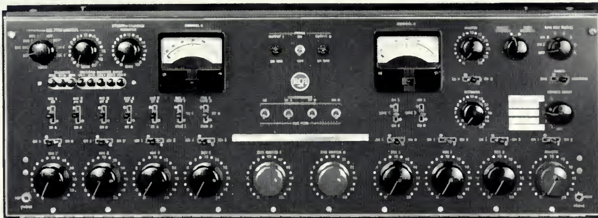
Etched front panel of the BC-6A Console showing entire operating facilities.
