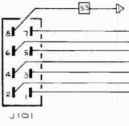
THESE CONNECTIONS INSTALLED IN BTE-10AT ONLY. LEAD FROM J107-18 TO TERMINAL TB102-46 ALSO DISCONNECTED AND TAPED IN BTE-10AT ONLY.
