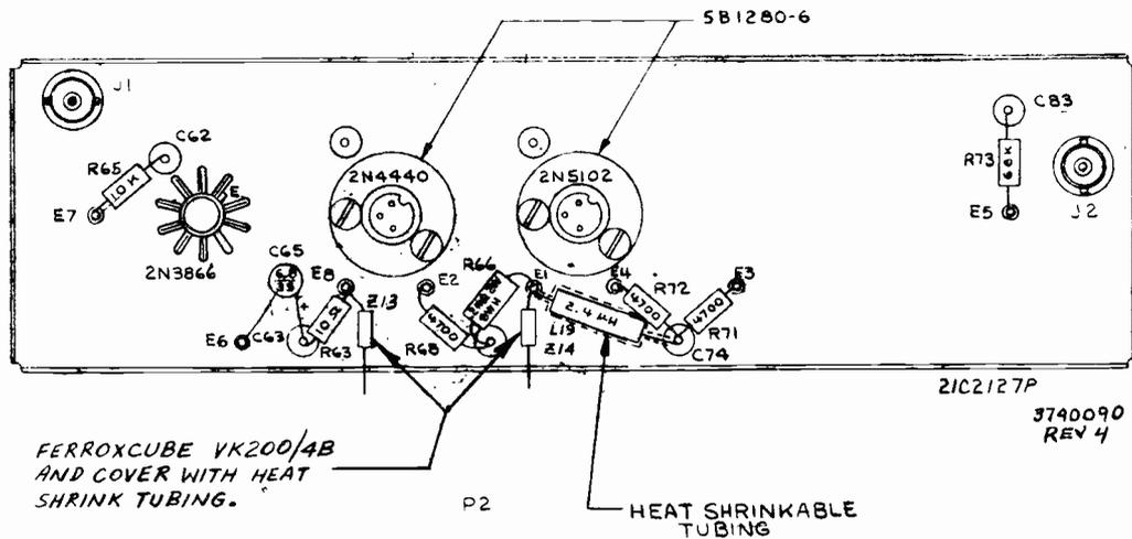
Figure 62. Exciter, RF Amplifier Assembly, Wiring Diagram
