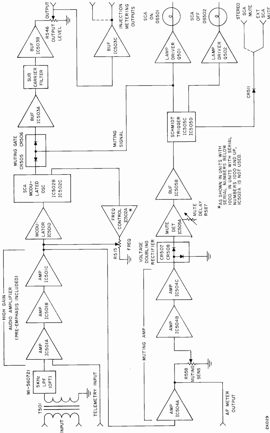
Figure 5. BTX-1B SCA Generator, Simplified Block Diagram
