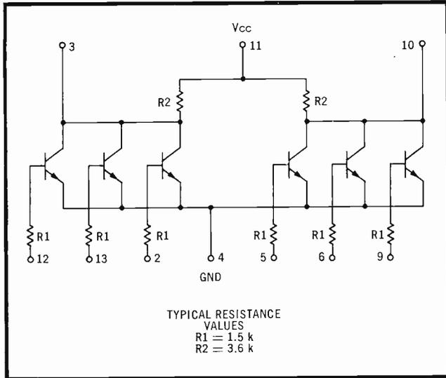
Two 3-input positive logic NOR gates in a single package. Each may be used independently, paralleled for increasing the number of inputs (subject to loading rules), or cross-connected to form bistable elements.
