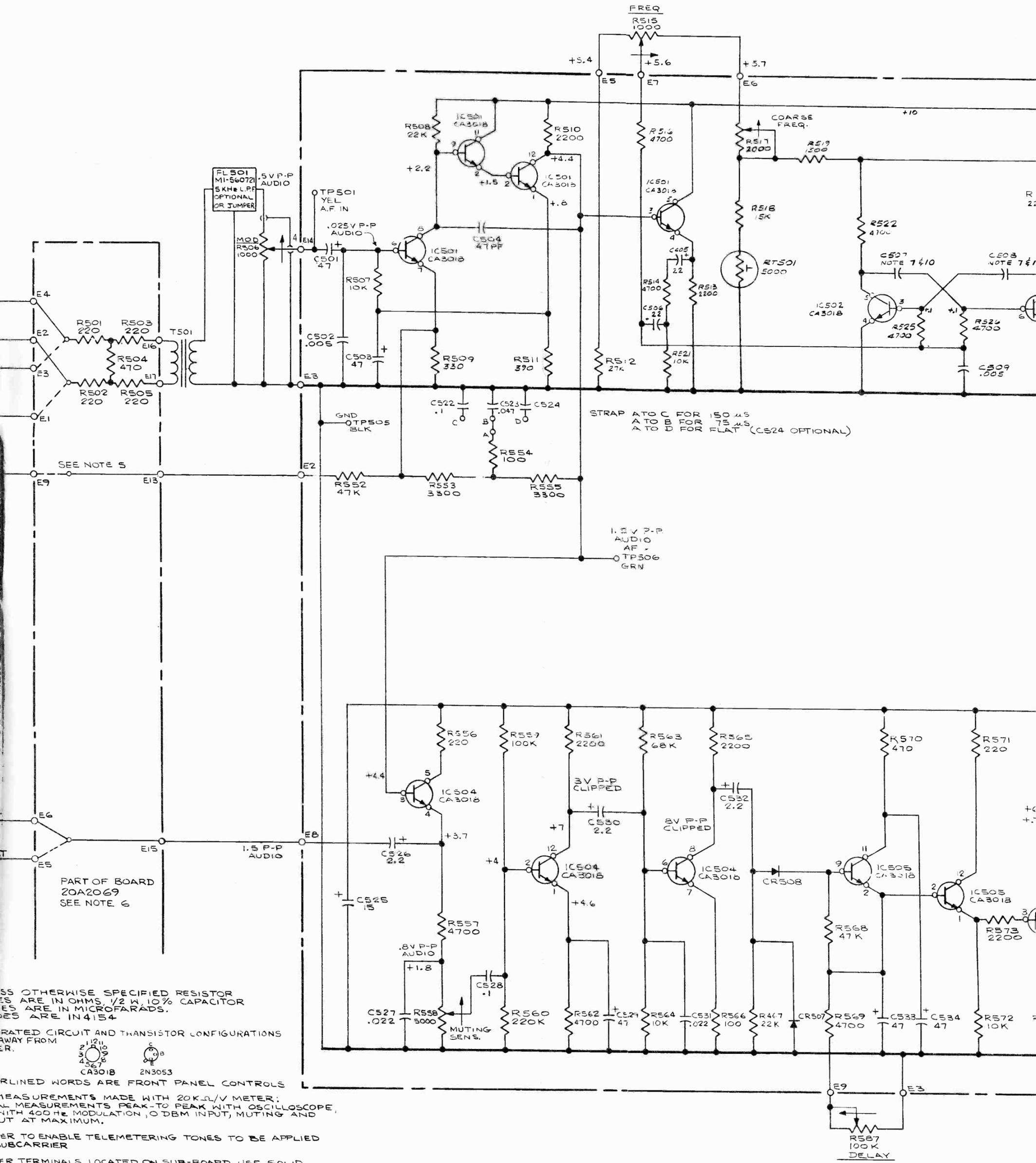
UNLESS OTHERWISE SPECIFIED RESISTOR VALUES ARE IN OHMS, 1/2 W, 10% CAPACITOR VALUES ARE IN MICROFARADS. RESISTOR VALUES ARE IN 4154
