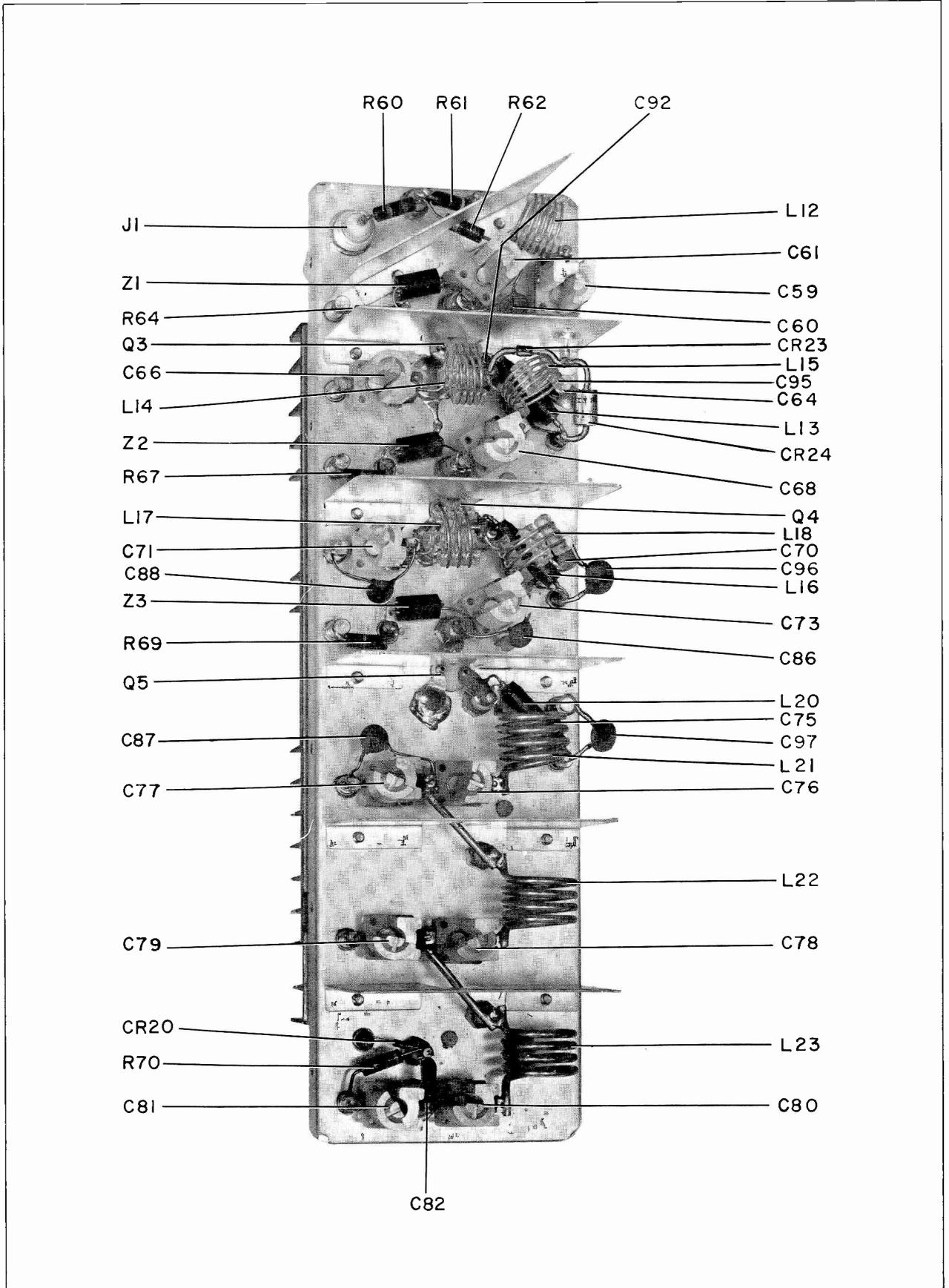
Figure 23. Exciter, RF Amplifier, Parts Location, Bottom
