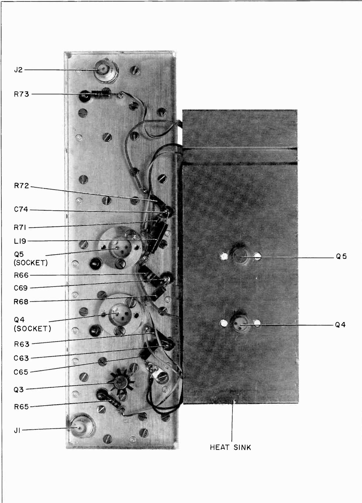
Figure 22. Exciter, RF Amplifier, Parts Location, Top
