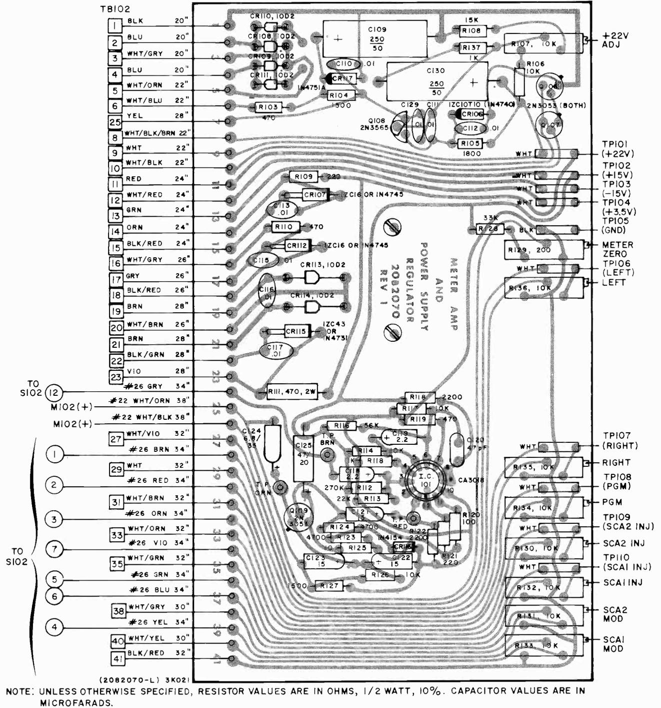
Figure 17. Main Frame Metering Amplifier Board, Parts Overlay, Bottom
