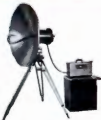
RCA Microwave Relay Transmitter TR-1A. Transmits the picture signals from field to studio (or from studio to transmitter). It includes a parabolic antenna with hook-shaped wave guide, built-in transmitter, and remote control unit. Matching receiver unit at the station picks up the microwave relay signal.
