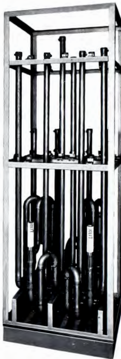
Triplexer with all covers removed to show system of tunable coaxial lines. Two output connections are made near the bottom, as shown. The two input lines are at the rear and are not visible.
