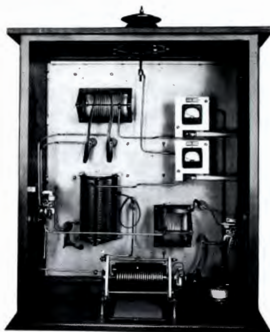
Interior view of a 5 KW line terminating unit mounted in a BPA-1A Housing
