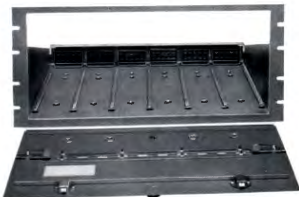
Panel removed showing guide bars and receptacles
