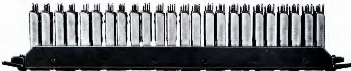
A Rear View of the 33-A Jack Panel
