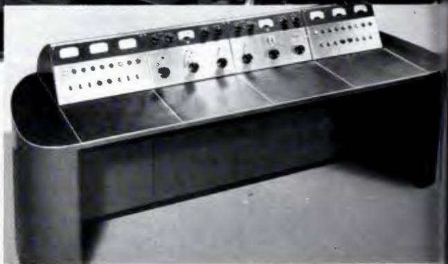
Typical console set-up for two transmitters, such as: two AM transmitters, two FM transmitters, or one AM and one FM transmitter. The turrets bolt to the desks. Desk sections bolt to each other. Knockouts for the wiring are provided in all desk and turret sections. All meters are recessed behind turret panels.
