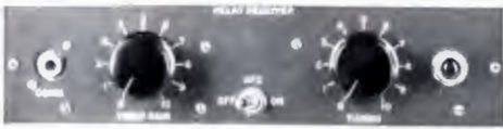
Relay Receiver Control, M1-26247. Controls video gain and receiver tuning. Includes 2 potentiometers, AFC "on-off" switch, tally light, and telephone jack.
