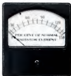
REMOTE ANTENNA AMMETER, MI-7184-A-150
