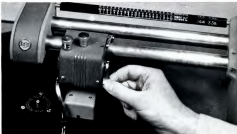
RAISING AND LOWERING the cutter head is easily done by this lever which permits raising the "to rest" position or a gentle lowering to the recording position.
