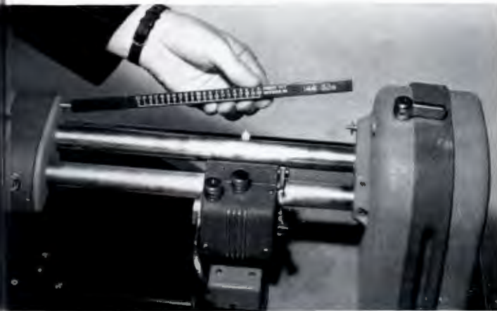
CALIBRATED TIME SCALES for 96, 104, 112, 120, 128, 136, 144 and 152 ("inside-out," "outside-in," at 33\frac{1}{3} or 78 rpm are provided. Here, proper scale to agree with "pitch" setting is inserted.
