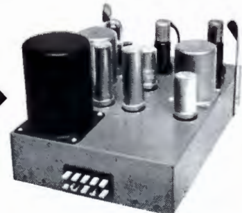
BA-2C Amplifier—Rear view. Plug-in chassis permits easy removal of amplifier for servicing
