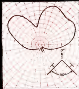
90° angle between dipoles 90° phasing between dipoles
