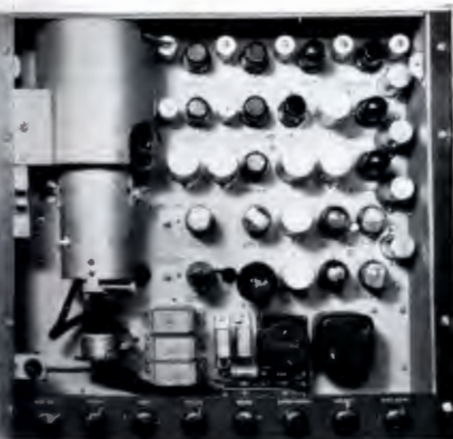
Monoscope Camera, TK-1A. Ideal as signal source of known quality for testing: station patterns, video amplifiers, picture tubes, TV receivers. Pattern covers scanning symmetry, vertical and horizontal resolution, contrast, and brightness.
