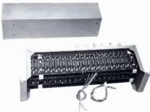
View of Sync Generator Delay Panel shown with protective cover removed
