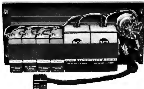
Rear view of Battery Cover showing batteries mounted in place
