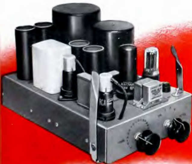
Program Amplifier (Type BA-13A) —The most versatile high-fidelity amplifier ever designed for broadcasting. Ideal as a program or line amplifier, bridge-line amplifier, isolator amplifier, cueing or monitoring amplifier. Improved design for greater accessibility; "plug-in" electrolytics for ease in servicing. Output: 2 watts (approx.). Higher gain: 65 db for matching input; 28 db for bridging input. Lower noise level: -82 db (with max. gain). Lower distortion: less than 0.5 to 1% rms, depending on output level. Frequency response: ±1 db, 30 to 15,000 cps.
