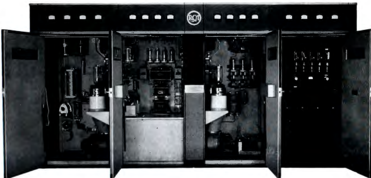
Front view with doors open showing interior construction. BTA-10F Transmitter with left and right wing extension cabinets.
