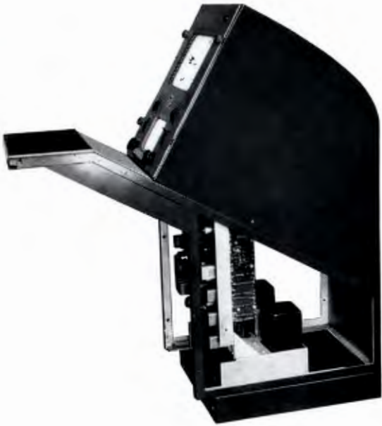
Camera Control Unit showing interior arrangement. This unit is normally housed in the master control console.
