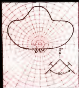
90° angle between dipoles 0° phasing between dipoles
