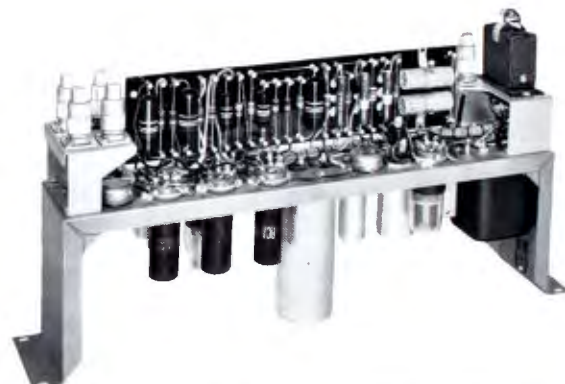
Small components, video and power connection are at rear of chassis
