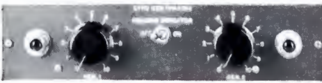
Sync Generator Phasing Control, M1-26249. Provides for phasing one of two local synchronizing generators with one remote synchronizing generator.
