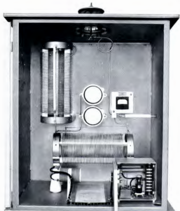
Interior view of BPA-10 with MI-7488A Monitor Rectifier
