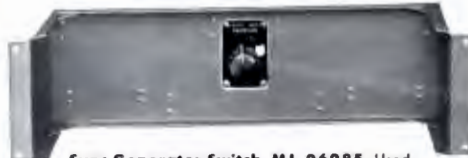
Sync Generator Switch, M1-26285. Used to switch outputs of either of two sync generators over to studio equipment. One selector for all 5 signals (horizontal, vertical, blanking, sync, and CRO sync).
