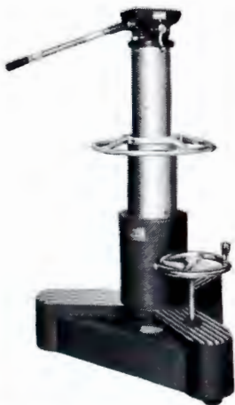
STUDIO CAMERA PEDESTAL, TD-1A —Television's favorite pedestal for studio and other indoor operations. Moves freely, quietly. Crank handle raises and lowers camera to any height between 40 inches and five feet above the floor. Moves in any direction—or about a point. Panning and tilting provided by Friction Head MI-26205.
