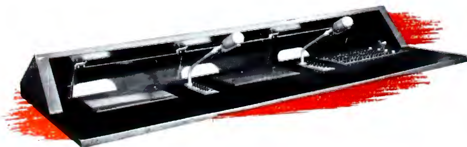
RCA Studio Consolelette Type 76-C4. This flexible and easy-to-operate control unit performs all the audio amplifying, monitoring, and control functions of a TV station—large or small. Can be used for single- or two-studio operation, and for two transcription turntables.
