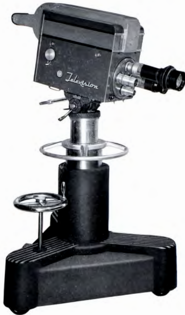
Studio Camera mounted on TD-1A Pedestal Dolly
