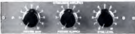
Stabilizing Amplifier Control, M1-26250. Includes three potentiometers. Controls: (1) picture gain; (2) picture clipper; (3) sync level in stabilizing amplifier.
