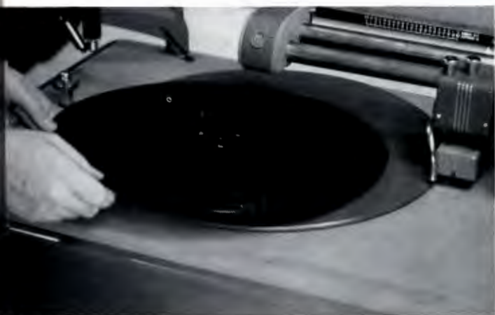
ANY TYPE BLANK may be used with the single driving pin provided. Here, recording blank is placed in position.
