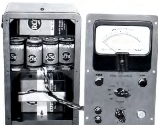
Removable panel provides easy access to batteries
