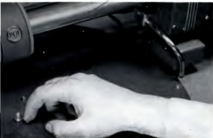
RECORD-DRIVE PIN comes up into position when this trigger-release button is pressed. Pin sinks into platter for records without driving holes.
