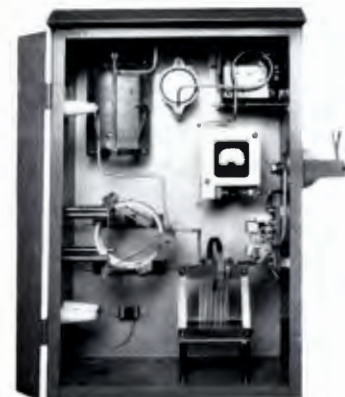
Interior view of 1 KW line terminating unit with phase sampling coil, antenna base metering and pattern switching facilities mounted in BPA-1A Housing
