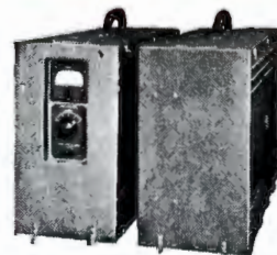
RCA Field Synchronizing Generator TG-10A. Produces timing pulses for TV field equipment. Unit No. 1 includes pulse-forming circuits, frequency-control circuits, and power supply. Unit No. 2 includes the pulse-shaping and output circuits.
