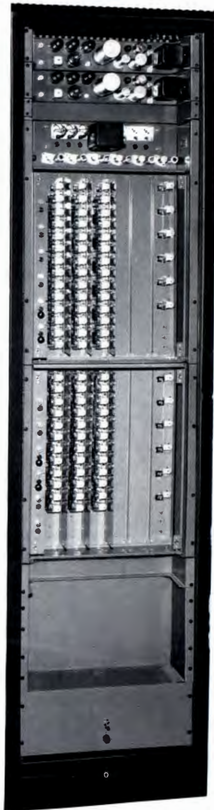
Standard rack containing relay chassis, amplifiers and power supplies.
