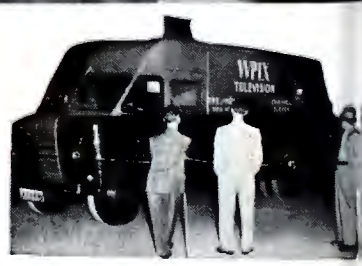
Television Studio-on-Wheels. This special RCA TV field truck is handling the track sound-and-picture pick-up between Roosevelt Raceway grandstand and WPIX in New York City. All RCA-equipped, it is designed to carry everything needed to operate up to 3 cameras in the field.
