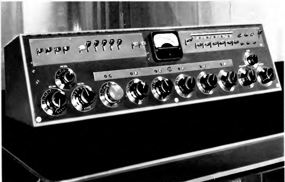
The studio console design shown below employs varied colored knobs and switch handles for easy and quick identification of certain controls. All escutcheons and dial plates are of nickel silver for attractiveness and long wear.
