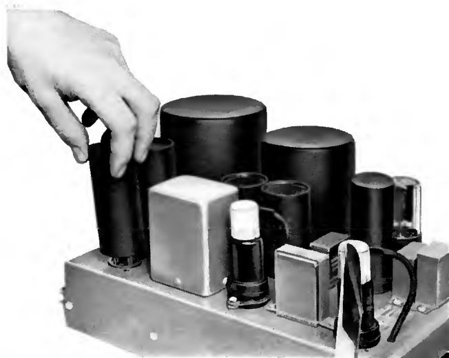
"Plug-in" type electrolytics provide long-life operation and maximum accessibility
