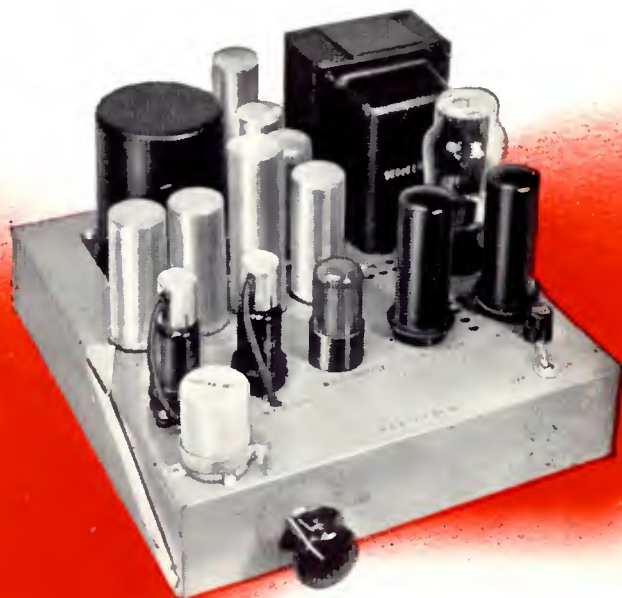
Monitoring Amplifier (Type BA-14A) —Designed for operation at microphone levels. High output of 12 watts is sufficient to drive several speakers or, in some applications, a recording head. Other uses include application as line amplifier for portable and mobile transmitters. High gain: 105 db. Low noise level: -20 db (with maximum gain); -40 db (with minimum gain). Low distortion: less than 3% at 12 watts. Frequency response: ±2 db, 30 to 15,000 cycles.
