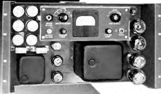
Regulated Power Supply, TY-25A. Provides well-regulated d-c source at loads from 200 to 300 ma. Output is adjustable between 260 and 290 volts. Less than 0.5% variation between minimum and maximum load.
