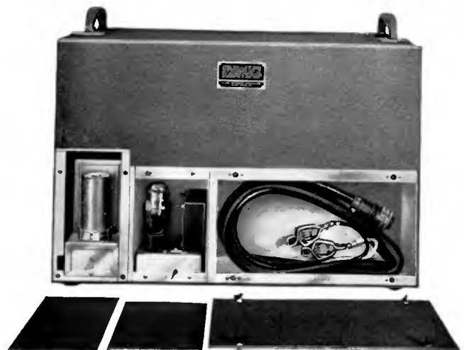
Rear view of WX-1A with cover plates removed. Compartments left to right are: Removable Vibrator Power Supply, Voltage Regulator and Filter, and cable and storage compartment.
