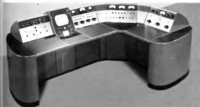
Typical console set-up for on RCA 5-kw television transmitter, and one AM or FM transmitter. From left to right: (1) TV transmitter control; (2) picture monitor; (3) TV audio monitor; (4) blank turret; (5) AM or FM transmitter control; (6) blank turret; and (7) AM or FM transmitter control.
