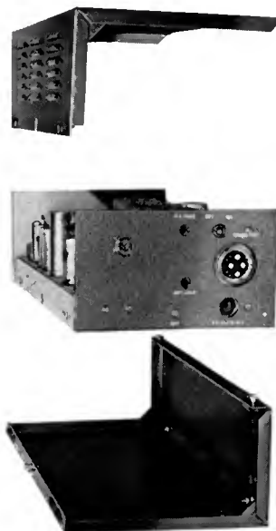
Accordion view showing construction of chassis and covers. Unique construction permits mounting on either right or left side.
