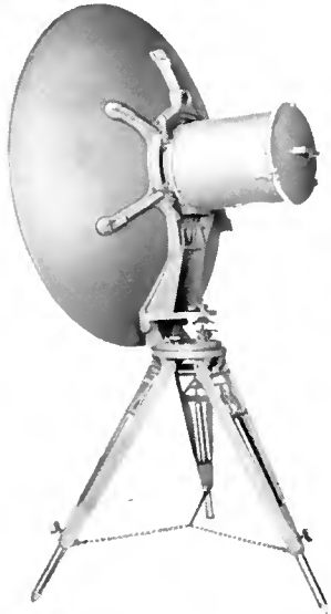
Reflector and Parapet Mount as used with TD-21A Tripod to support Relay Transmitter
