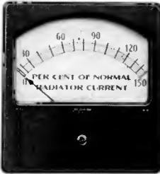
REMOTE ANTENNA AMMETER, MI-7184-A-150
