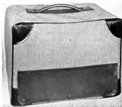
OP-7 with front panel cover removed. Covers of OP-7 and OP-6 provide space for carrying interconnecting cables.
