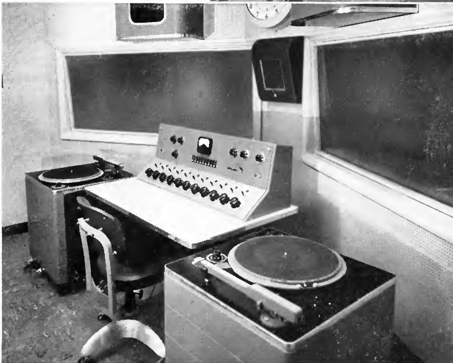
WJPG-FM, Green Bay. One of the specially-built studio-control consoles in WJPG-FM's 4-studio arrangement. Complete two-channel operation (AM and FM), simultaneous audition and broadcast from any combination of studios, remote lines, cueing and talkback are provided.
