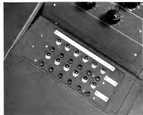
MI-26222 Master Control Panel shown mounted in sloping desk portion of TV console section.
