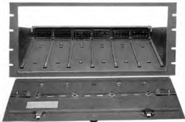
Panel removed showing guide bars and receptacles
