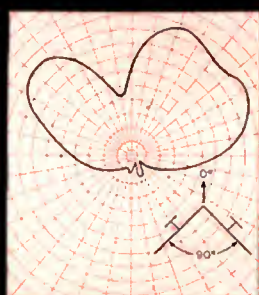
90° angle between dipoles 90° phasing between dipoles
