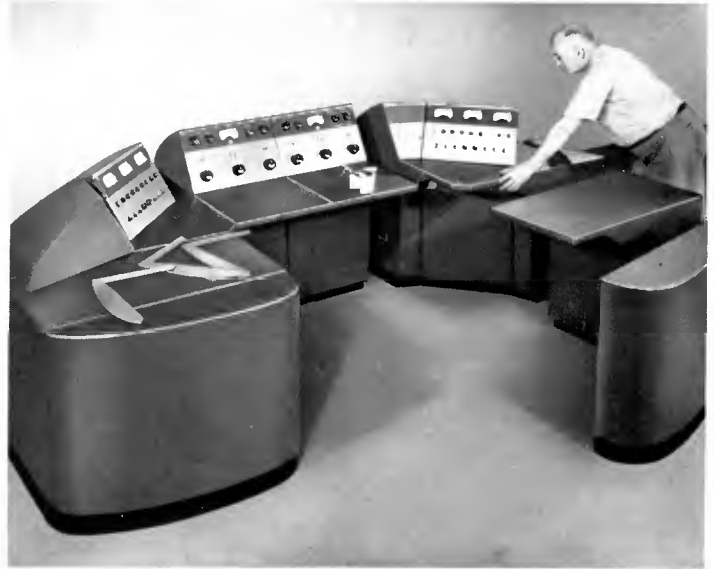
90° desk sections and 45° turret wings being used to "block-built" a "U" shaped arrangement to accommodate two transmitters (AM and/or FM). Sections simply bolt together.
