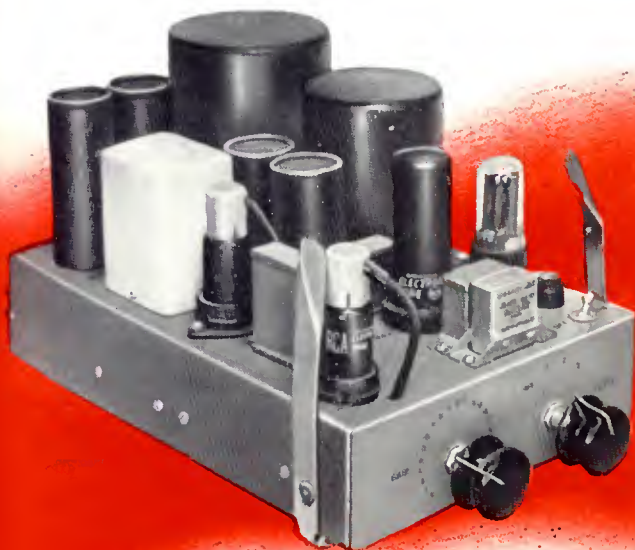
New Program Amplifier (Type BA-13A) —The most versatile high-fidelity amplifier ever designed for broadcasting. Ideal as a program or line amplifier, bridging amplifier, isolator amplifier, cueing or monitoring amplifier. Improved layout for greater accessibility; "plug-in" electrolytics for ease in servicing. Output: 2 watts (approx.). Higher gain: 65 db for matching input; 28 db for bridging input. Lower noise level: -82 db (with max. gain). Lower distortion: less than 0.5 to 1% rms, depending on output level. Frequency response: ±1 db, 30 to 15,000 cps.
