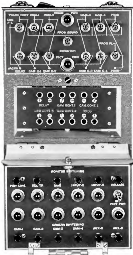
Front view of Switching Unit showing panel detail
