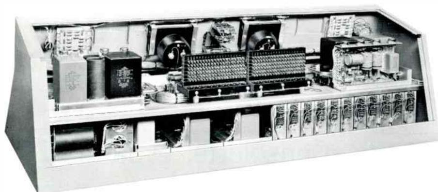
Rear of BC-7A with cover removed showing plug-in monitoring amplifiers and accessibility to external plug-in connection terminals.
