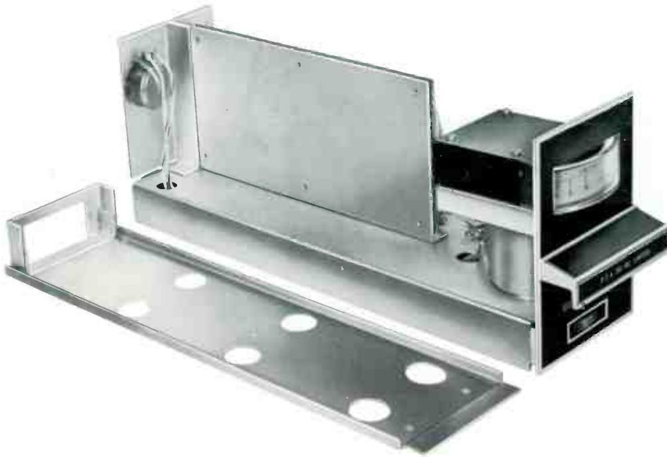
The BA-46 Limiter Amplifier, MI-11456 shown with the guide assembly ready for mounting in the BR-22 Mounting Shelf. The amplifier prevents over-modulation of the system on heavy passages of music or speech.
