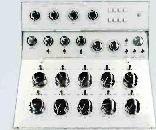
Custom-built ten-input mixer for Station WCAU designed for three-channel output. An accessory panel has been included to provide special utility and switching controls. This panel has been built into a special housing which is mounted on top of basic console form.
