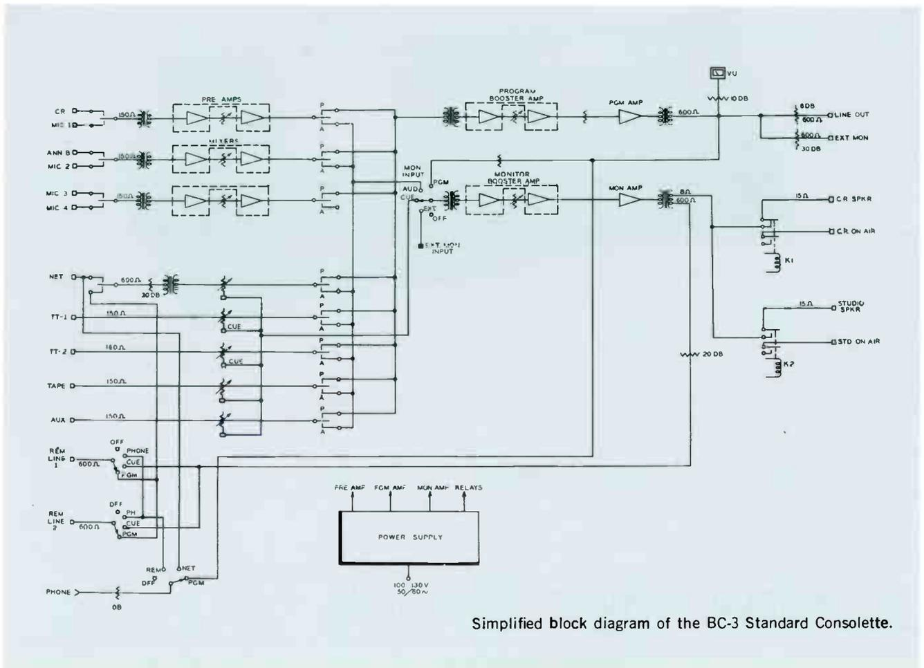
Simplified block diagram of the BC-3 Standard Console.
