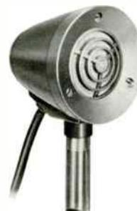
The Type SK-39 Aerodynamic Microphone has excellent response for close talking announce purposes. Its light weight and small size make it ideal for remote pickup and mobile use. It is used for paging and announcing in areas of high noise level because its rising high frequency characteristic gives excellent intelligibility.
