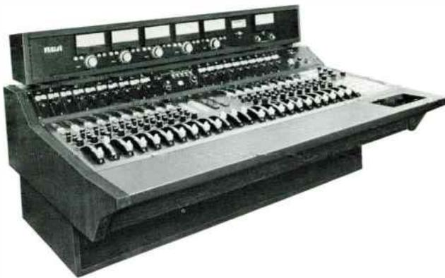
Built especially for Lewron Television in New York City, this is one of two custom audio consoles recently installed. The console offers 20 inputs, which accept either high- or low-level signals, fed to any or all of four output channels. A fifth output channel is equipped with built-in AGC. Each output channel feeds a one-by-two splitter. Also included is a slating switch and a built-in tone oscillator.
