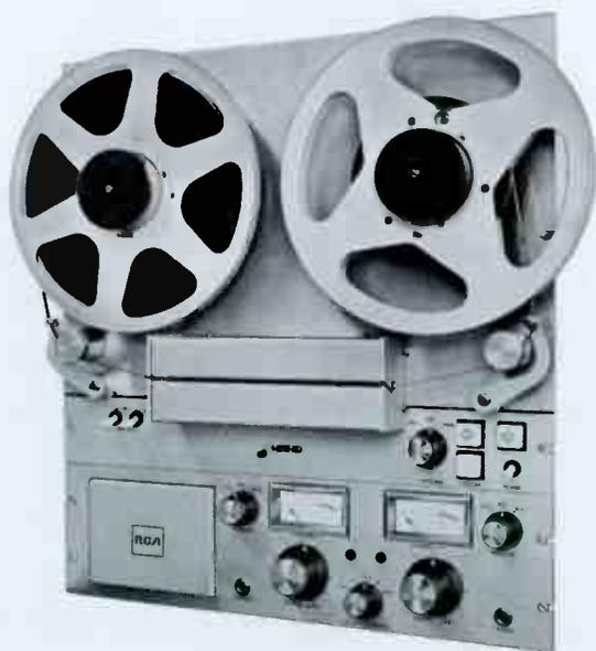
The Type RT-19 Program Logger tape recorder is designed for continuous long-duration recording. It records and plays in both directions to equal performance specifications. The logger is especially useful in broadcasting where it can serve as a complete and accurate program log and monitor to assure compliance with FCC regulations.
