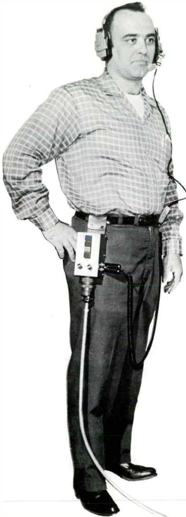
Unique "belt box" station for studio floormen. The box hangs on his trousers belt and connects him with the intercom system without restricting mobility. Four pushbuttons give him two-way communication with as many stations on the intercom system.
