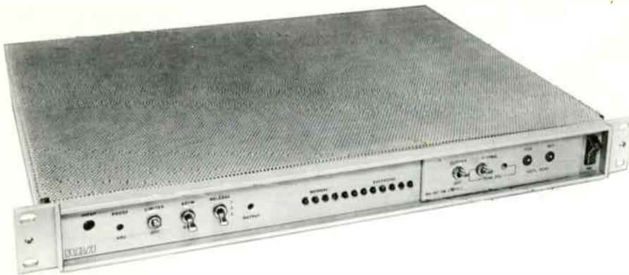
Either unit occupies only 1¾ inches (44 mm) of rack space. Depth of 14½ inches (360 mm) allows mounting in 18-inch (457 mm) depth rack or rack cabinet.
