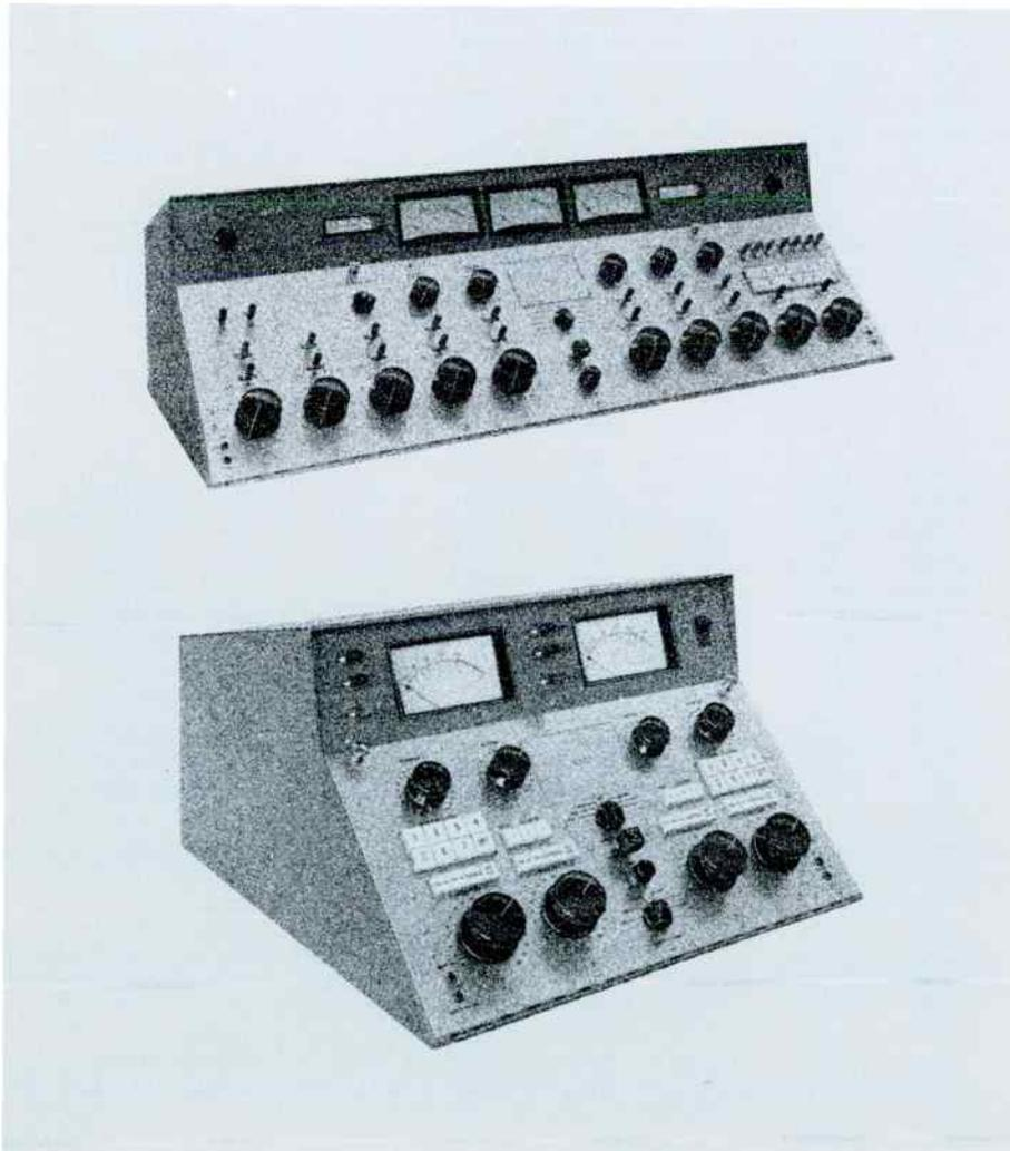
RCA Audio Consoles are high-quality systems designed to stand up under day-in, day-out use and abuse. There are mono, stereo, two- and three-channel consoles plus an auxiliary console for system expansion. Modular construction permits a variety of input combinations, depending on the modules selected. For your convenience, a selection of input arrangements is included for each console.
