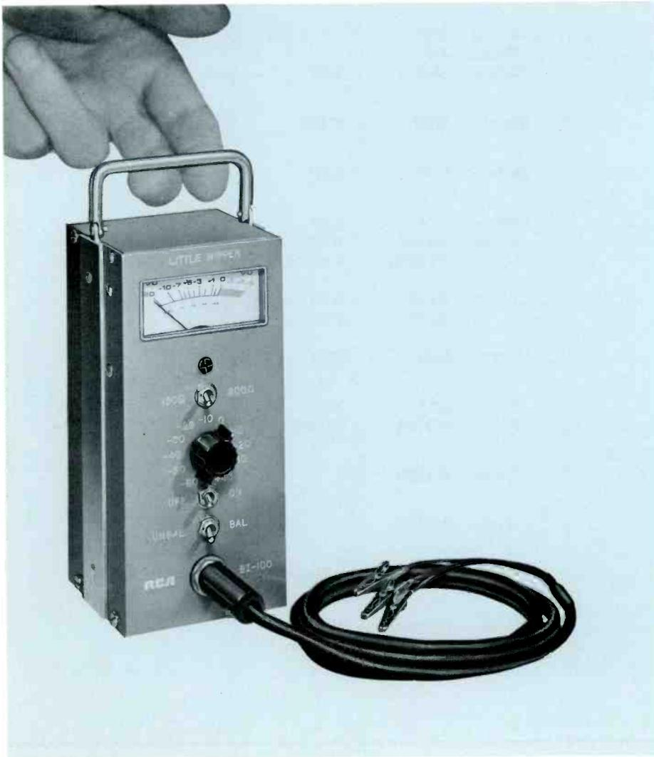
The extremely compact and light weight "Little Nipper" Audio Level meter is designed for use as a utility level meter in checking audio distribution systems, remote lines and other similar applications.
