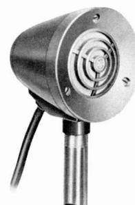
The Type SK-39 Aerodynamic Microphone has excellent response for close talking announce purposes. Its light weight and small size make it ideal for remote pickup and mobile use. It is used for paging and announcing in areas of high noise level because its rising high frequency characteristic gives excellent intelligibility. Another application is for use by an individual soloist, where a second microphone is used to pick up the musical accompaniment.
