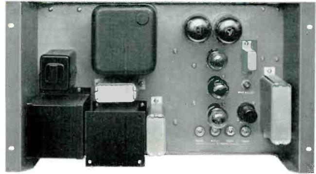
Regulated bias supply for the visual power amplifier is a chassis mounted unit located in extreme right hand cabinet of TT-25DH.
