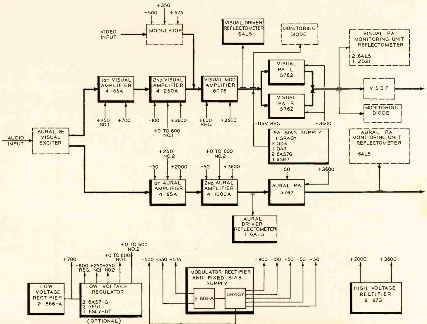
vides an adjustable line voltage to the filament primaries, exciter, modulator, low voltage rectifiers and bias supply. Automatic filament line voltage regulators and automatic regulators capable of handling the complete transmitter are available as optional items.
