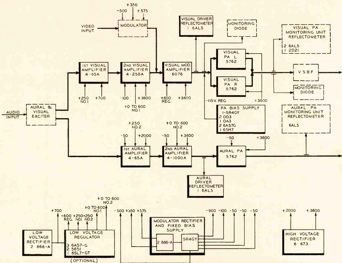
vides an adjustable line voltage to the filament primaries, exciter, modulator, low voltage rectifiers and bias supply. Automatic filament line voltage regulators and automatic regulators capable of handling the complete transmitter are available as optional items.
