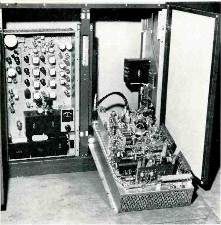
Transmitter exciter unit (left), and modulator unit (right) are mounted on hinged chassis which tilt forward for ease of servicing.
