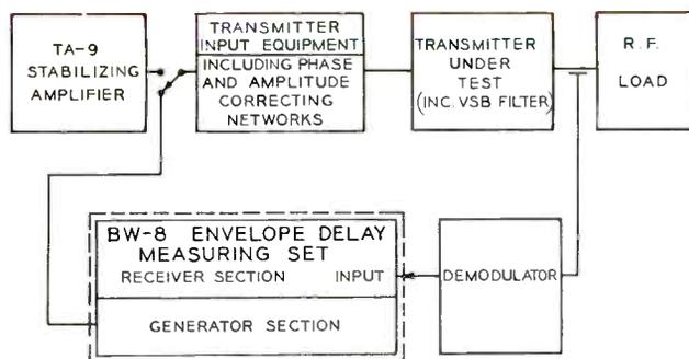
Test set-up to measure envelope delay
