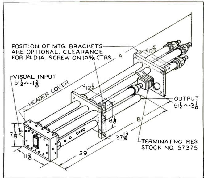
Vestigial sideband filter, MI-19114-B, designed for the TT-2BH Transmitter.
