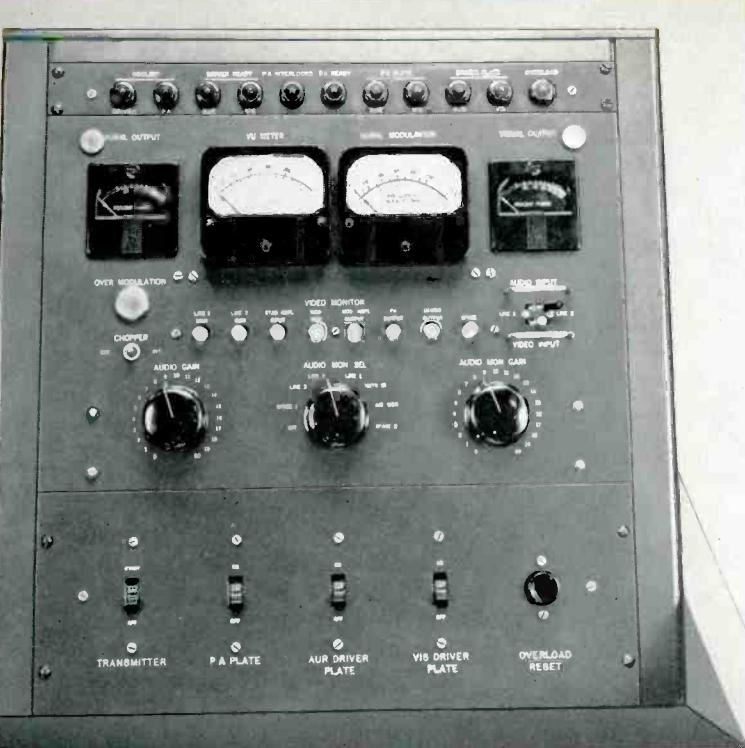
Closeup view of indicator, monitor control and transmitter control panels mounted in 22 inch console housing.
