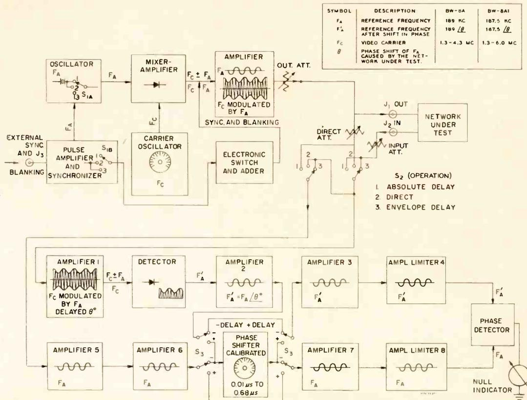
signal fed to the transmitter. Position 2 measures the amplitude of the signal at the input of the receiver. Position 3 is for balancing the VTVM and positions 4 and 5 are for use as a null indicator for the phase detector. Position 4 is of lower sensitivity for initial balancing of the phase detector. By means of another switch, the phase shifter network can be introduced into either one of the two receiver chains, allowing compensation of positive or negative phase delay.
