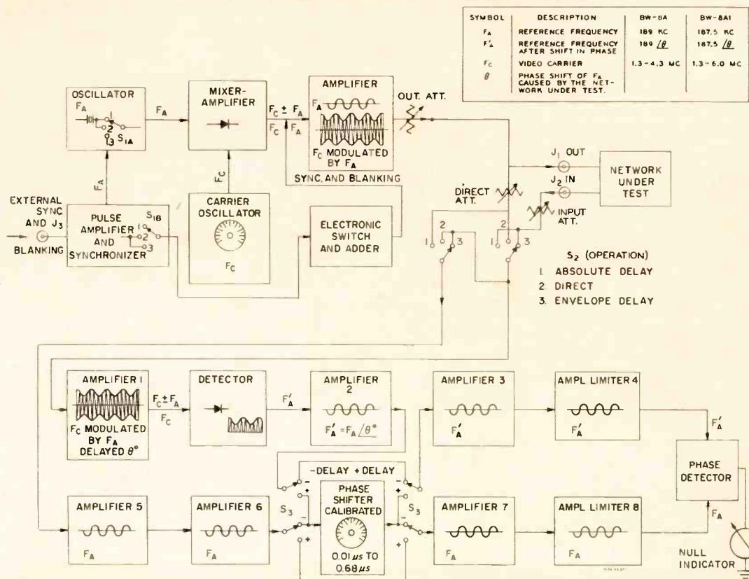
signal fed to the transmitter. Position 2 measures the amplitude of the signal at the input of the receiver. Position 3 is for balancing the VTVM and positions 4 and 5 are for use as a null indicator for the phase detector. Position 4 is of lower sensitivity for initial balancing of the phase detector. By means of another switch, the phase shifter network can be introduced into either one of the two receiver chains, allowing compensation of positive or negative phase delay.
