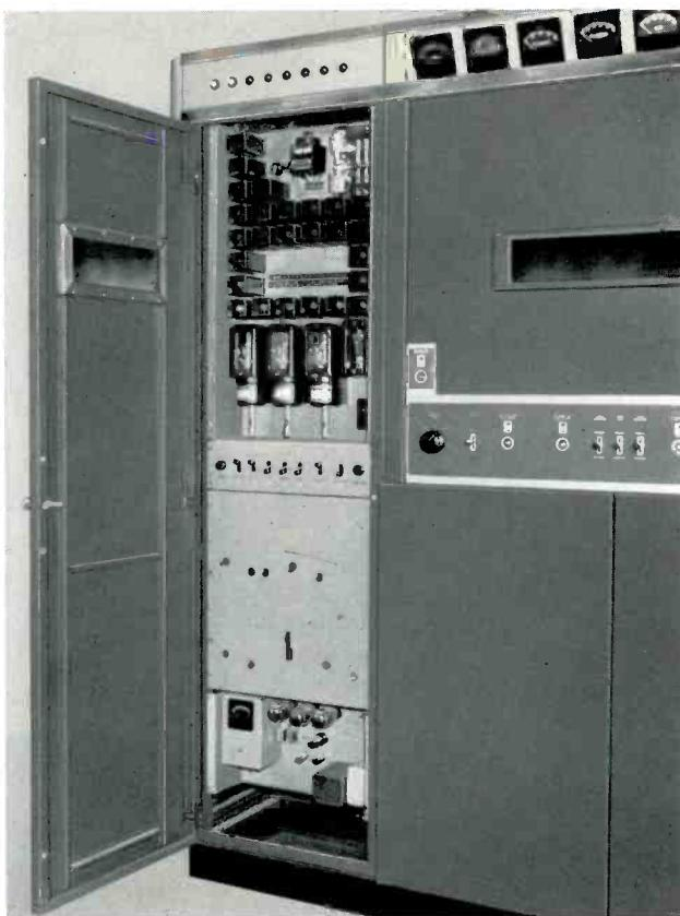
Control circuits of the TT-6AL are grouped in separate cabinet with status lights on a panel above the door. Auxiliary switches, breakers, overload and auxiliary relays, and overload indicating lights are located behind door.
