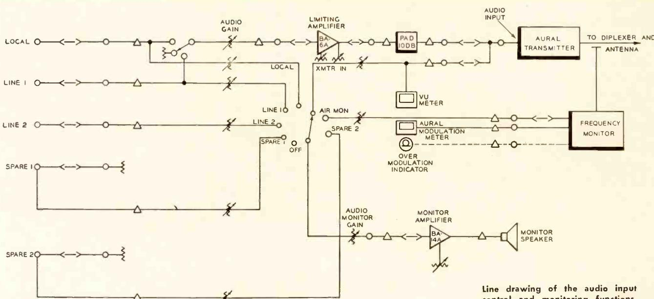
Line drawing of the audio input control and monitoring functions.
