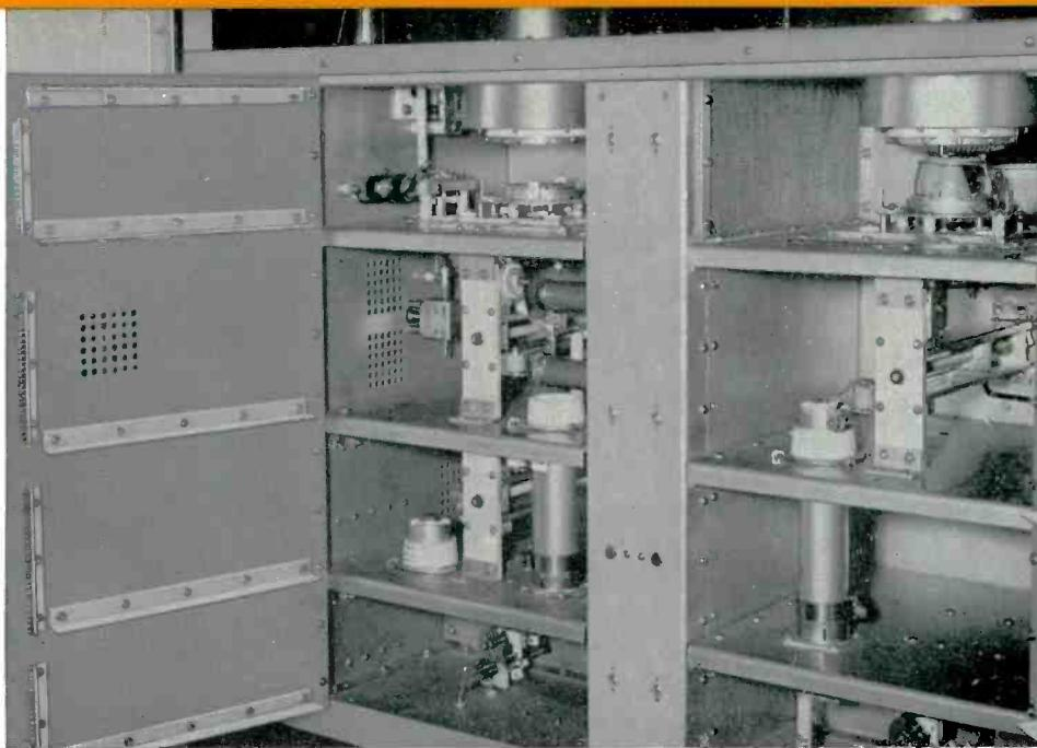
Transmitter exciter (left) and modulator unit (right) are mounted on hinged chassis which allow units to tilt forward for utmost accessibility.
