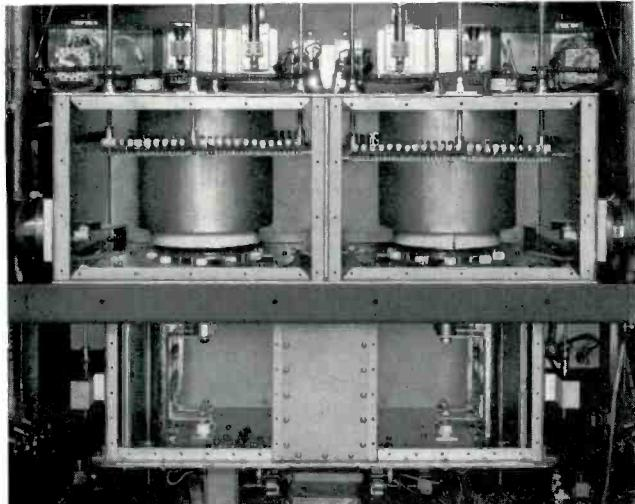
Detailed rear view of r-f amplifier showing aural high-power cavity (right) and one of dplexed visual amplifiers (left) and highlighting accessibility of the high power plate and grid cavities for routine cleaning and maintenance.
