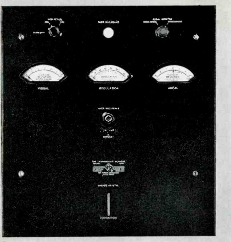
The GR-1184-A-A Monitor Equipment is removable from the front of the rack for servicing and inspection.
