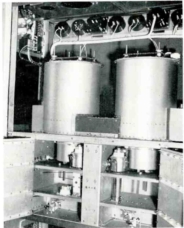
Photo showing the rear of the r-f circuitry—visual left and aural right—with the excellently shielded lower-level stages. Note that each stage occupies its own compartment. This compartment technique eliminates parasitic and other possible interactions between stages.
