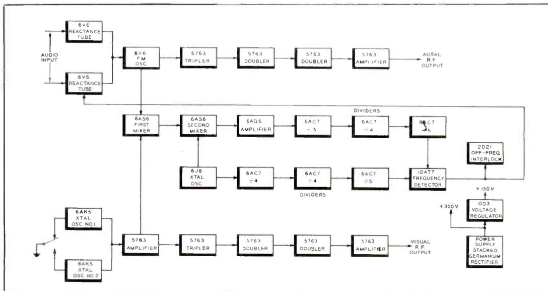
quency of the oscillator is varied at an audio rate to furnish the required FM signal. The mean frequency of the oscillator is controlled by varying the grid bias of one of the reactance tubes. This bias voltage is the d-c output voltage of the frequency detector stage of the exciter.
