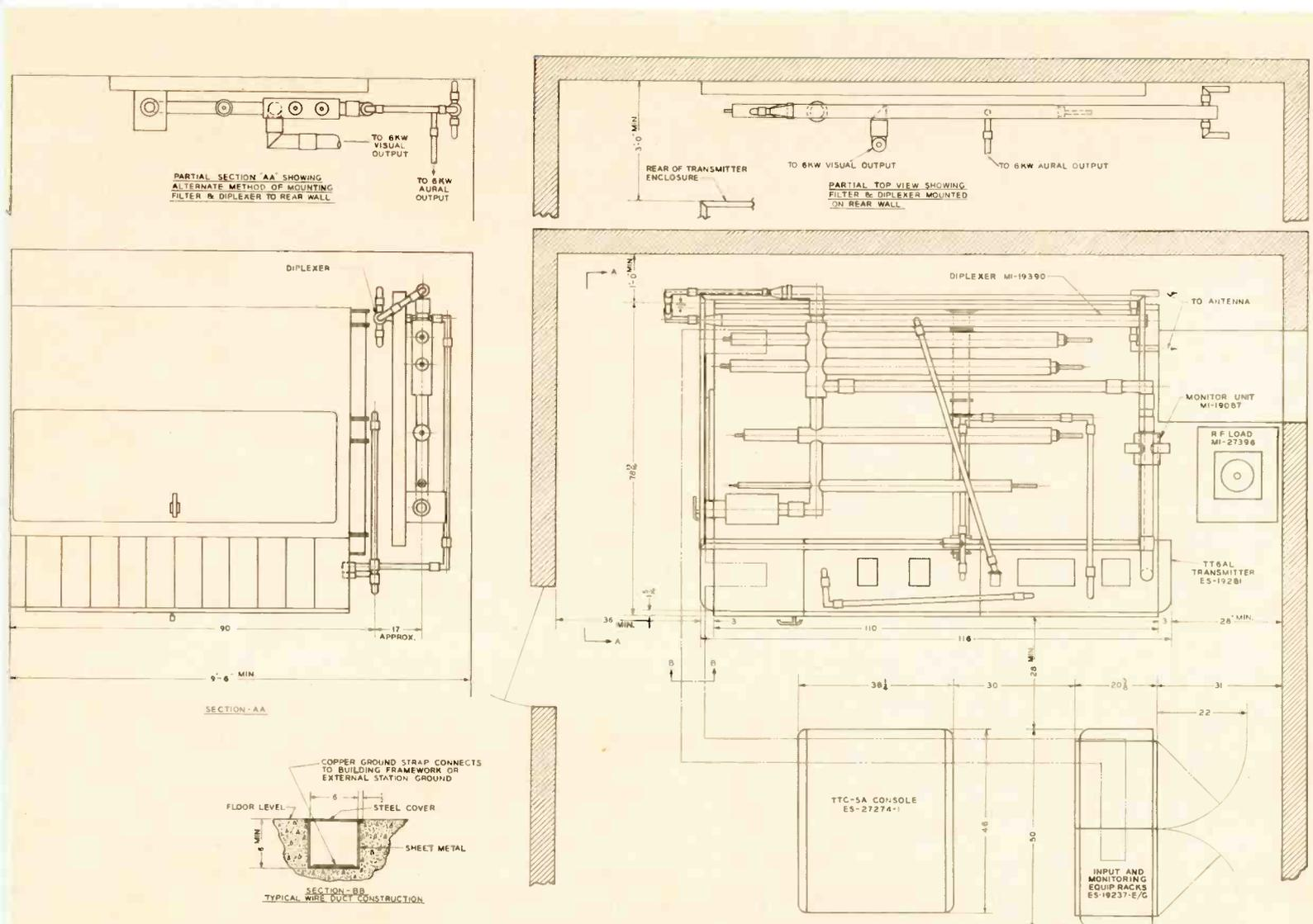
Typical Floor Plan #1 for TT-6AL transmitter with rectifier enclosure attached.
