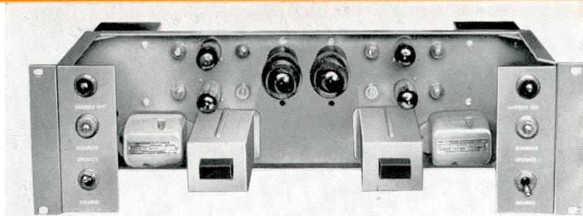
used. One provides a voltage reference level, and the other provides a low voltage which varies with the input signal (reflectometer output). The voltage appearing at the output terminals is therefore proportional to the reflectometer voltage and has good linearity due to the cancellation of Edison effect in the tubes.
