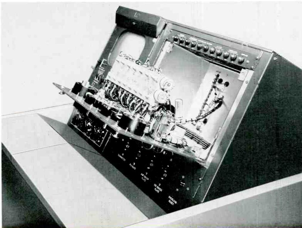
Monitor Control Panel includes four major circuit functions and other related ones, namely, meter circuits, audio monitor circuits, video monitor signal level indication and control.
