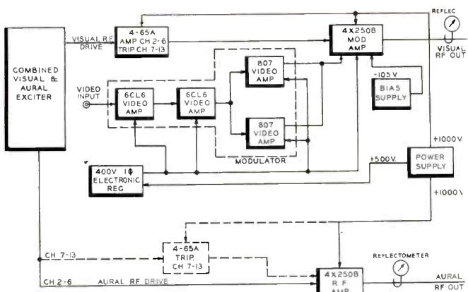
Simplified block diagram of the TTL-100AL/AH Transmitter.
