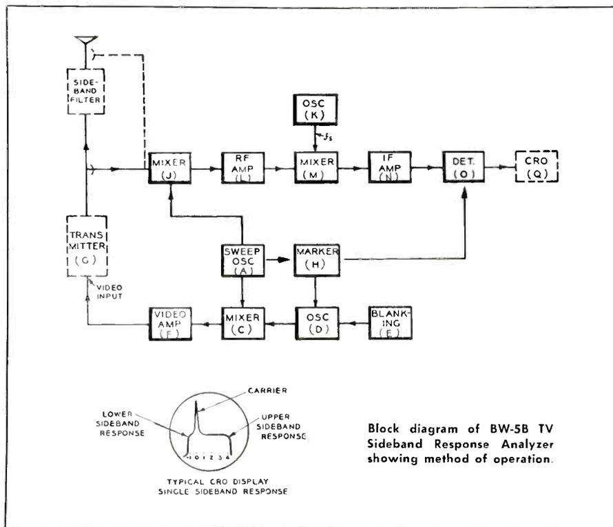
Block diagram of BW-5B TV Sideband Response Analyzer showing method of operation.
