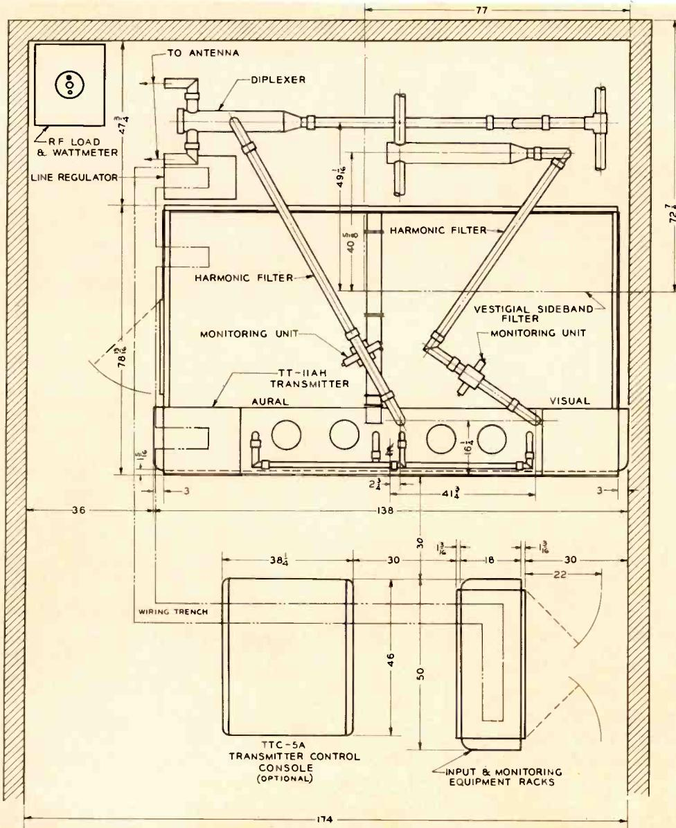
**Typical floor plan arrangement for the TT-11AH Transmitter.** The rectifier enclosure is shown placed immediately behind the front line of cabinets; however, it may be placed in other convenient locations to meet specific building requirements.
