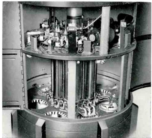
Closeup showing the cluster of seven air-cooled 5762-A triodes used in the 35 kw amplifier equipment.
