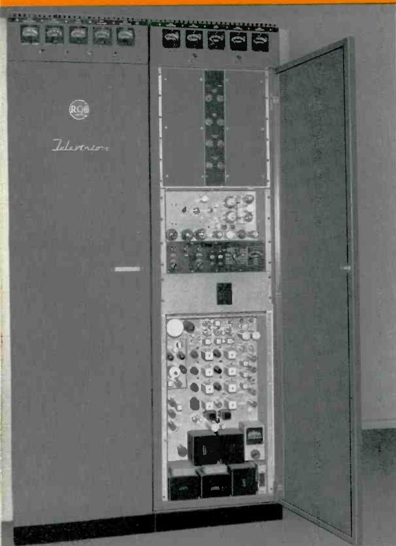
TTL-500AL/AH Transmitter with driver cabinet open.
