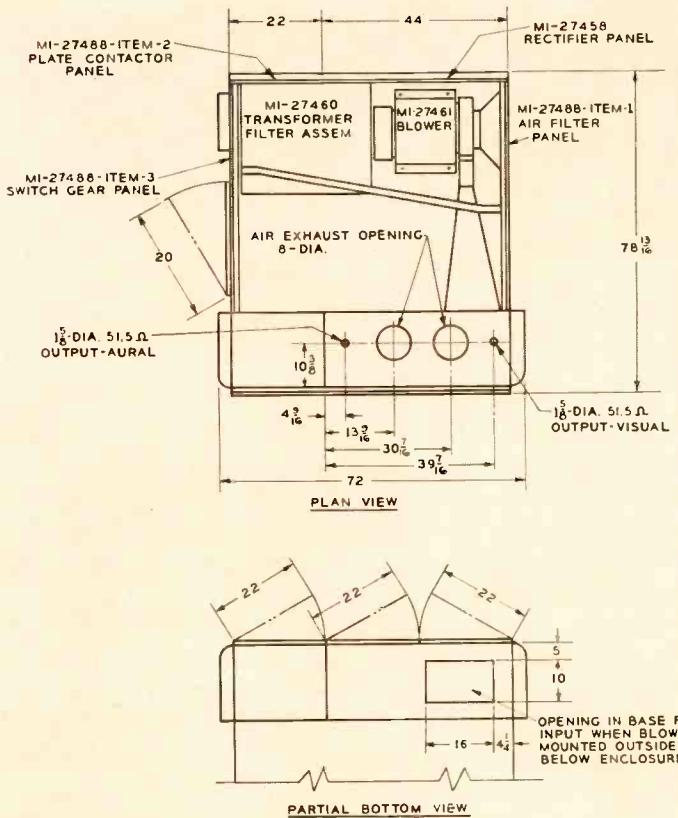
Typical floor plan for the TT-2BH VHF Transmitter showing accessible floor-saving cabinet design.
