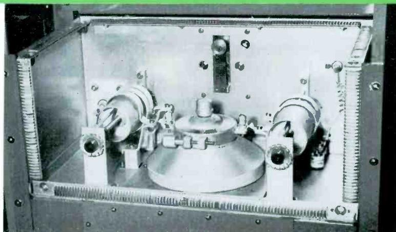
R-f cavity with shielded cover removed.
