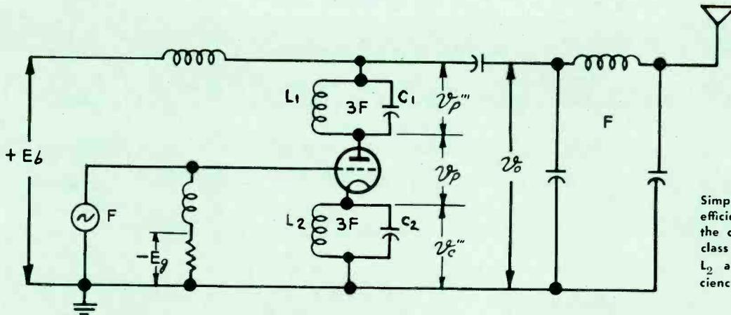
Simplified schematic of the new high efficiency PA stage. The adjustment of the circuit differs from a conventional class "C" only in that the coils  $L_1$  and  $L_2$  are resonated for maximum efficiency.
