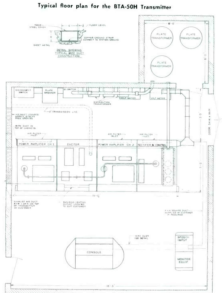
transmitter buildings. The mounting of these components, however, is not critical as to location. They can be mounted in existing power distribution areas if desired. These components include the main plate circuit breaker, a delta-ye switch, a distribution circuit breaker, a 460 to
