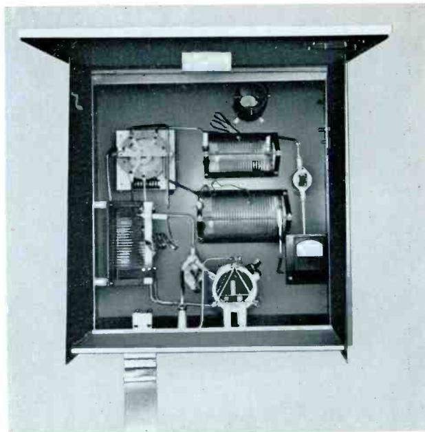
Line Terminating Unit installed in weatherproof cabinet.
