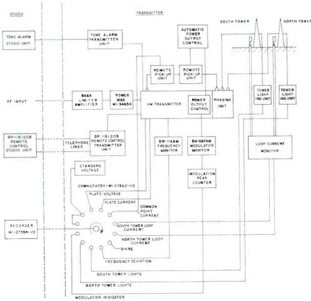
Block diagram of typical remote Automatic Logging Control System for AM Station.
