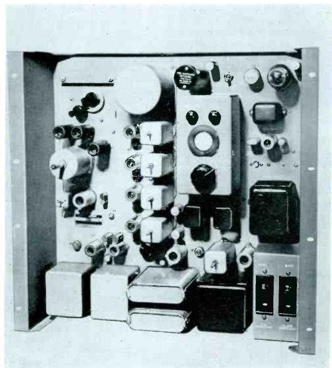
Type BTX-1A Multiplex Subcarrier Generator which is an optional accessory for multiplex operation.
