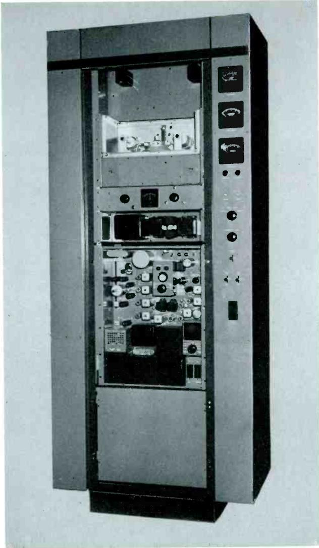
Type BTF-1D transmitter with door and r-f cavity shield removed.
