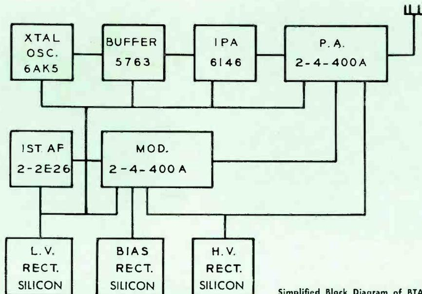
Simplified Block Diagram of BTA-1R1 AM Transmitter.
