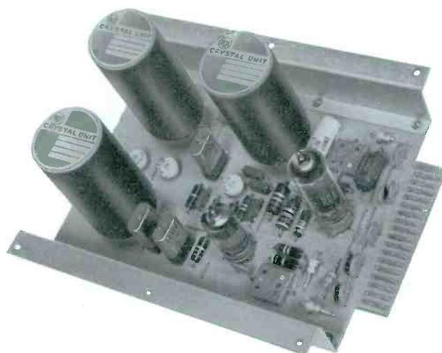
View of oscillator chassis. The terminal strip on right contains all of the oscillator connections. The three crystals are switchable from a front panel control.
