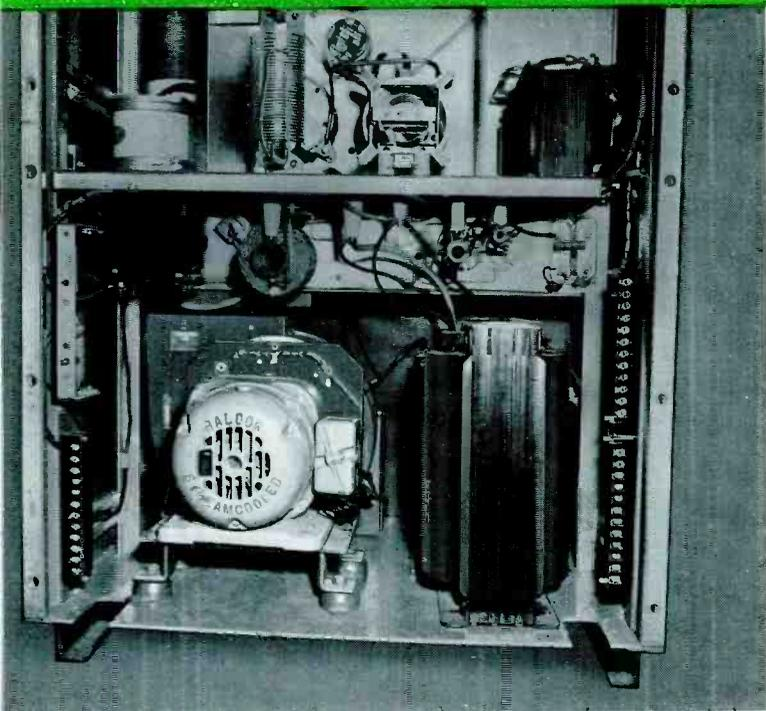
The high efficiency PA permits use of a slow speed blower shown above. The unit is mounted on rubber shock mounts in the base of the PA cubicle. Quiet operation of the blower makes it possible to locate the transmitter in a central control room in smaller stations.
