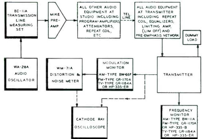
Test set-up for transmitter aural measurements.
