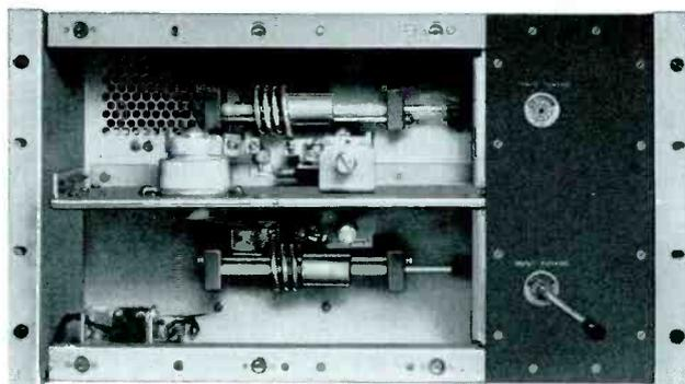
BTF-5D 250-Watt IPA with front panel removed.
