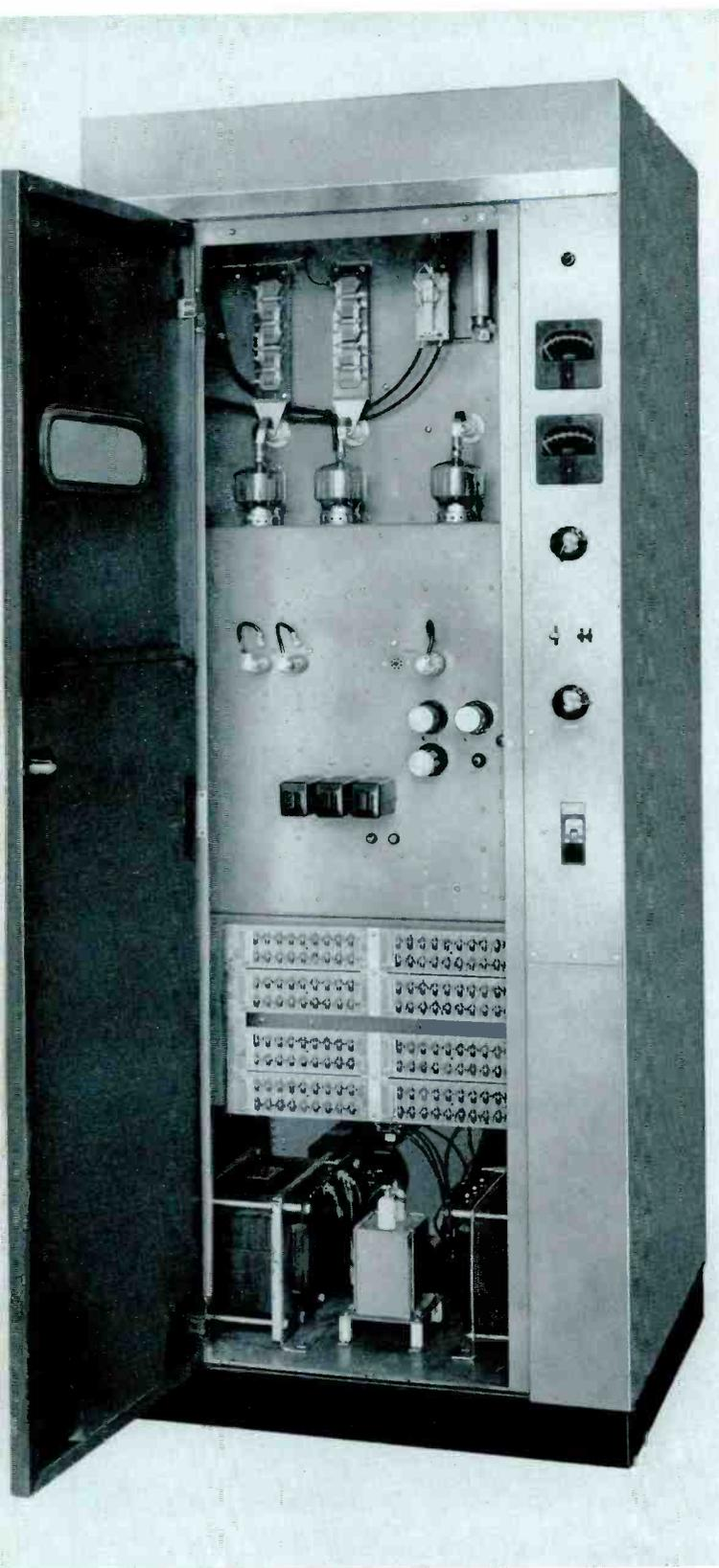
BTA-1R1 Transmitter with front door open showing accessibility of tubes and components. Power Amplifier and Modulator tubes are shown on top chassis; below is exciter chassis. All normal operating controls are shown on two side panels.
