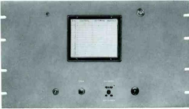
Front view of BTR-20B Transmitter Control Unit.
