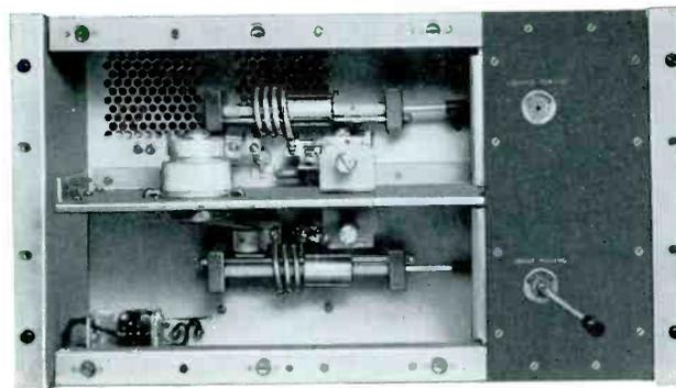
400-Watt IPA stage used to drive the dual 10-kw PA stages of the BTF-20D.
