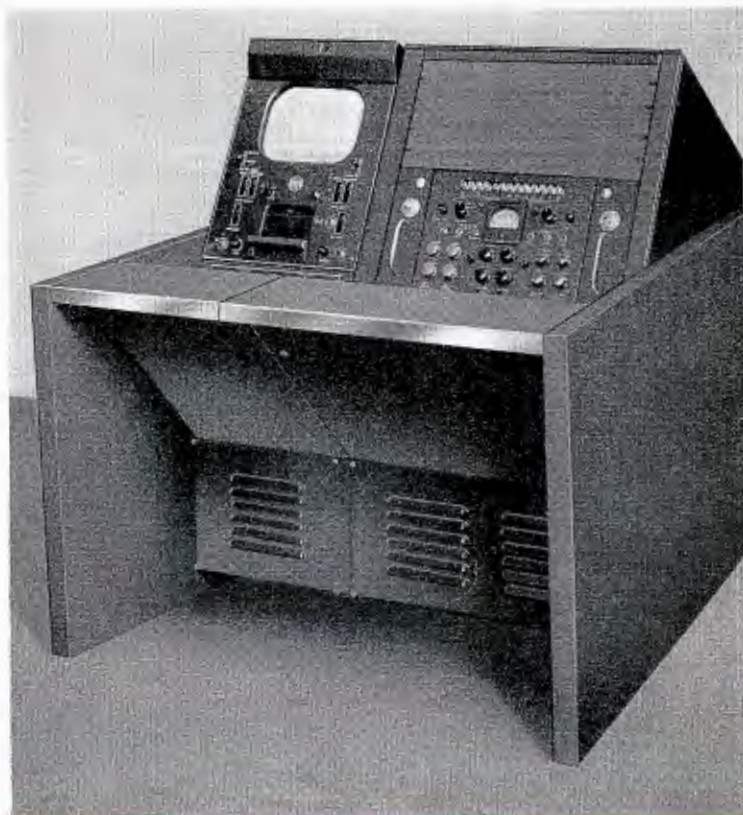
Master Monitor and Processing Amplifier mounted in new console housings. The consoles are also designed to house Camera Control Panel, Color Monitor, and other camera chain equipment.
