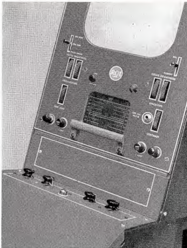
Remote control panel mounts below master monitor for control room operations with waveform and picture display.
