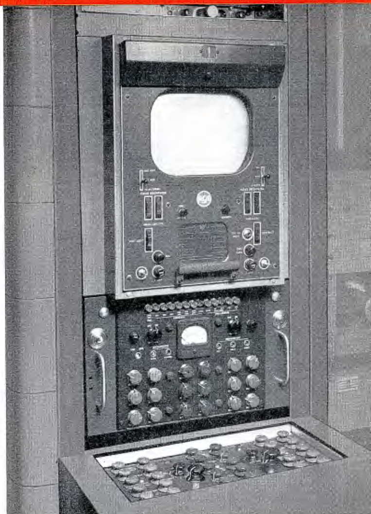
Optional rack mounting for the TK-41 control equipment may be specified. A convenient desk with top panel removed to reveal set-up controls is shown above.
