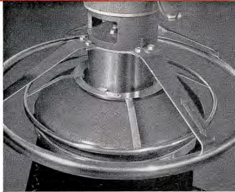
Arrows on steering wheel show direction of wheels. Lower ring locks column and controls drag.
