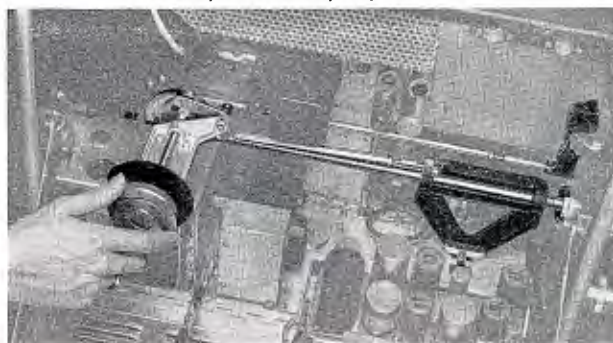
Cam operated focus mechanism provides non-linear travel for easy focus at any object distance.
