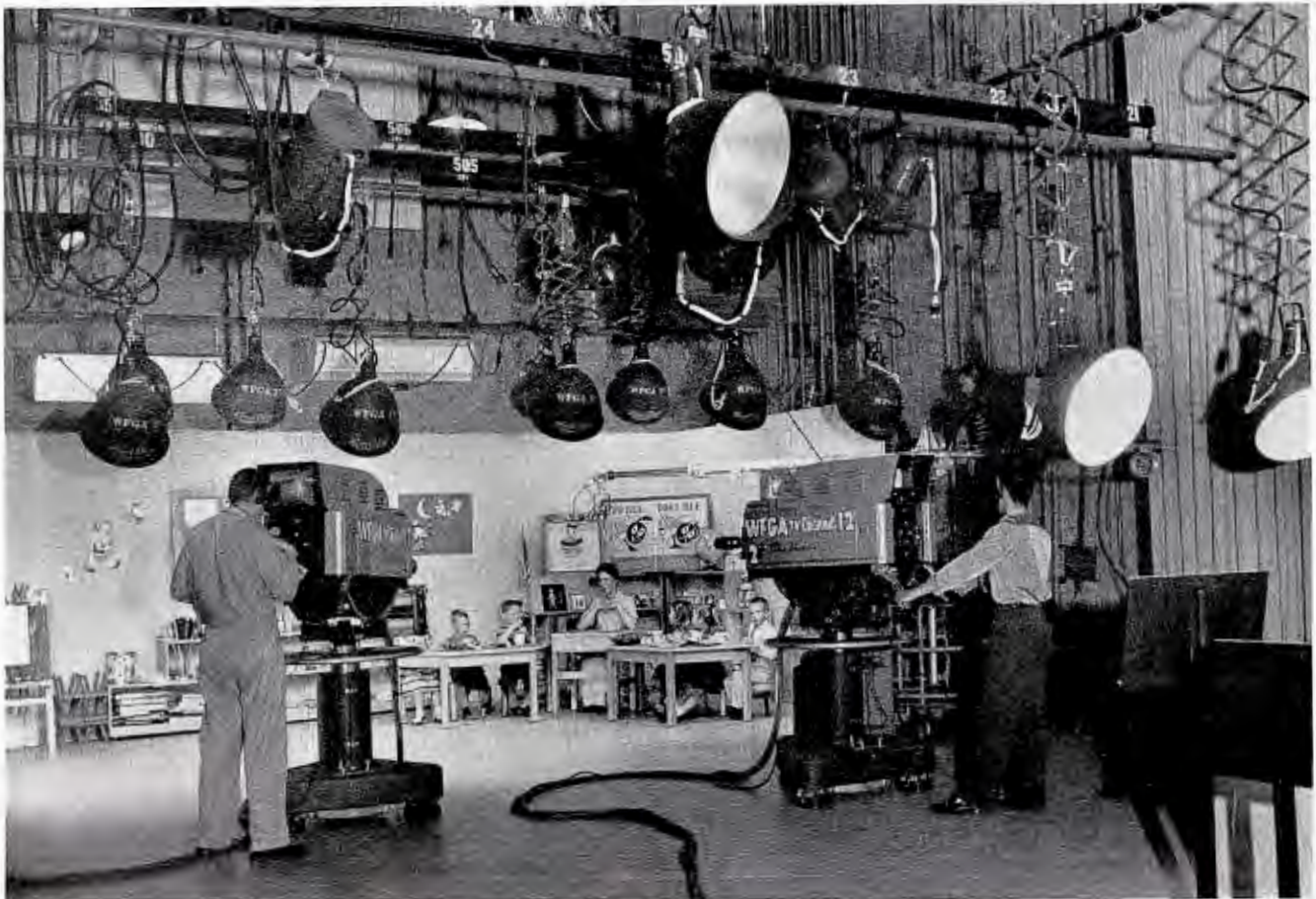
In this studio scene overhead spots and floods are manipulated to provide desired lighting effect.
