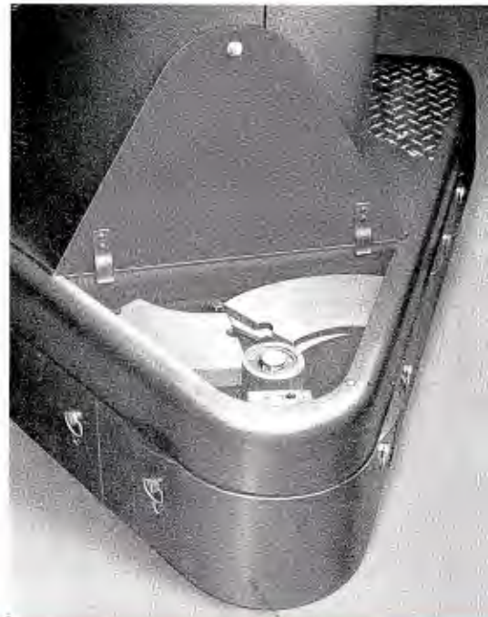
◀ Pedestal with housing removed, showing placement of lead weights for counterbalancing camera.
