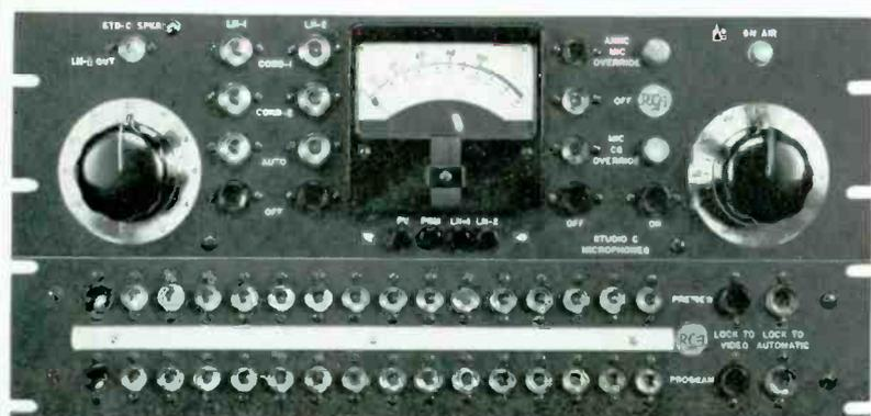
◀ Control and switching units used in the WTAE automation equipment. It permits switching of 15 program or preview program sources.
