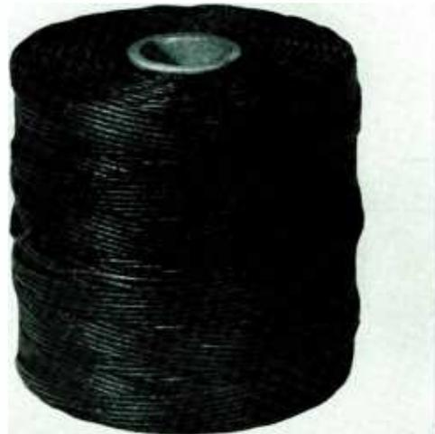
Lacing cord is available for general cable lacing and dressing uses. Cord is of strong material such as linen and hemp and thoroughly impregnated with a beeswax and paraffin mixture. Supplied in one pound spools as shown above.
