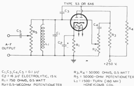
FIGURE 56 - A simple sine-wave audio oscillator of the capacity-feedback type. Figure 57(a) shows the wave form of the output, the frequency being about 1250 cycles per second for the LC constants given above.
