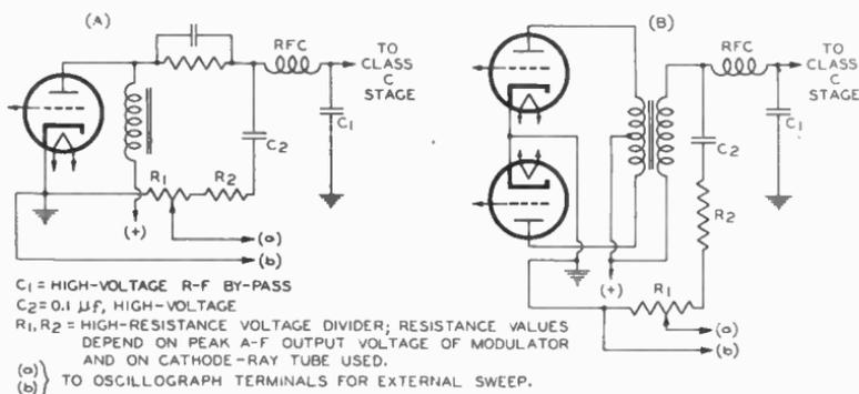
FIGURE 53 - Method of coupling modulator to oscilloscope for trapezoidal patterns.
