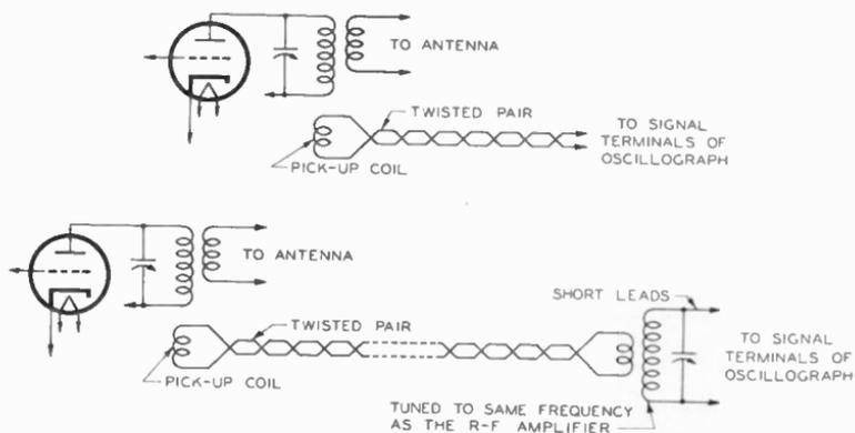
FIGURE 54 - Two methods of coupling r-f amplifier to oscillograph.
