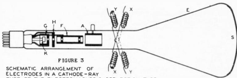
Another type of cathode-ray tube is shown schematically in Figure 3. In this case, no electrostatic deflecting plates are employed. Deflection of the beam both horizontally and vertically is accomplished by means of two electromagnetic fields, produced by two pairs of coils, X and Y. In other respects, this type of tube functions essentially the same as the electrostatic-deflection type.
