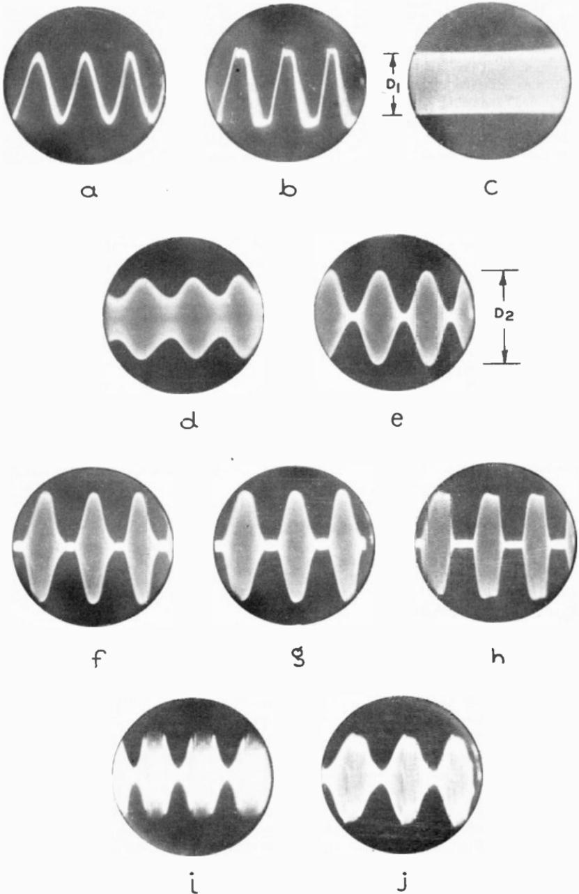
FIGURE 57 - Patterns (d) to (j) obtained by the modulated-envelope method; see text for interpretation.
