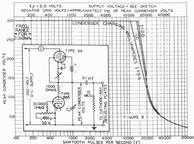
FOR A 0.5 MILLIAMPERE CHARGING CURRENT, SWEEP VOLTAGES MAY BE OBTAINED BETWEEN ESSENTIALLY 0 AND 300 VOLTS FOR A FREQUENCY RANGE UP TO ABOUT 10000 CYCLES. AT HIGHER FREQUENCIES, THE MAXIMUM OBTAINABLE SWEEP VOLTAGE FALLS OFF AS SHOWN ON THE CURVE.
