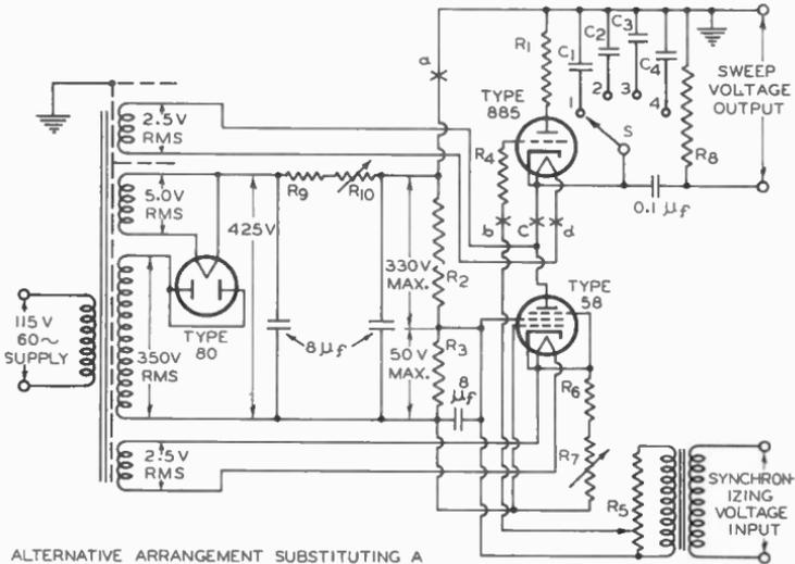
ALTERNATIVE ARRANGEMENT SUBSTITUTING A CURRENT-LIMITING INDUCTANCE FOR  $R_1$  AND PROVIDING AUTOMATIC SELECTION OF PROPER INDUCTANCE FOR EACH CONDENSER SETTING
