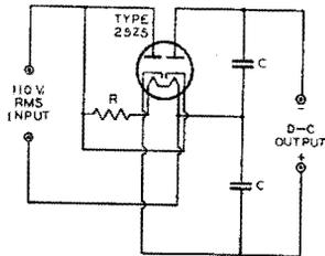
R=HEATER VOLTAGE REDUCING RESISTOR
