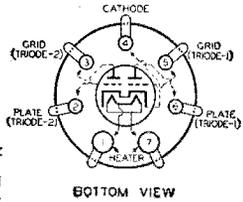
The 53 is a heater-cathode type of tube combining in one bulb two high- $\mu$  triodes designed for Class B operation. It is intended primarily for use in the output stage of a-c operated radio receivers. The
