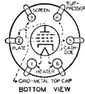
this tube to handle usual signal voltages without cross-modulation and modulation-distortion makes it adaptable to the r-f and i-f stages of receivers employing automatic volume-control. The internal shield around the plate of the 78 is connected to the cathode within the tube.
