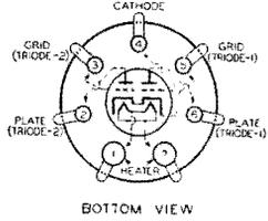
cathodes and heaters, so that circuit design is similar to that of Class B amplifiers utilizing two tubes in the output stage. The 6A6 may also be used as a Class A amplifier (with triode units connected in parallel) to drive a 6A6 as a Class B amplifier in the output stage.
