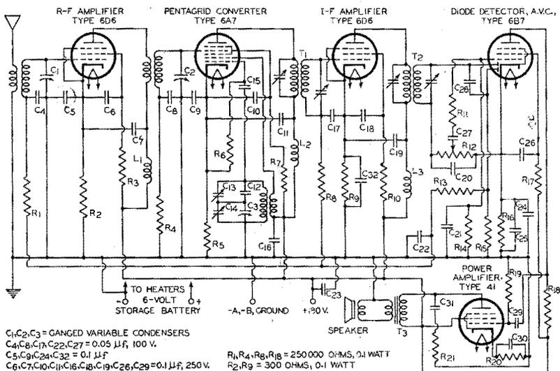
$C_1, C_2, C_3$  = GANGED VARIABLE CONDENSERS
