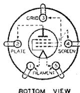
The 33 is a power-amplifier pentode for use in the output stage of battery-operated receivers where economy of battery consumption is important. The 33 is capable of producing greater power
