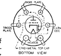
The 75 is a 6.3-volt heater type of tube consisting of two diodes and a high- $\mu$  triode in a single bulb. It is for use as a combined detector, amplifier, and automatic-volume-control tube in radio
