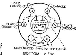
The 79 is a heater-cathode type of tube combining in one bulb two high- $\mu$  triodes designed for Class B operation. It is intended for use in the audio-output stage of radio receivers with 6.3-volt
