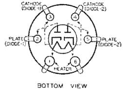
The 25Z5 is a full-wave, high-vacuum rectifier of the heater-cathode type for use in suitable circuits designed to supply d-c power from an a-c power line. This tube is of particular interest because of its
