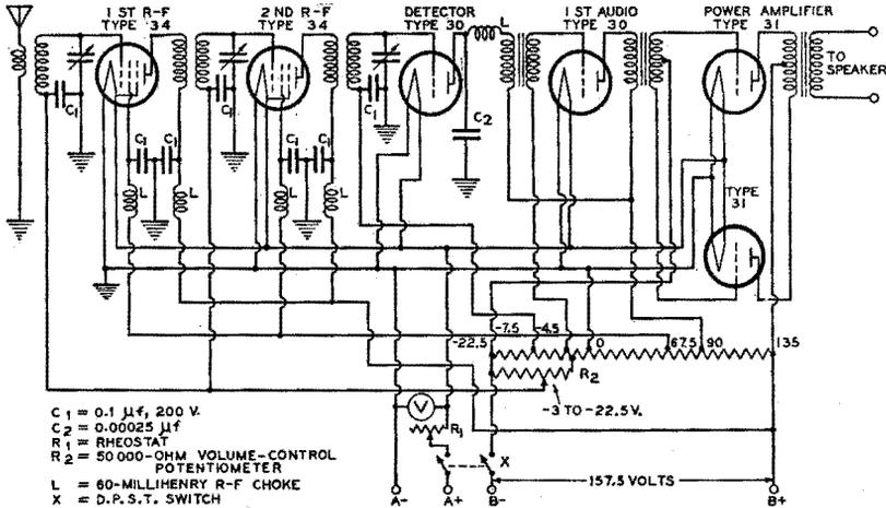
NOTE: THE BLEEDER, WHICH SHOULD HAVE ADJUSTABLE TAPS TO GIVE THE VOLTAGES INDICATED, CAN HAVE A TOTAL RESISTANCE OF 30,000 OHMS.
