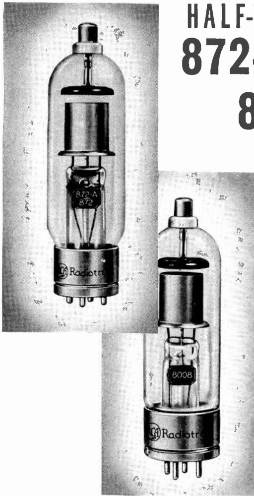
Both are heavy-duty tubes, capable of giving long trouble-free service. The 872-A/872 supersedes both of the older RCA types, 872-A and 872, and combines the ability of the 872-A to withstand high peak inverse voltages and the ability of the 872 to conduct at relatively low applied voltages. The 8008 has the same electrical characteristics as the 872-A/872 but it is equipped with a heavy-duty base.
