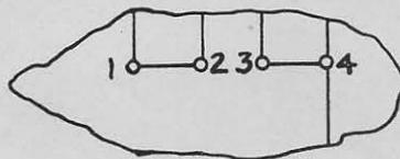
NOTE: Where filament supply is likely to be noisy, or where it is connected through resistance or filter systems which may cause oscillation, reconnect amplifier for no tertiary (0.25 amp.) as shown below:
