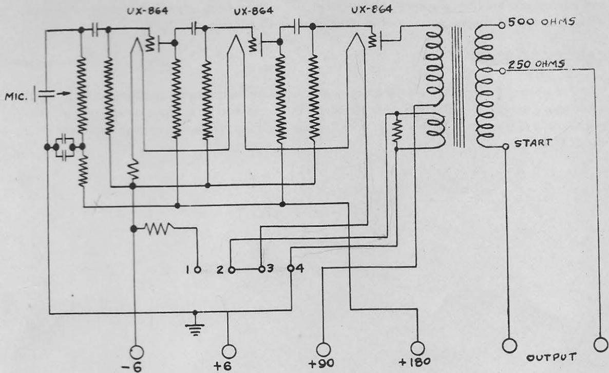
NOTE: Above connection is for 0.25-amp. filament supply.
