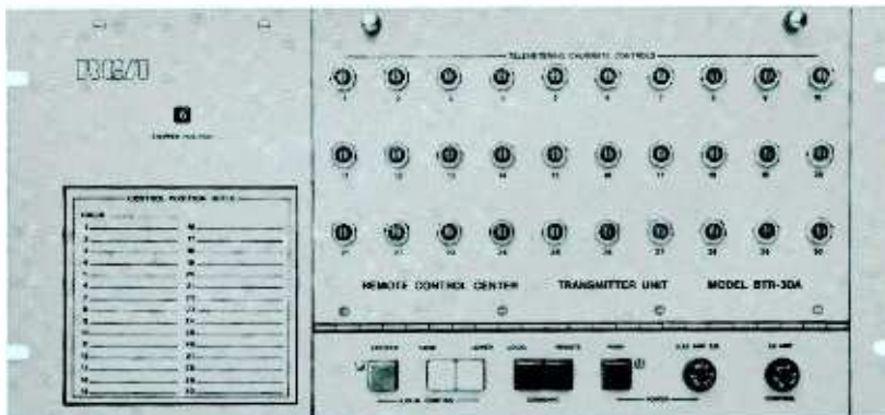
Fold-down front panel in transmitter-control unit provides quick access to all modules. Note 10-turn potentiometers on panel.
