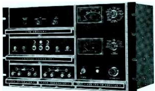
Solid-state FM Exciter system, Type BTE-15A, showing "Direct FM" exciter at upper left with optional stereo generator units shown in place. Right hand module is power supply and metering section.
