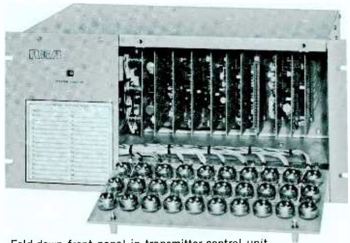
Fold-down front panel in transmitter-control unit provides quick access to all modules. Note 10-turn potentiometers on panel.
