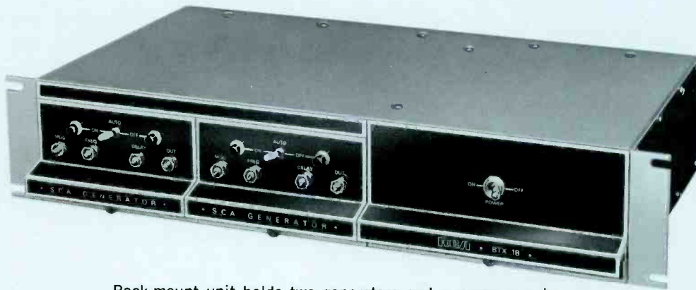
Rack-mount unit holds two generators and a power supply.
