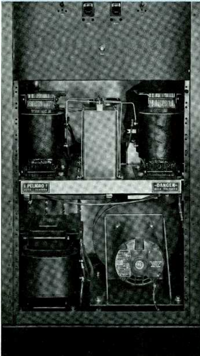
Lower front with access panel removed showing oversized blower, plate transformers and reactors.
