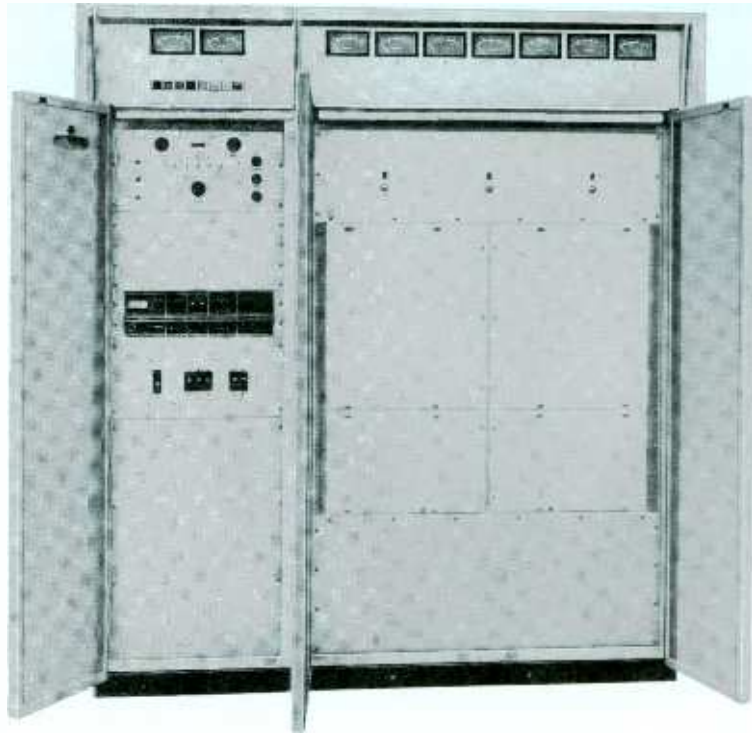
Front view, doors open. Note exciter unit.
