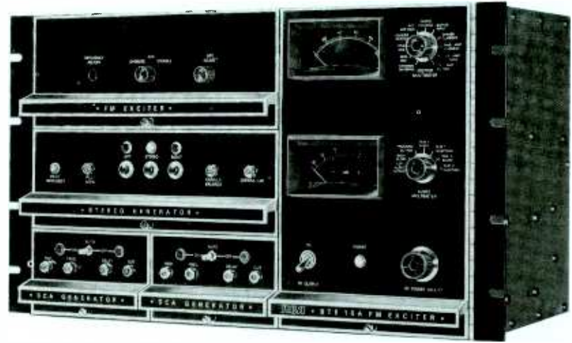
Exciter unit. "Stereo Generator" and two "SCA Generators" are optional. Note dual meters, one for dc parameters, one for audio measurements.
