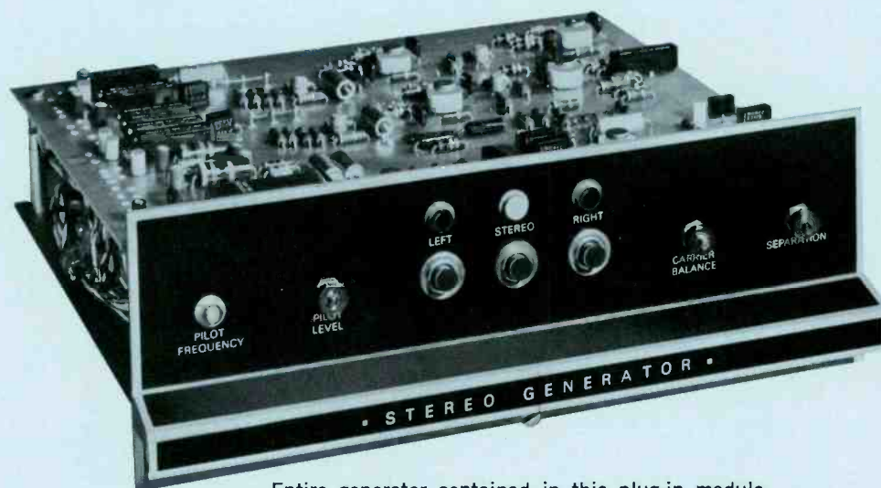
Entire generator contained in this plug-in module.
