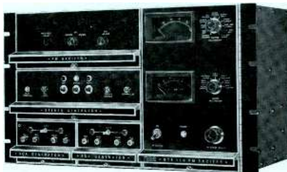
Solid-state FM Exciter system, Type BTE-15A, showing "Direct FM" exciter at upper left with optional subcarrier generator units shown in place. Right hand module is power supply and metering section.
