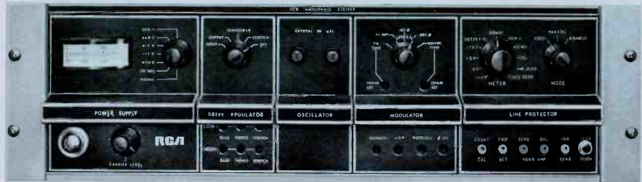
Exciter/modulator unit. Completely solid-state, this unit is used in all RCA Amphiphase transmitters. Available separately for use as a spare. See Accessories.
