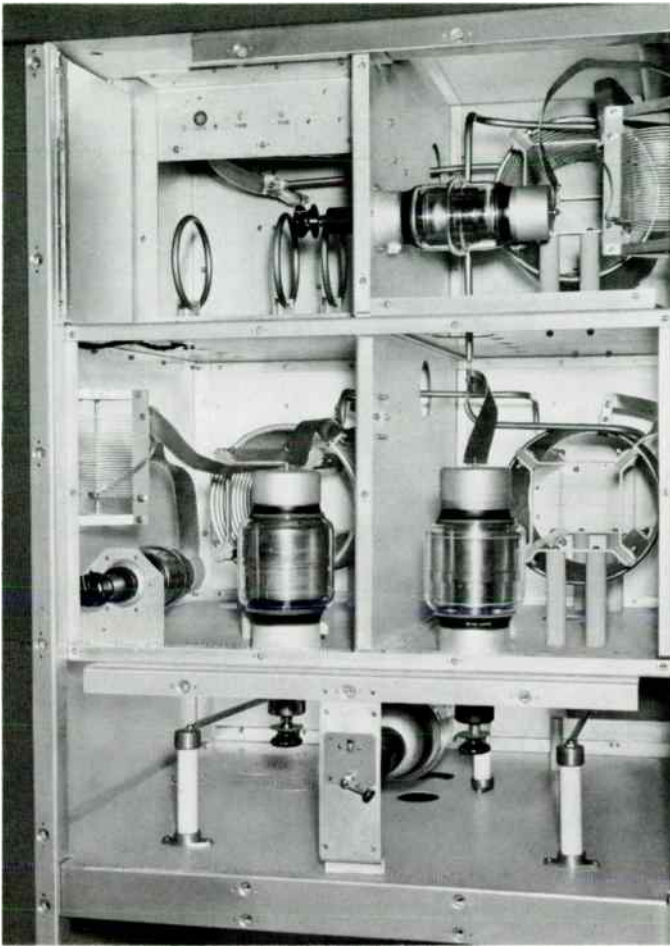
Upper rear of exciter cabinet showing the combining and output networks.
