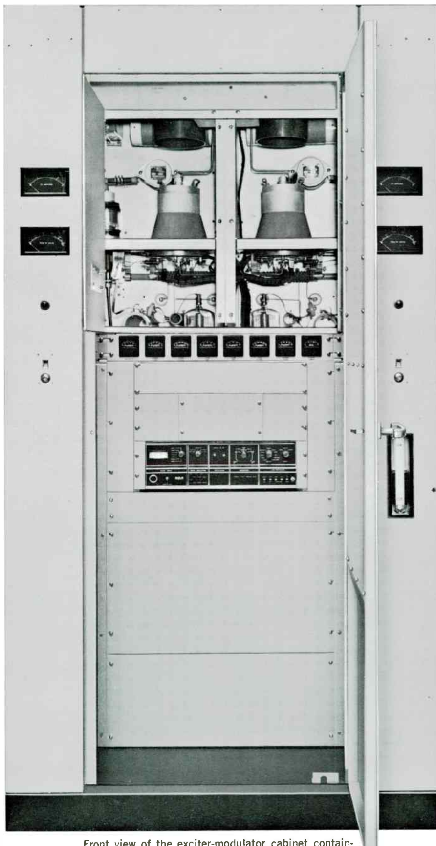
Front view of the exciter-modulator cabinet containing all sections from oscillator through driver stages.
