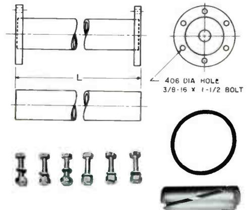
Inner conductor connector included with MI-19313-1NF. Use MI-19313-1SFH or MI-19313-1BSFH for replacement only. Channels between 97 and 99 MHz require 19<sup>1</sup>/<sub>2</sub> foot (5.94 m) sections (MI-19313-1BH or -1BSFH).
