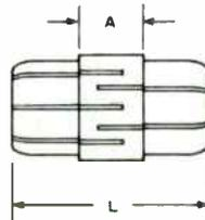
Couples inner conductor of 50 ohm line 6 1/8 inch, MI-561579, to the inner conductor of 51.5 ohm 6 1/8 inch, MI-19314C.
