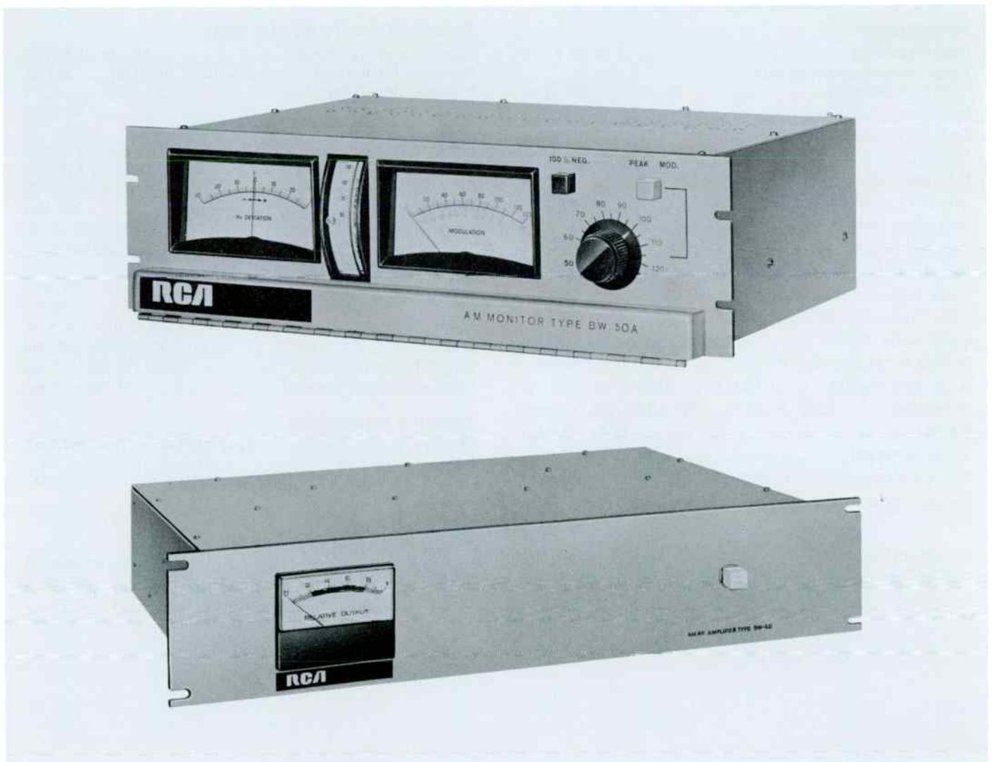
The BW-50 is a solid-state, sensitive AM receiver using a unique new approach to accurate AM transmitter monitoring. It incorporates a highly linear AM detector for modulation monitoring and a digital counter circuit for frequency-deviation monitoring.
