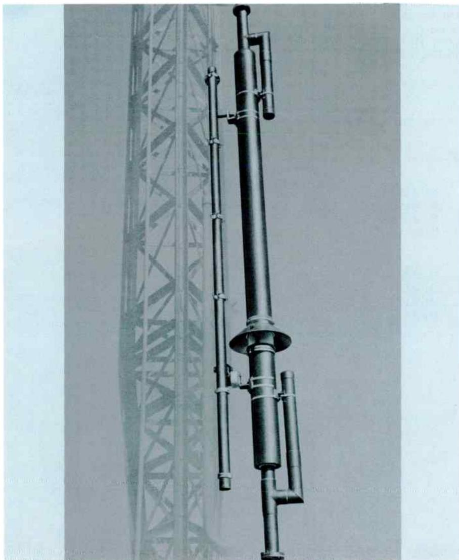
The RCA Type BAF-15A and BAF-16A FM-AM Isolation Units are designed to transfer FM power across the base insulator of an AM antenna tower to feed an FM antenna mounted atop the tower. The units provide isolation of FM and AM signals and efficient operation over the entire FM frequency range.
