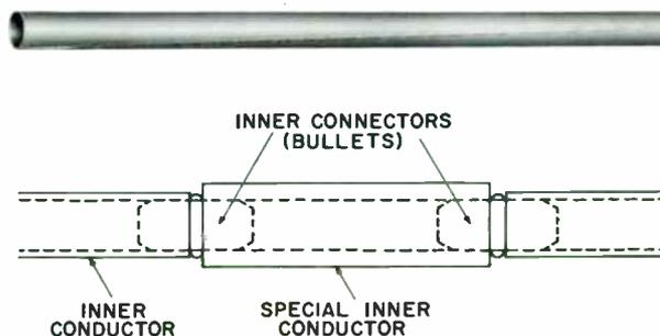
Oversize inner-conductor tube for splicing MI-19113C line when cut at point other than midway between insulators. Each splice requires two MI-19113C-11 inner-conductor connectors. (Not supplied, see below.)
