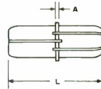
Couples inner conductor of 1 1/8 inch 50 ohm line (MI-561565) to inner conductor of 1 1/8 inch 51.5 ohm line (MI-19112).
