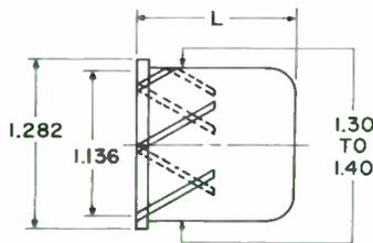
Reduces inner diameter of MI-19313 inner conductor to mate with MI-19113 component inner conductors.
