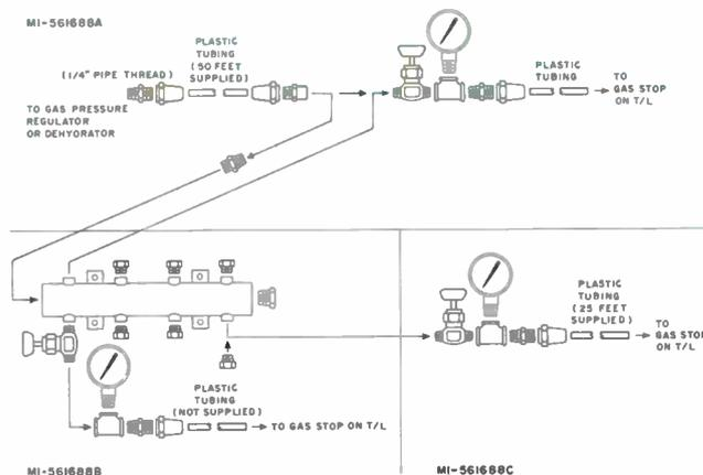
There are three gassing system kits: an "A" kit which is basic to Kit "B" which, in turn, is basic to Kit "C".
