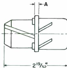
Connects inner conductors of MI-19113C line with those of MI-19313 line.
