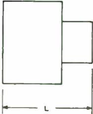
Reduces unflanged 6 1/8 inch line (MI-561579) to unflanged 3 1/8 inch line (MI-27791K). Requires coupling MI-27791K-4A (not supplied). Coupling for 6 1/2 inch end included with two clamps.
