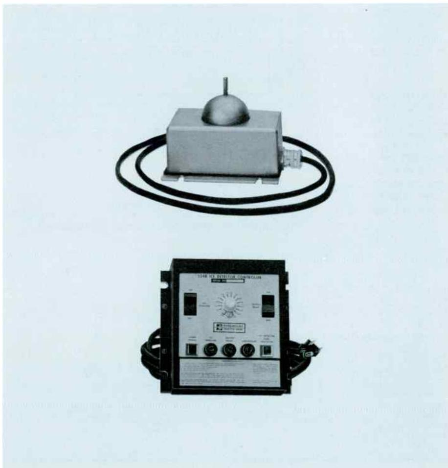
Active only during antenna-icing weather, the Rosemount Antenna Ice Detector senses buildup of broadcast-antenna ice and generates a signal which, with appropriate power-contacter equipment (not supplied), automatically energizes an antenna's sleetmelters. At the conclusion of icing conditions, the device automatically de-energizes the heaters after an adjustable time-delay period expires.
