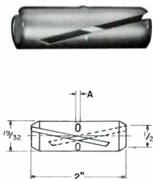
Joins inner conductors of MI-19113 components at joints or splices.
