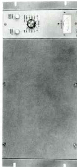
Marti remote-pickup transmitter. Four audio inputs and a multi-purpose front-panel meter. Available for 150-172 and 450-470 MHz bands.
