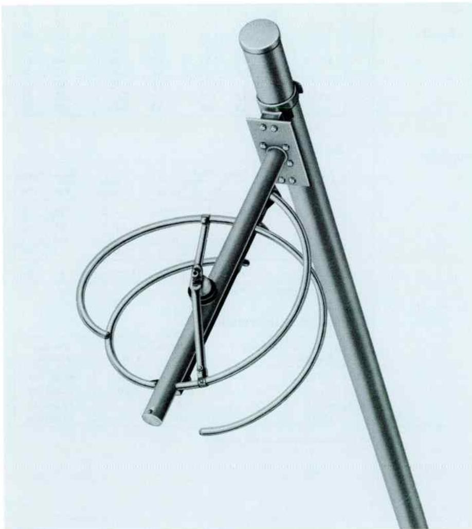
The BFI- antenna series are low-power elements for the 10-watt educational/campus FM station. It is available in circular or horizontal polarization in one- or two-section arrays. Mounting brackets are not included. Connector is Type "N". Specifications and ordering information in next page.
