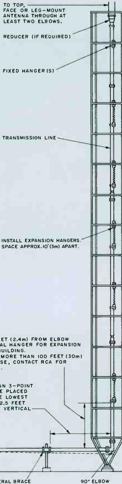
ALLOW EIGHT FEET (2.4m) FROM ELBOW TO FIRST VERTICAL HANGER FOR EXPANSION OF LINE FROM BUILDING. IF BUILDING IS MORE THAN 100 FEET (30m) FROM TOWER BASE, CONTACT RCA FOR THIS DIMENSION.
