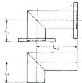
Flanged elbow uses swivel flanges and includes inner-conductor connector, O-ring gasket, six bolts, nuts, lockwashers. Unflanged elbow includes inner-conductor connector only.
