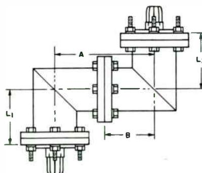
All flanges swivel. Includes one O-ring gasket, two captive connectors, twelve bolts, nuts, lockwashers.
