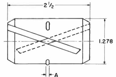
For joining inner conductors of MI-19313 transmission line sections.
