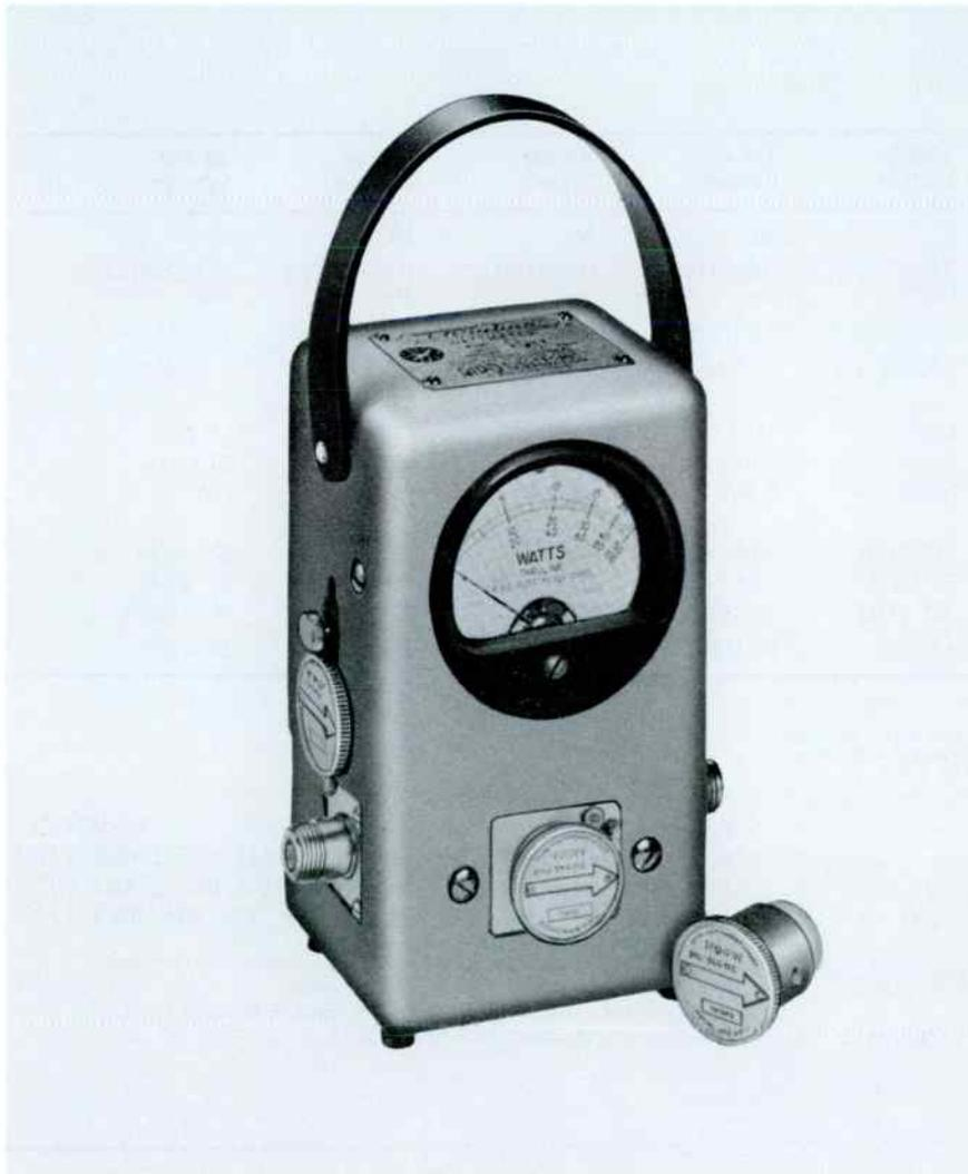
The loads and wattmeters described here are dual-purpose units. As non-inductive dummy loads, they aid in transmitter tune-up without radiation; as wattmeters, they terminate the transmitter output and indicate an accurate measure of power output.
