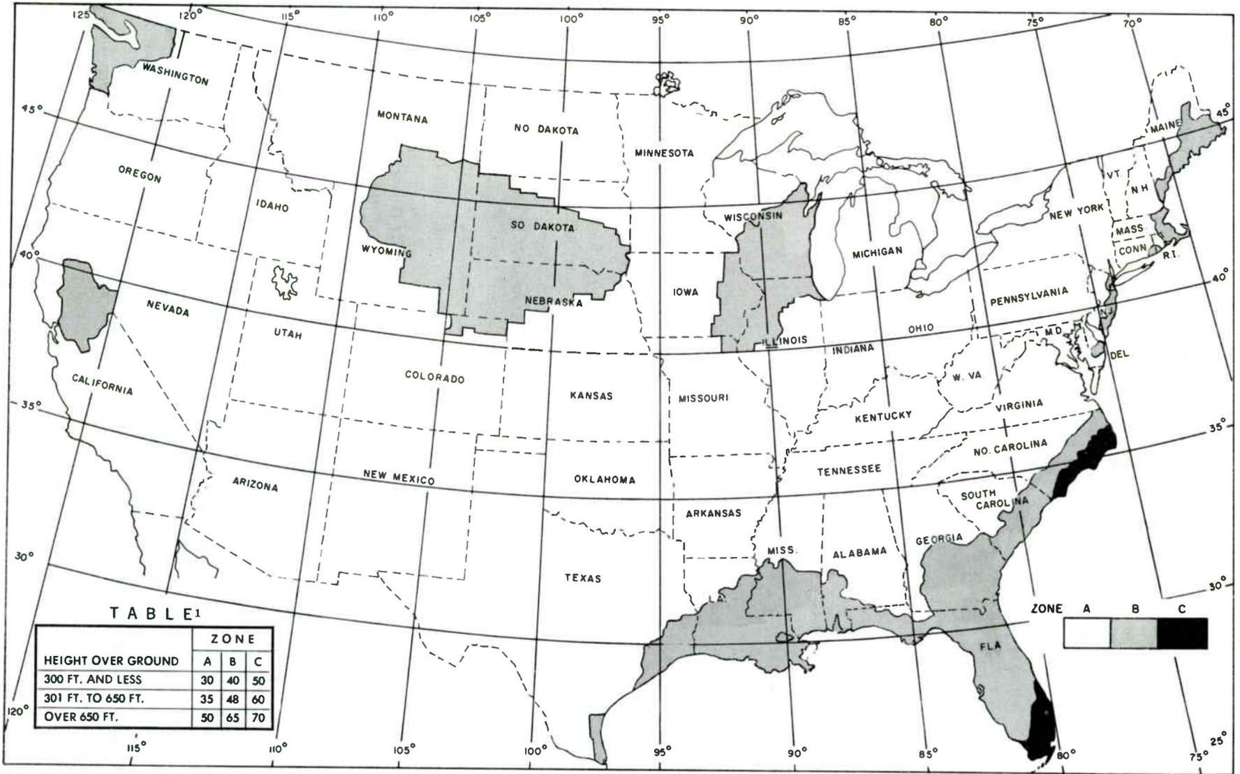
This map and table, extracted from EIA Standard RS-222B, gives minimum horizontal design windload pressures in pounds per square foot, on flat surfaces and with no ice for the zones indicated. The map, as well as the table, must be interpreted in view of local knowledge and applicable building codes. See RS-222B for zone boundaries defined by state and county.
