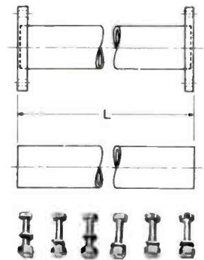
Shipped two sections per package. Use MI-19113C-1SF (swivel flange) for field replacement only. Channels between 97 and 99 MHz require 19 1/2 foot (5.94m) sections (special order only).
