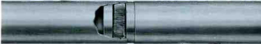
Teflon-insulated 51.5 ohm line is available in flanged and unflanged styles and features a "wristband spring" inner-conductor expansion joint that prevents galling and contamination of the insulation.
