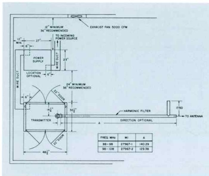
Space-saving floor plan of the BTF-10E1. The separate, unitized power supply may be installed in the basement, attic, closet, or other convenient place. (Wire duct and fan shown are not furnished.)
