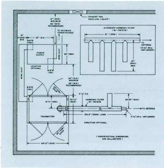
Space-saving floor plan of the BTF-20E1. Some units use three-inch diameter harmonic filter (inset). The separate, unitized power supply may be installed in a basement, attic, closet or other convenient place. (Wire duct and fan shown in drawing not furnished.)
