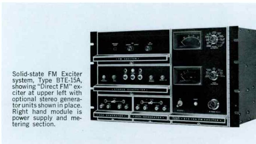
Solid-state FM Exciter system, Type BTE-15A, showing "Direct FM" exciter at upper left with optional stereo generator units shown in place. Right hand module is power supply and metering section.
