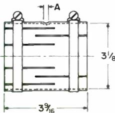
Couples unflanged line sections and components. Omits inner connector.
