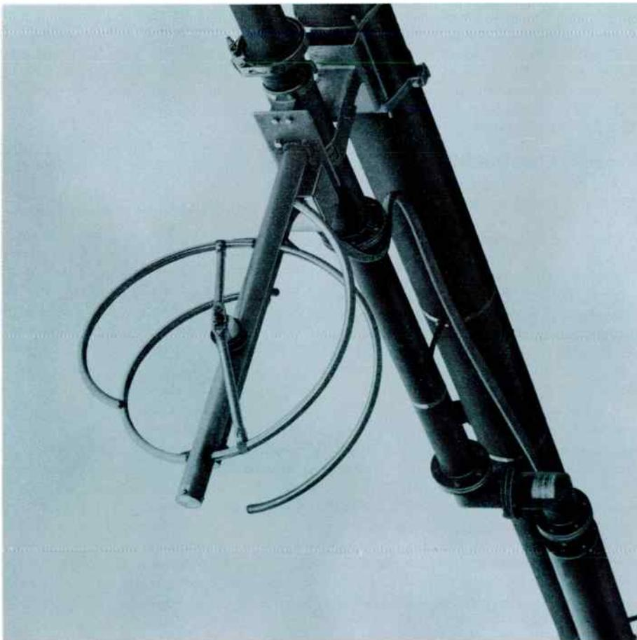
The most popular RCA FM antenna. The BFC-antenna is a circularly polarized device with a power rating of 4kW per section (10kW with radomes) and available in stacked arrays of up to 16 sections with an input rating to 40 kilowatts. For situations where ice formation is common, the arrays can be equipped with electrical de-icers or radomes. Both are options at extra cost.
