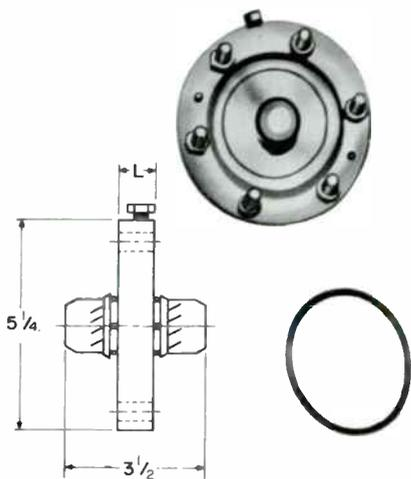
Seals pressurized section from unpressurized. Fits MI-19113C or MI-19313 components. O-ring gasket and hardware (six bolts, nuts, lockwashers) included.
