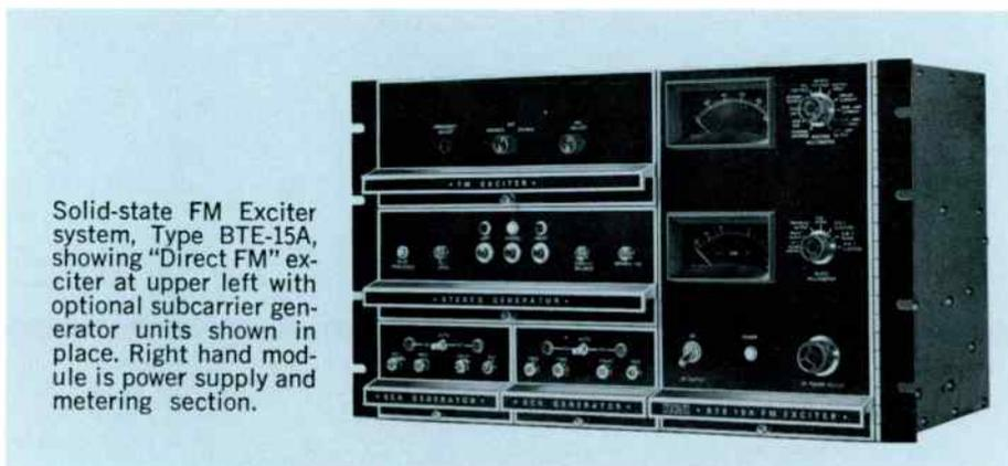
Solid-state FM Exciter system, Type BTE-15A, showing "Direct FM" exciter at upper left with optional subcarrier generator units shown in place. Right hand module is power supply and metering section.
