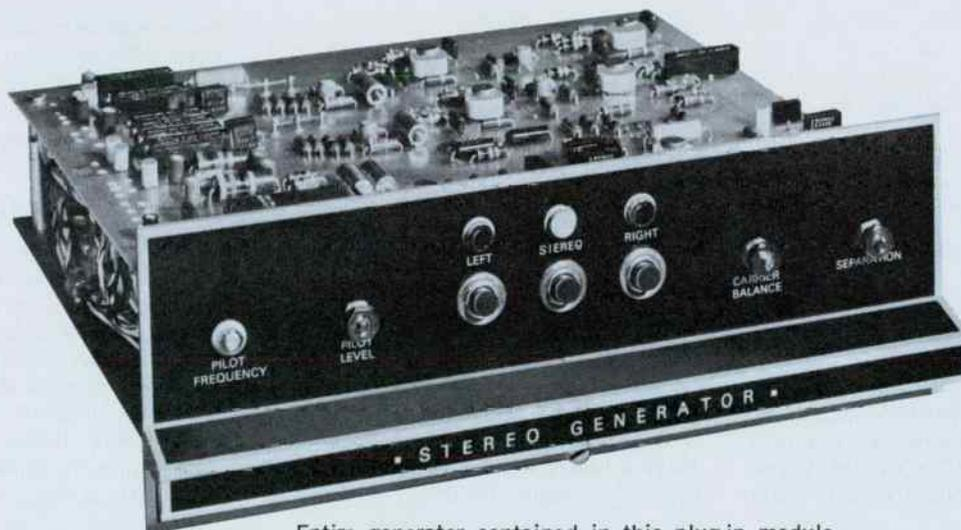
Entire generator contained in this plug-in module.
