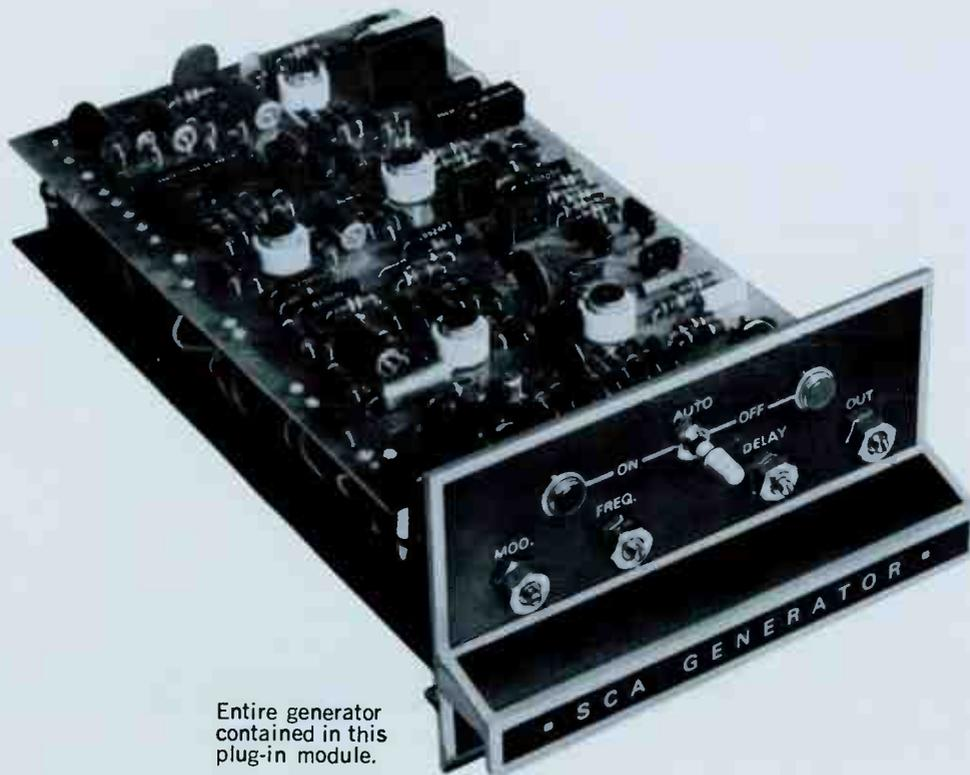
Entire generator contained in this plug-in module.
