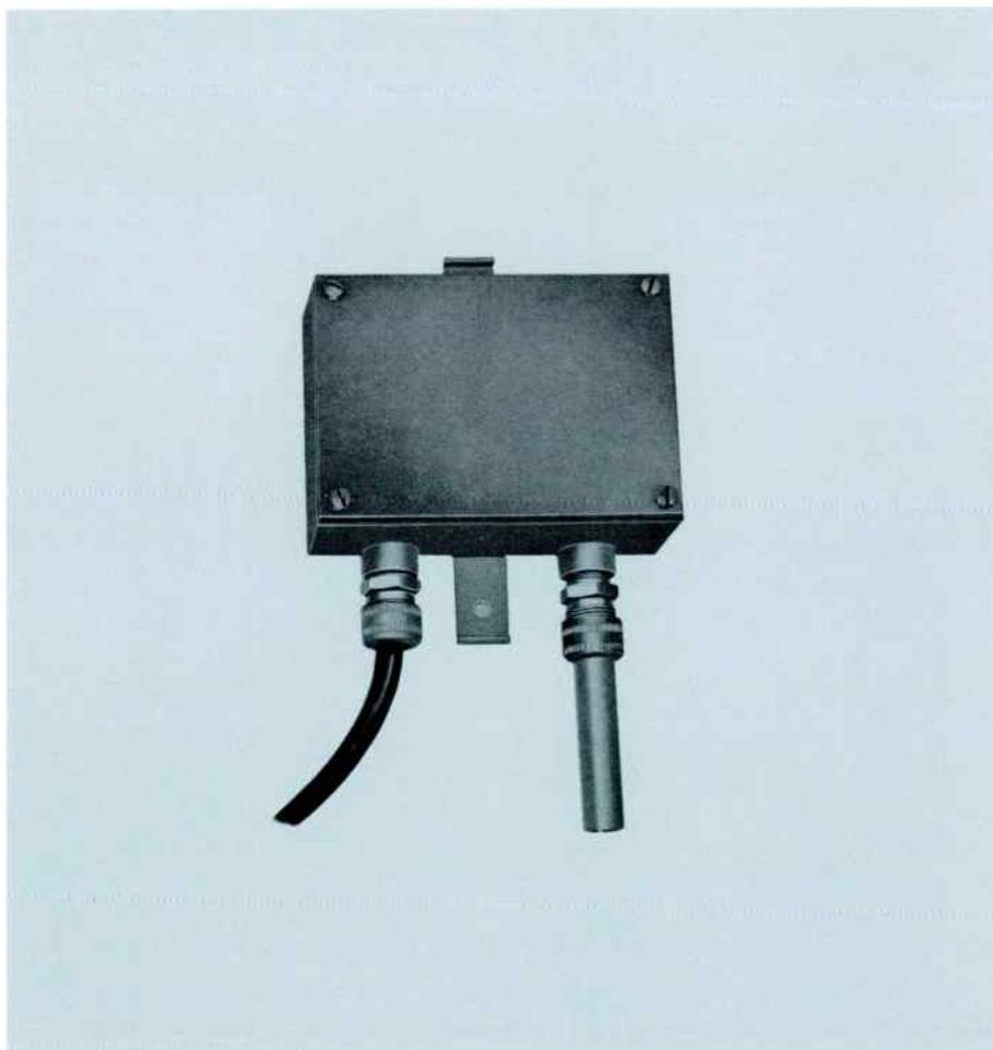
The Automatic Sleet Melter Control Unit prevents severe damage to transmission equipment through automatic thermostatic control of antenna de-icers. The control allows de-icers to be left unattended at all times and proper operation is assured. Furthermore, the antenna will be free of ice and in condition for immediate operation following possible icing conditions during the night.
