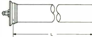
Transforms 6 1/8 inch 50 ohm (MI-27791K) to 6 1/8 inch 75 ohm (MI-27792D) and provides Universal female flanges. Specify channel or frequency when ordering.
