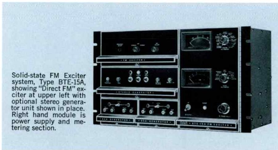
Solid-state FM Exciter system, Type BTE-15A, showing "Direct FM" exciter at upper left with optional stereo generator unit shown in place. Right hand module is power supply and metering section.
