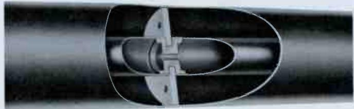
Efficient, precision-built line and line accessories. Featuring an electrically transparent Teflon insulator, this line uses the familiar bolt-flange connection. Insulator characteristics and precise inner-conductor centering allows cutting and re-flanging in the field without a change in operating impedance at the cut.
