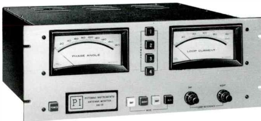
The PM-19 system uses the AM-19 (204) Antenna Monitor as a base and adds to it a PMA-19 Precision Monitor Adapter. The combination of the two units increases resolution and repeatability to one-tenth degree for phase angle and one-tenth percent for current deviation measurements. The system reads out loop current ratios directly. The system provides both analog and digital readout of all three parameters.
