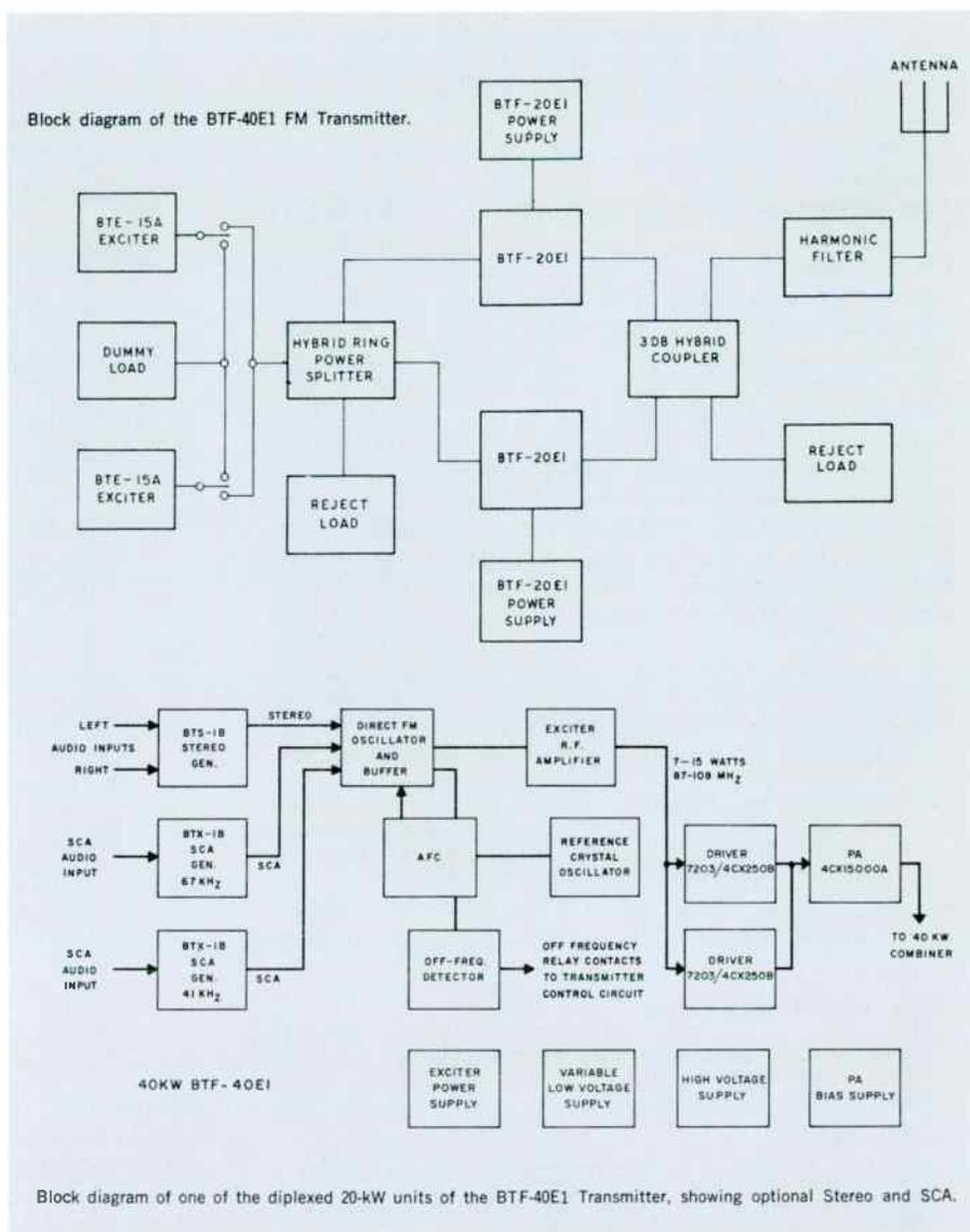
Block diagram of one of the diplexed 20-kW units of the BTF-40E1 Transmitter, showing optional Stereo and SCA.
