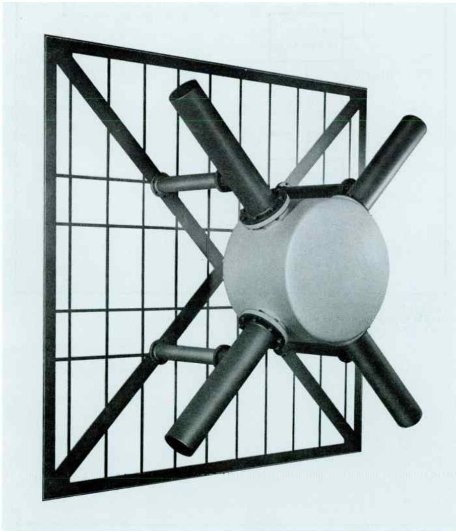
FM Panel Antennas, Types BFB, BFD, BFE and BFF are broadband, custom-tailored antenna systems that permit a number of high powered FM stations to share a common antenna. They are circularly polarized for optimum coverage and perform excellently in either omnidirectional or directional applications. Bandwidths range from 4.5 to 20 MHz in the FM broadcast band, and power ratings extend up to 80 kilowatts (CW) per panel.
