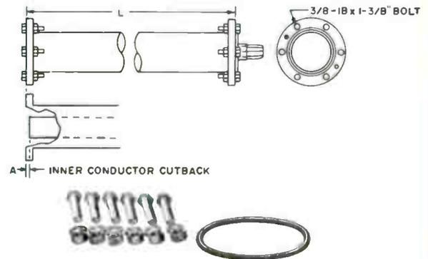
Shipped two sections per package. Each section includes one captive anchor insulator-connector, expansion joint, O-ring gasket, six bolts, nuts, lockwashers.
