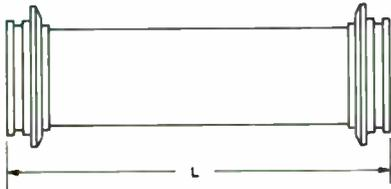
Couples female ends of line with two male flanges. Two O-ring gaskets included.
