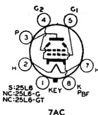
The 25L6, 25L6-G, and 25L6-GT are beam power amplifier tubes of the heater-cathode type designed for use in the output stage of "transformerless" (a.c.-d.c.) receivers. These tubes provide high power output at the relatively low plate and screen voltages available for transformerless receivers. The high power output is obtained
