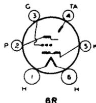
The tube, therefore, is essentially a voltage indicator and as such is particularly useful as a convenient and non-mechanical means to indicate accurate tuning of a receiver to the desired station. The 6E5 is similar to the 6U5/6G5 except that the 6U5/6G5 triode unit is designed with a remote plate-current cut-off characteristic. For discussion of Electron-Ray Tube considerations, refer to RADIO TUBE APPLICATIONS section.
