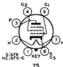
because of the heater-cathode construction, uniformly low hum-level is attainable in power-amplifier design.
