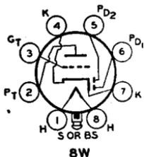
The 7B6-LM is a multi-unit tube of the locking-base type containing two diodes and a high-mu triode in one envelope. The 7B6-LM is designed for use as a combined detector, amplifier, and automatic-volume-control tube. The triode unit is recommended for use in resistance-coupled amplifier service and may be used under the same conditions as given for the 6SQ7 in the RESISTANCE-COUPLED AMPLIFIER CHART. The
