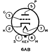
For heater operation and cathode connection, refer to Types 12A8-GT and 6A8, respectively.
