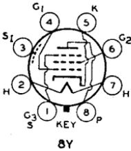
RCA-6AG7 is a heater-cathode type of metal tube intended for use primarily in the output stage of the video amplifier of television receivers. It may also be used advantageously in television transmitters as a coupling device between video-frequency stages and transmission lines.
