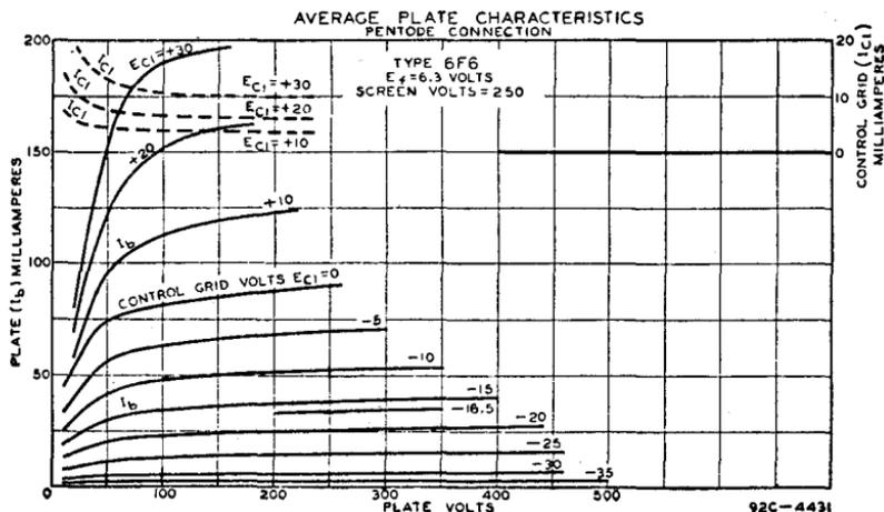
recommended. When the grid circuit has a resistance not higher than 0.1 megohm, fixed bias may be used; for higher values, cathode bias is required. With cathode bias, the grid circuit may have a resistance as high as, but not greater than, 0.5 megohm provided the heater voltage is not allowed to rise more than 10% above rated value under any condition of operation.
