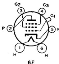
istics. The ability of the tube to handle the usual signal voltages without cross-modulation and modulation distortion makes it adaptable to the r-f and i-f stages of receivers employing automatic volume control. The 6D6 is constructed with an internal shield connected to the cathode within the tube. Except for capacitances, given below, the electrical characteristics of the 6D6 are identical with those of the 6U7-G.
