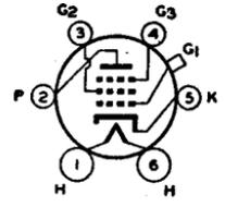
SECTION. The base of the 57 fits the standard six-contact socket which may be installed to hold the tube in any position. For heater operation and cathode connection, refer to Type 2A5. For screen voltage and shielding requirements, see Type 6C6.
