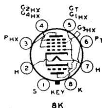
The 6K8 is a multi-electrode tube of metal construction consisting of a triode oscillator and a hexode mixer in a single envelope. The design of the 6K8 reduces interaction between the oscillator and mixer sections of the tube, and thereby permits optimum performance at the high as well as the low radio frequencies.
