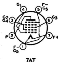
within a single tube. The 1R5 is designed with high operating efficiency especially for compact, light-weight, portable equipment. The high operating efficiency even with only a 45-volt B-supply has been attained by a new design which provides the miniature size without decreasing the size of essential electrode parts. The conventional base has been replaced with a glass button base. For general discussion of pentagrid types, see Frequency Conversion in RADIO TUBE APPLICATIONS section.
