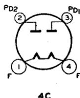
and typical operating conditions are the same as those for the Type 5U4-G. The base of the 5Z3 fits the standard four-contact socket which should be mounted to hold the tube preferably in a vertical position with the base down. Horizontal operation is permissible if pins 1 and 4 are in a horizontal plane. Physical characteristics of the 5Z3 are shown in Fig. 2-27, OUTLINES SECTION. Filament operation and ventilation are discussed under Type 5T4.
