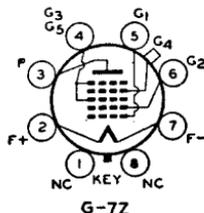
often designed to cover frequencies as high as 20 megacycles. For general discussion of pentagrid types, see Frequency Conversion in RADIO TUBE APPLICATIONS section.
