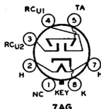
control electrodes. The tube, therefore, is a voltage indicator and as such is particularly useful as a convenient and non-mechanical means to indicate accurate tuning of a receiver to the desired station. Features of the 6AF6-G are its small size and its flexibility of application.
