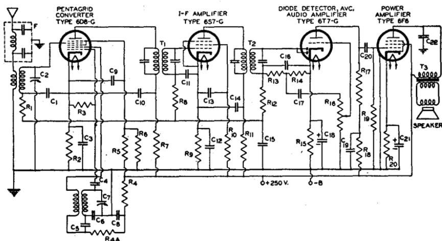
$C_1, C_{11}, C_{13}, C_{20} = 0.05 \mu\text{f}$  paper
