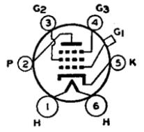
Physical characteristics of the 58 are shown in Fig. 2-20, OUTLINES SECTION. The base of the 58 fits the standard six-contact socket which may be installed to hold the tube in any position. For heater operation and cathode connection, refer to Type 2A5. For control-grid bias variation, screen voltage, and suppressor connection, refer to Type 6SK7. Shielding requirements are similar to those for Type 6C6.
