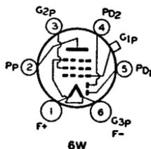
installed to hold the tube preferably in a vertical position with the base down. Horizontal operation is permissible if pins 1 and 6 are in a vertical plane. Physical characteristics of the 1F6 are shown in Fig. 2-16, OUTLINES SECTION. Filament operation of the 1F6 is discussed under Type 1C7-G.
