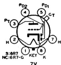
The 6R7 and 6R7-G are multi-unit tubes. Each type contains two diodes and a triode in a single envelope and is for use as combined detector, amplifier, and automatic-volume-control tube in radio receivers designed for its characteristics. For diode-detector considerations, refer to the RADIO TUBE APPLICATIONS section.
