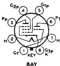
The 6AD7-G contains a voltage amplifier triode, and a power amplifier pentode similar to the 6F6-G. It is of the heater-cathode type. The 6AD7-G is especially useful in combination with a separate 6F6-G in a push-pull amplifier; in this service, the triode unit serves as the phase inverter. Curves shown under the 6F6-G apply to the pentode unit of the 6AD7-G. Physical characteristics are shown in Fig. 2-21, OUTLINES SECTION. The tube may be mounted in any position.
