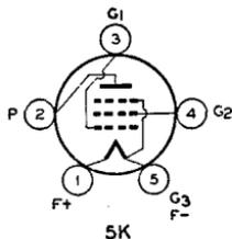
preferably in a vertical position with the base down. Horizontal operation is permissible if pins 1 and 5 are in a vertical plane. Physical characteristics of the 1F4 are shown in Fig. 2-25, OUTLINES SECTION. Filament operation is discussed under Type 1C7-G. Application is the same as for Type 1F5-G.
