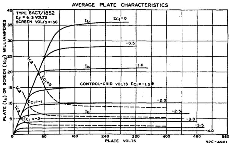
As an amplifier, the 6AC7 is especially suited for use in the r-f and i-f stages of the picture amplifier of television receivers and may also be used in the first video stages when several such stages are used. The use of the 6AC7 as a high-gain audio amplifier is not recommended unless the heater is operated from a battery source. Additional information on application of the 6AC7 is the same as shown for Type 6AB7.
