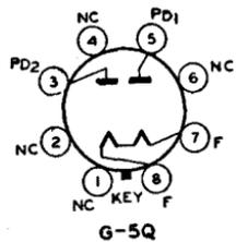
are the same as those for Type 5U4-G. The base of the 5X4-G fits the standard octal socket which should be mounted to hold the tube preferably in a vertical position. Horizontal operation is permissible if pins 2 and 7 are in a horizontal plane. Physical characteristics of the 5X4-G are shown in Fig. 2-26, OUTLINES SECTION.
