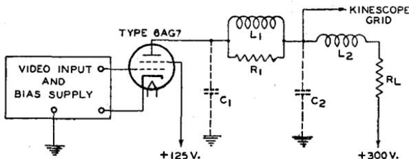
$C_1 = 9.5 \mu\text{f} = \text{Tube Capacitance} + \text{Socket Capacitance} + \text{Wiring Capacitance} + \text{Coil Capacitance}$
