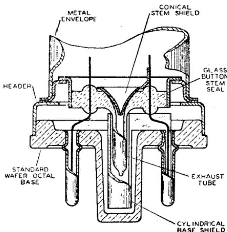
grounding pin (pin No. 1). The cylindrical base shield is positioned inside the locating base plug, and is also connected to pin No. 1. The conical shield reduces the capacitance between leads in the glass of the stem: the cylindrical shield reduces the capacitance between those pins that are diametrically opposite each other. Since the grid and the plate leads are diametrically opposite, the capacitance between them is kept to a value comparable with that obtainable with top-cap construction.
