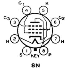
For heater operation and cathode connection, refer to Types 12A8-GT and 6A8, respectively.
