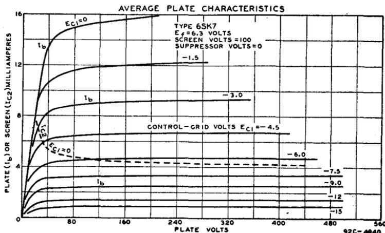
Therefore, the ability of the tube to handle large signals is somewhat impaired. This effect may be nullified by means of a series resistor in the screen circuit.
