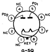
socket which should be mounted to hold the tube preferably in a vertical position. Horizontal operation is permissible if pins 2 and 7 are in a horizontal plane. Physical characteristics of the 5Y4-G are shown in Fig. 2-21, OUTLINES SECTION. Filament operation and ventilation are the same as for Type 5T4.
