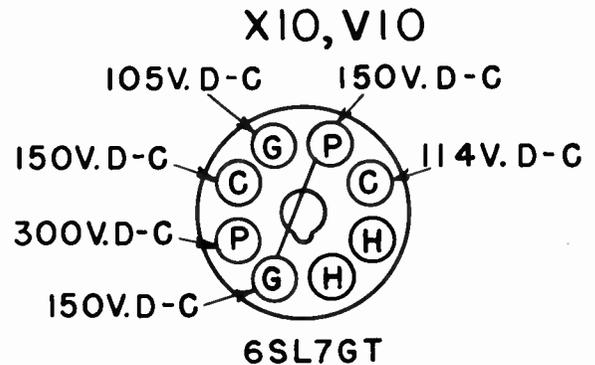
Figure 10—Type 580-D Regulated Power Supply, Typical Tube Socket Voltages
