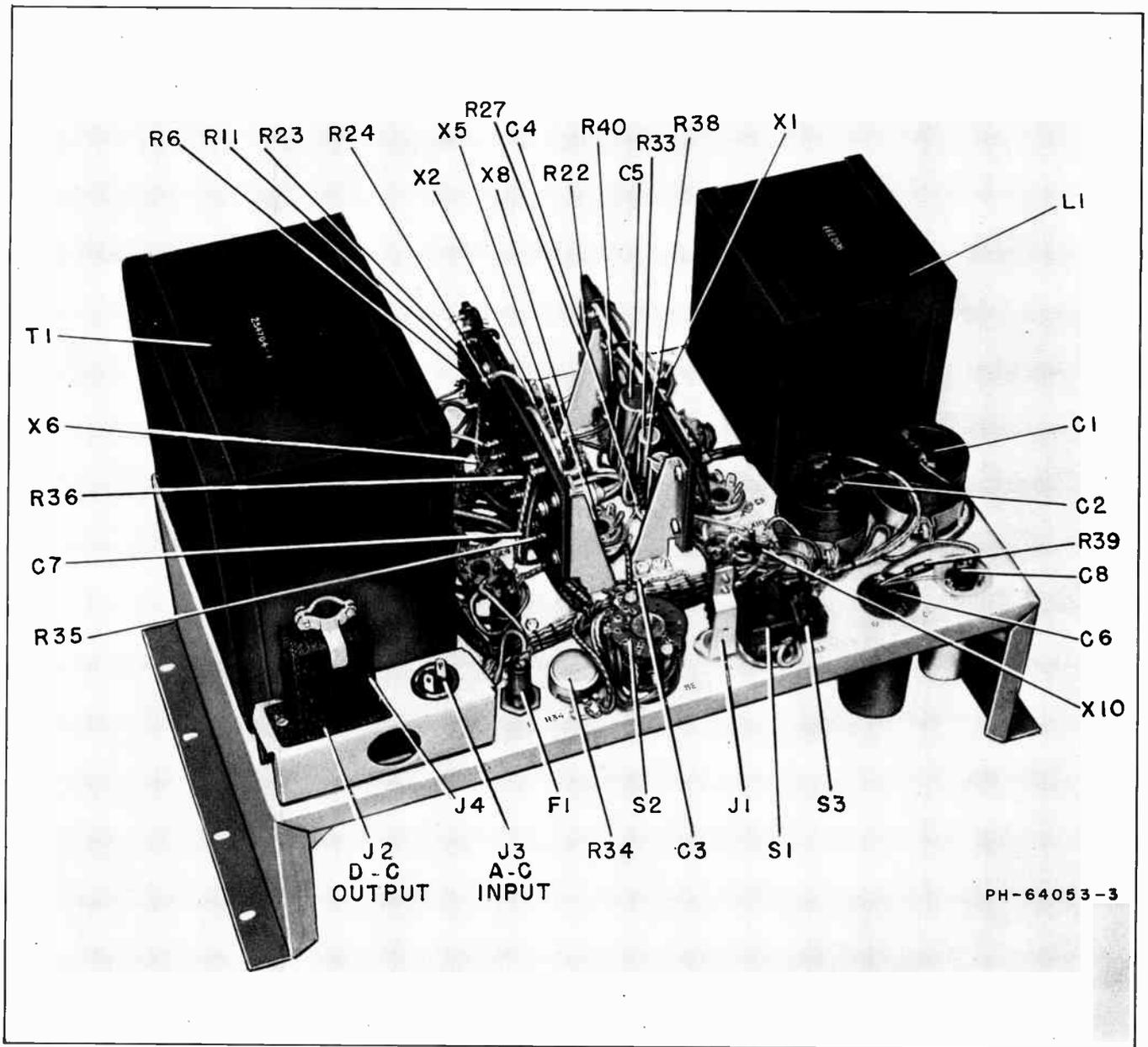
Figure 7—Type 580-D Regulated Power Supply,
