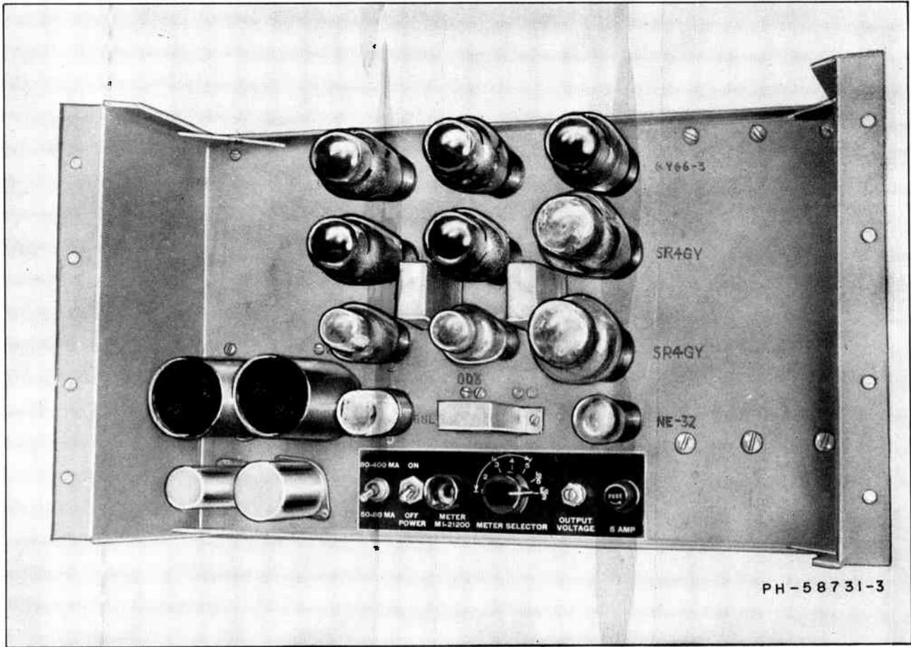
Figure 1—Type 580-D Regulated Power Supply, Front View
