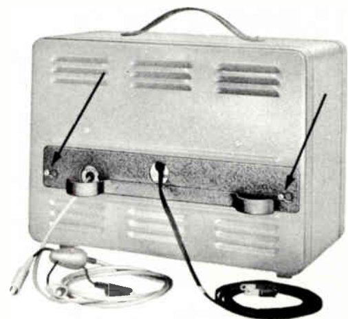
Figure 1. Rear View of WR-51A Showing Cable-Holding Bracket
