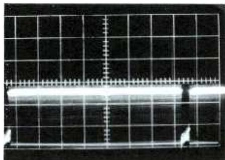
Blanking at Kinescope Grid #1
