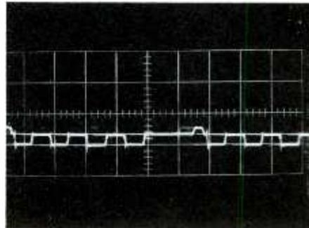
Blue Signal at Kinescope Pin #13
