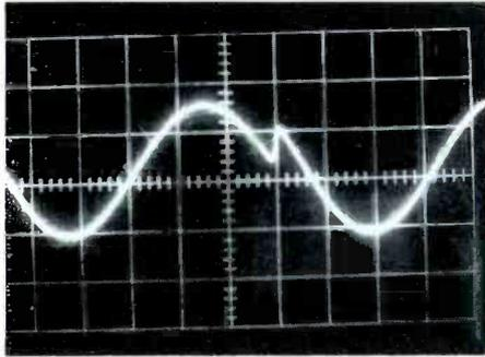
Ringing Coil Voltage at Pin 8 of 5V3
