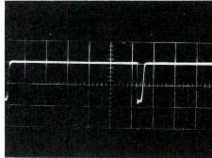
Clamp Pulse at Pin 1 of 4V3
