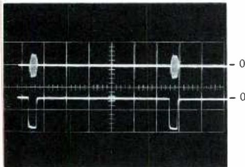
Top Trace: Demodulated Burst at Emitter of 2Q7
