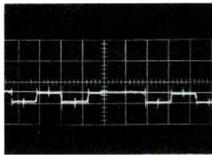
Red Signal at Kinescope Pin #4
