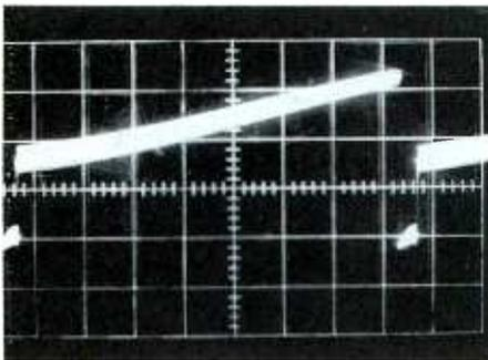
Vertical Sawtooth at Pin 1 of 5V1
