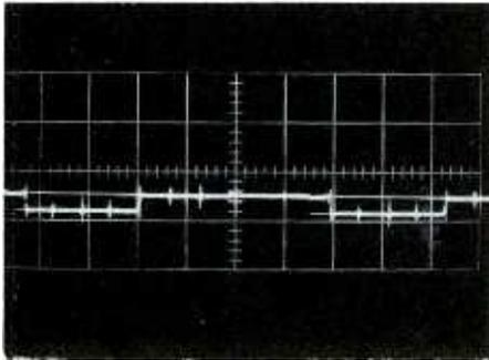
Green Signal at Kinescope Pin #5
