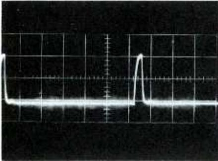
Clamp Pulse at Pin 6 of 4V3
