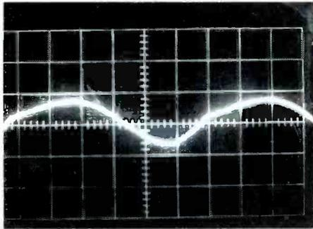
Damper Plate, Pin 2 of 5V7
