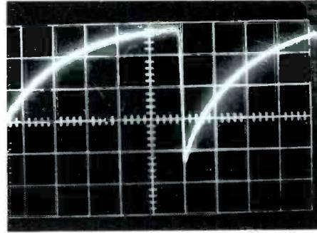
Grid Drive at Pin 5 of 5V4
