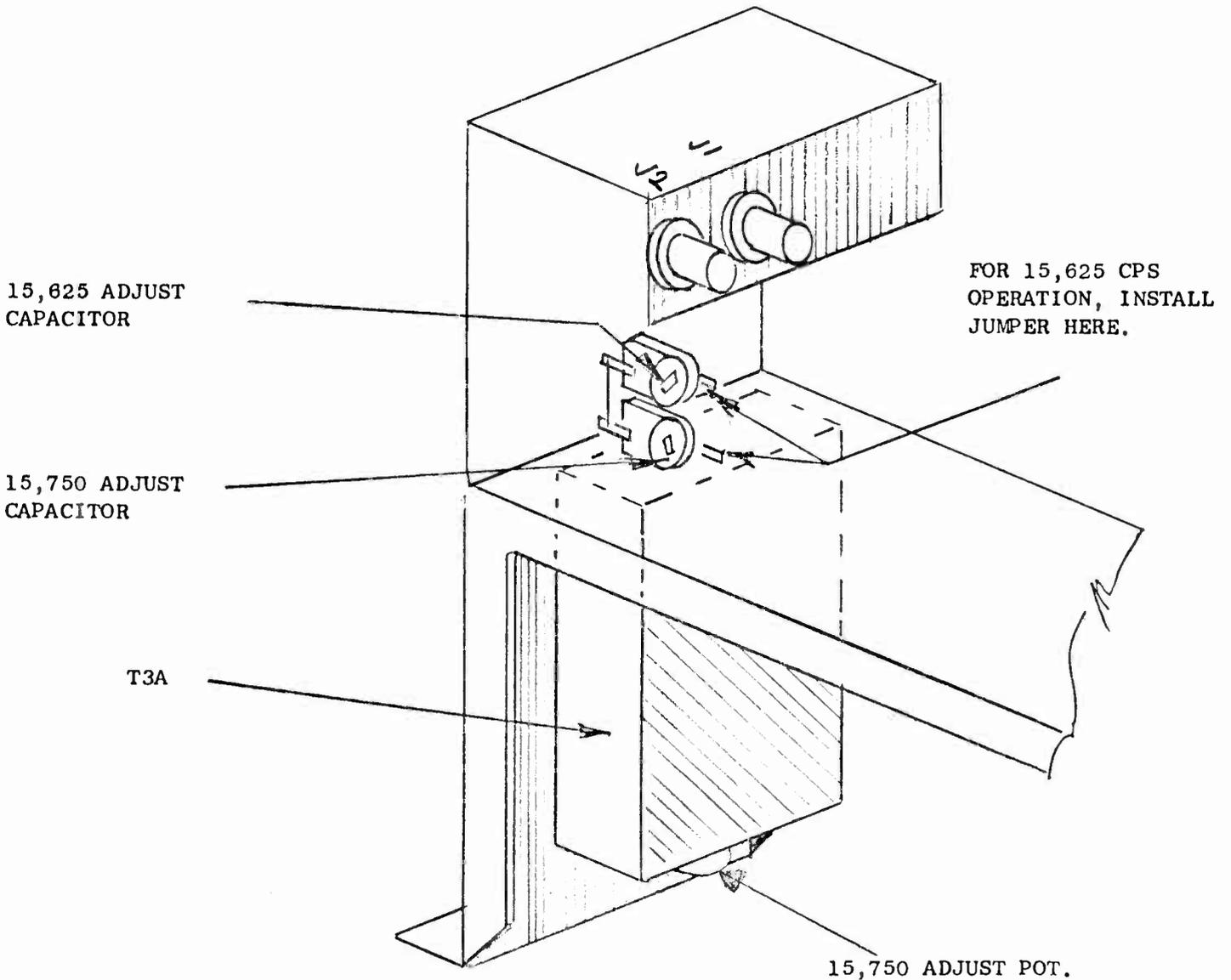
TSD-2B & TSD-3A MICROWAVE SOUND DIPLEXER DEMODULATOR 15,750 CPS/15,625 CPS FILTER ADJUSTMENT LOCATIONS.
