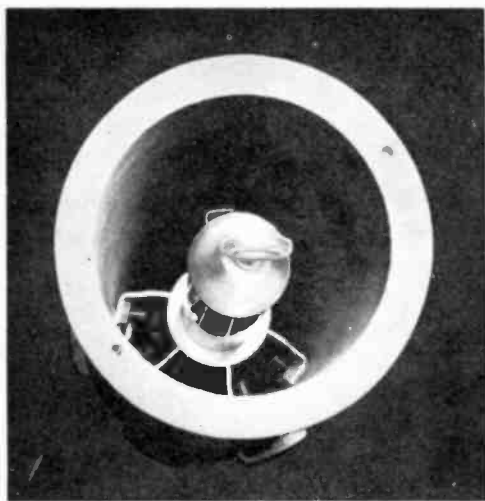
FIG. 2. Top View of TFU-24-BH Antenna with Beacon Mount Removed Showing Spoke Type Shorting Plug and Transmission Line. Harness is moved by use of Ring for Electrical Pattern Tilt Adjustment.
