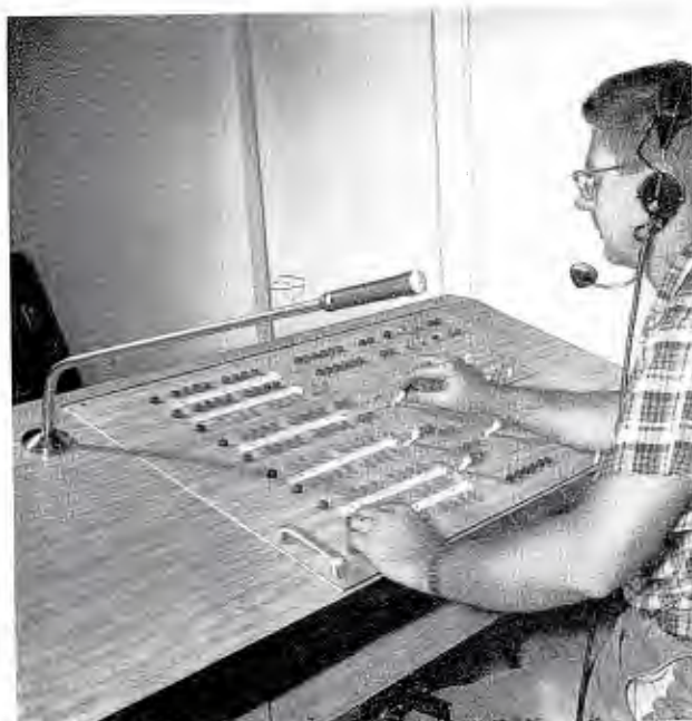
View of custom switching console in mobile unit.
