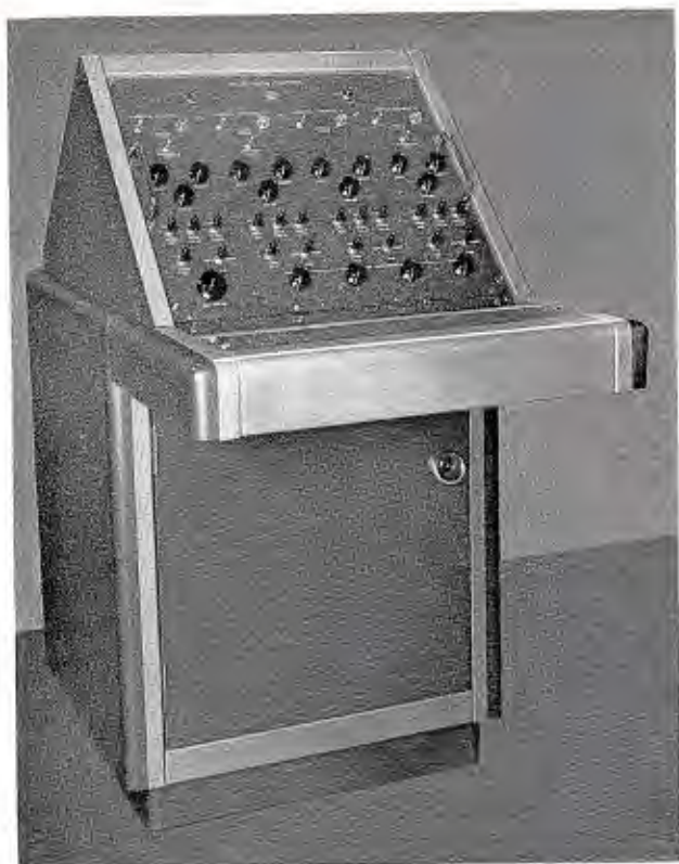
Custom control panel and console as built by RCA for a closed circuit television installation.
