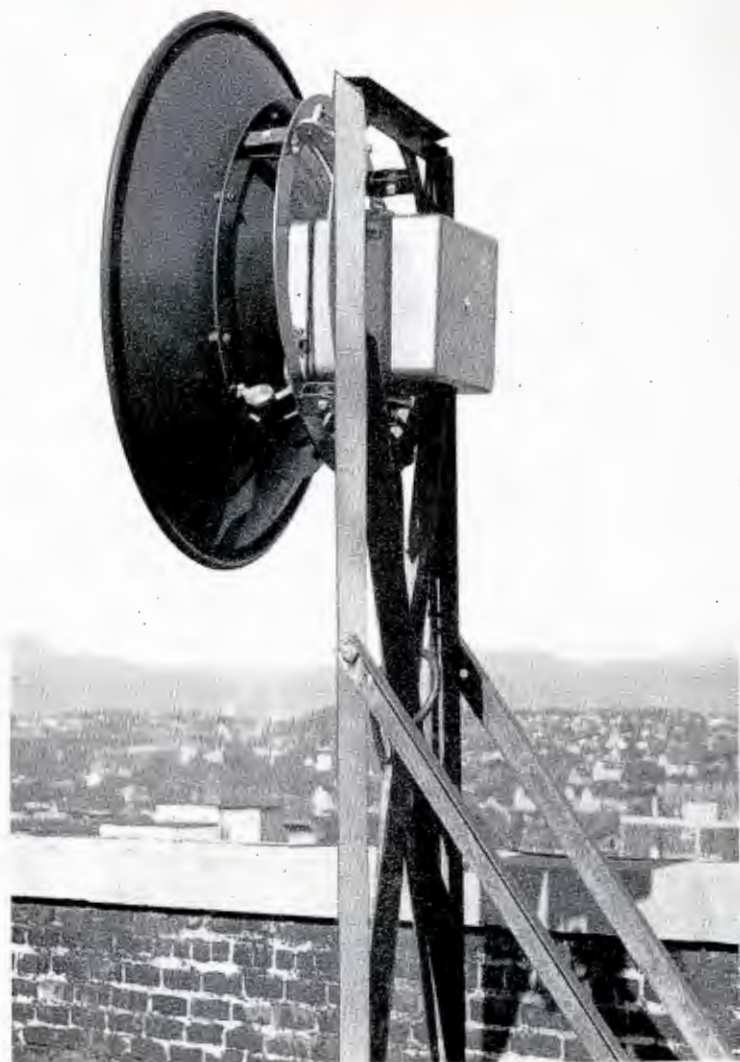
Relay Antenna Gimbal Ring Mount, MI-26207, mounted to bosses of 4 foot parabolic antenna and fixed service support allows horizontal or vertical adjustment of the antenna. View also shows TVM-1A Relay Transmitter Head, MI-26450, attached to parabola by means of Reflector Mount, MI-26435-A.
