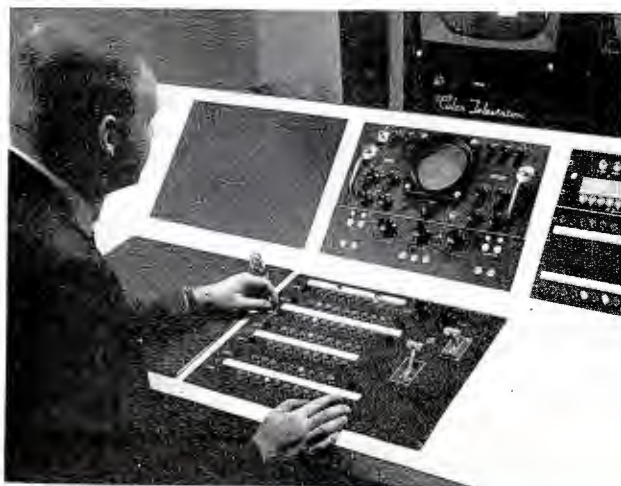
View of the television tape switching control panel at master control in Reeves Sound Studios. The inputs to six RCA Tape Machines are all switchable at this central location.
