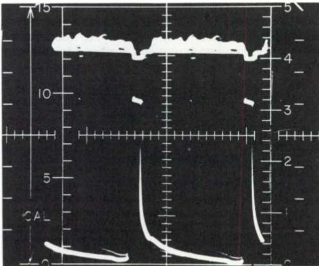
Figure 7-6 Sync Separator With Waveforms at Base (Top) and Collector. Horizontal Rate, Double Exposure, Scope Gain Constant for Both Waveforms
