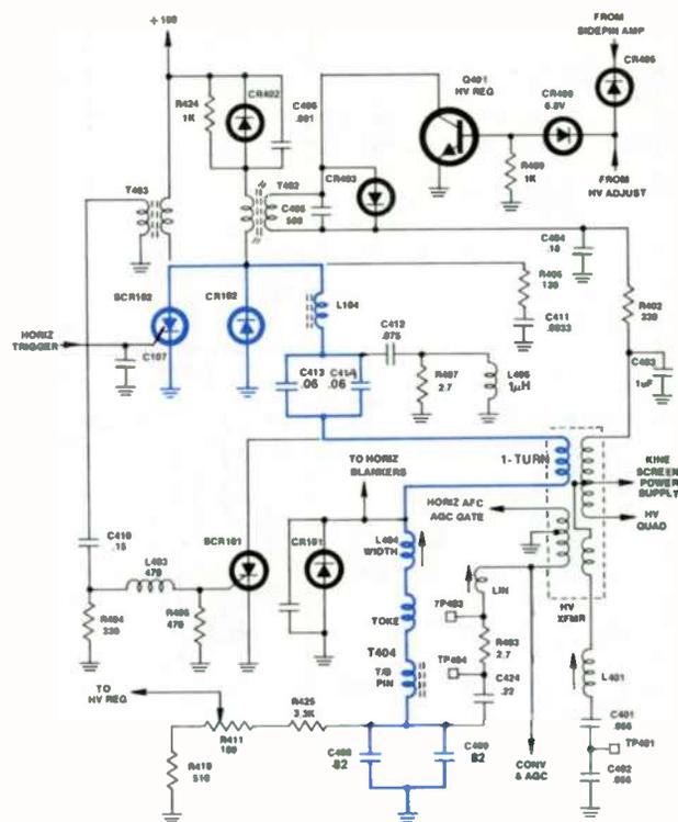
Figure 4-3B Retrace Resonant Circuit
