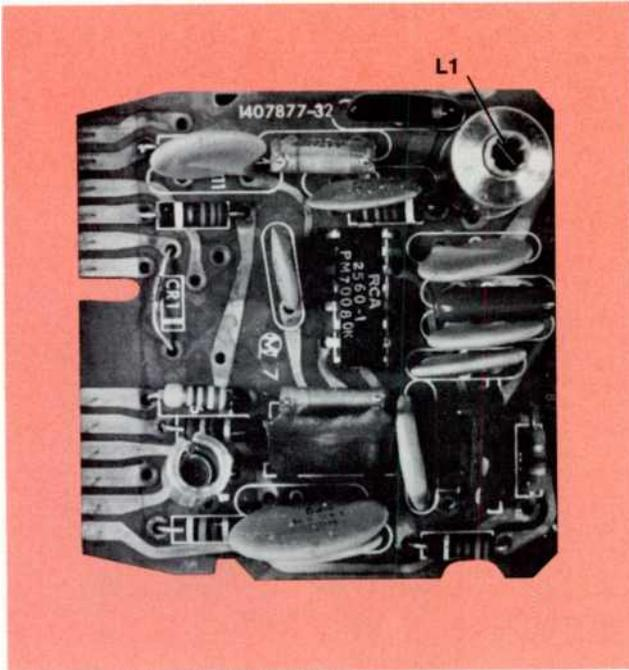
Module MAE (Chroma-2 module) contains the chroma demodulators and color-difference amplifier, and accommodates the tint control. L1 may be adjusted in the field to center tint-control range.
