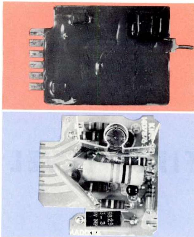
Two different types of MAD modules may be used in the RCA CTC 49 chassis. The ceramic module (top) and the module using discrete components (bottom) are interchangeable, requiring only readjustment of the kine drive control for tracking.
