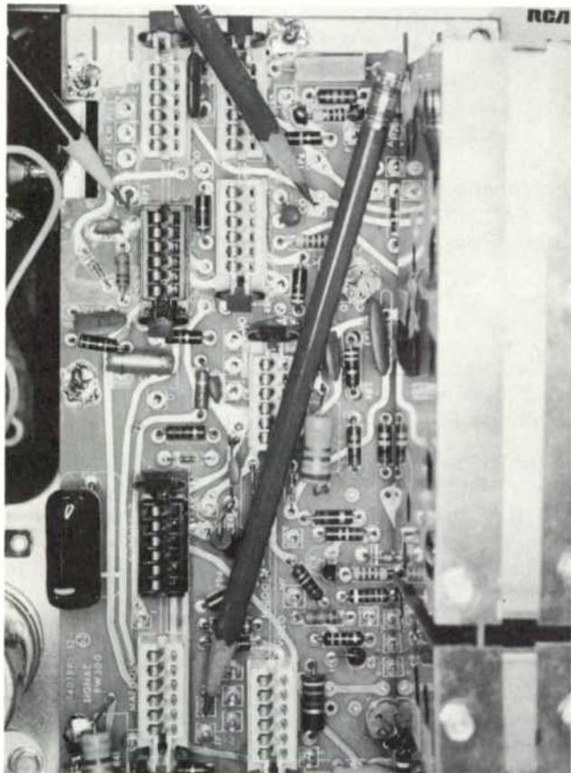
The locations of TP 305, stake CO (top, left and right), and stake AF (bottom) are indicated by the three pencils. CO is used to monitor the chrominance-video output from the Module MAK. TP 5 is the observation point for the burst-blanking pulse, and stake AF is the regulated 11-volt test point.
