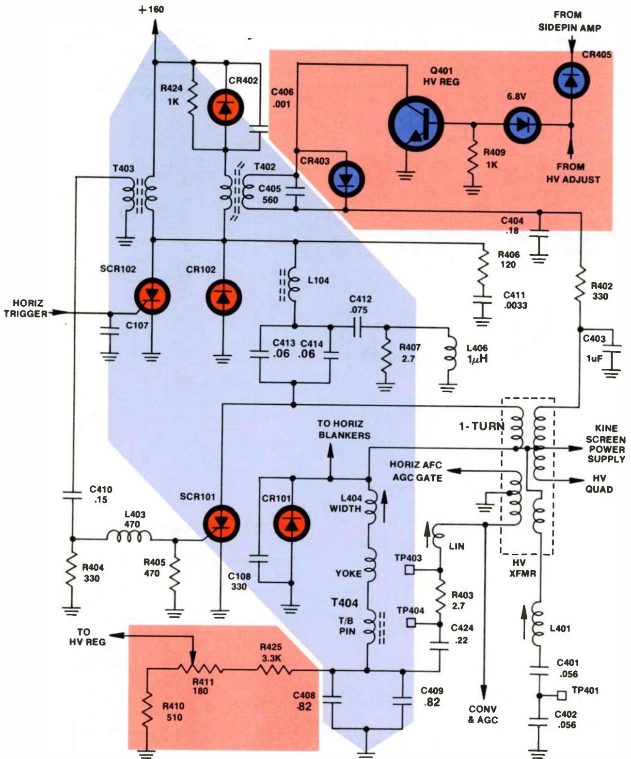
Figure 4-3 Horizontal Deflection and High-Voltage Regulation Circuits
