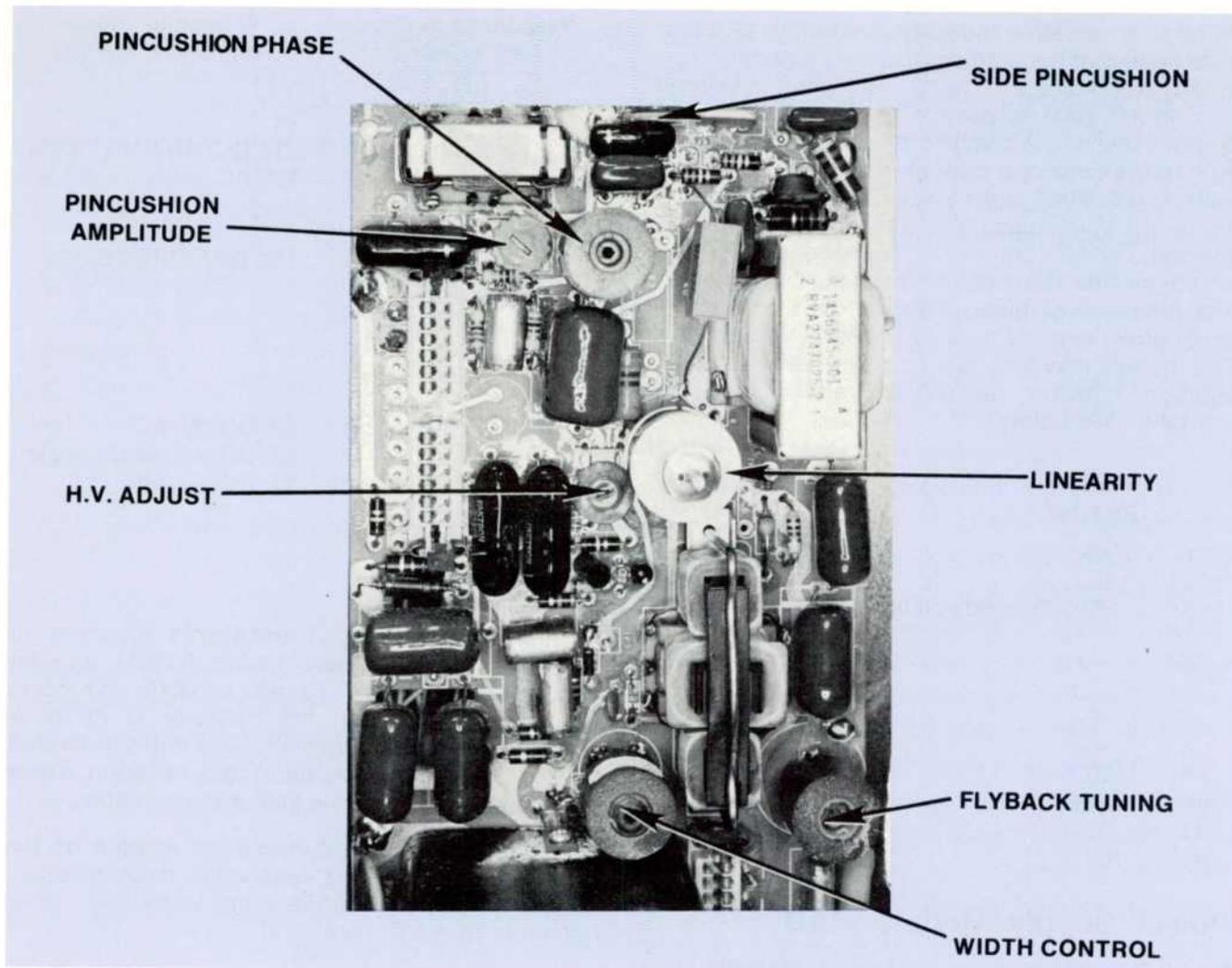
*The linearity, pincushion, high voltage, and width adjustments are located in this view of PW 400.*
