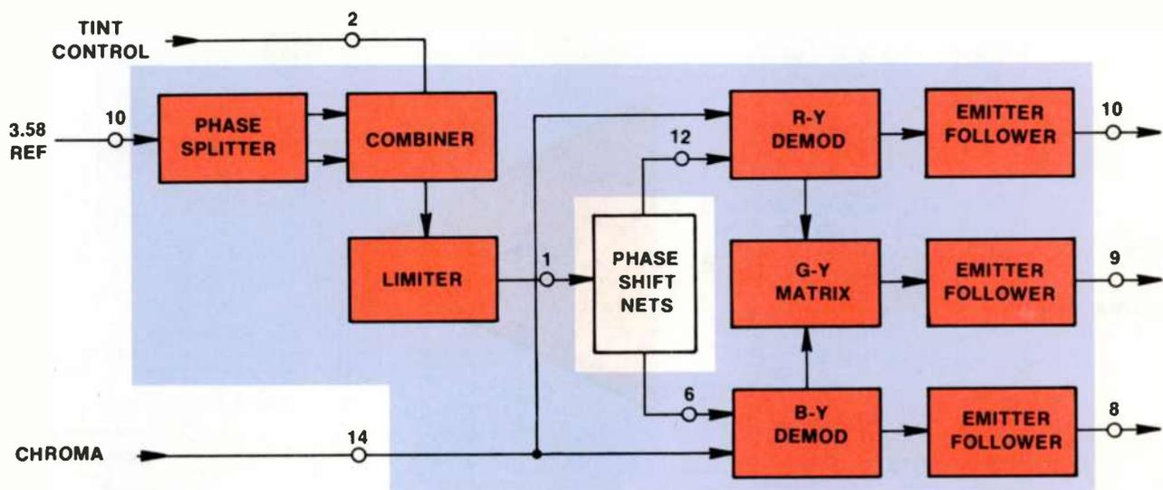
Figure 3-5 Functional Diagram of Chroma-Demodulator IC
