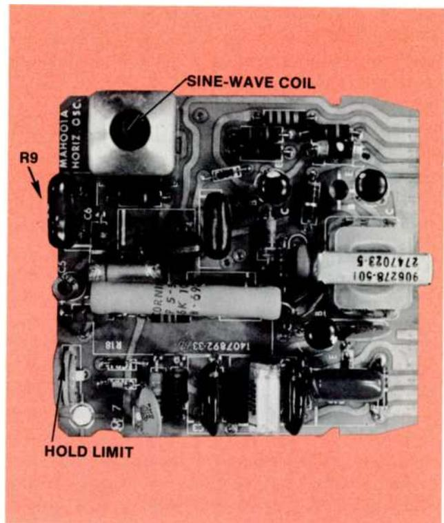
MAH is the horizontal oscillator and AFC module. The hold-limit and sine-wave coil adjustments are indicated, R9 parallels C6 and is located behind it.
