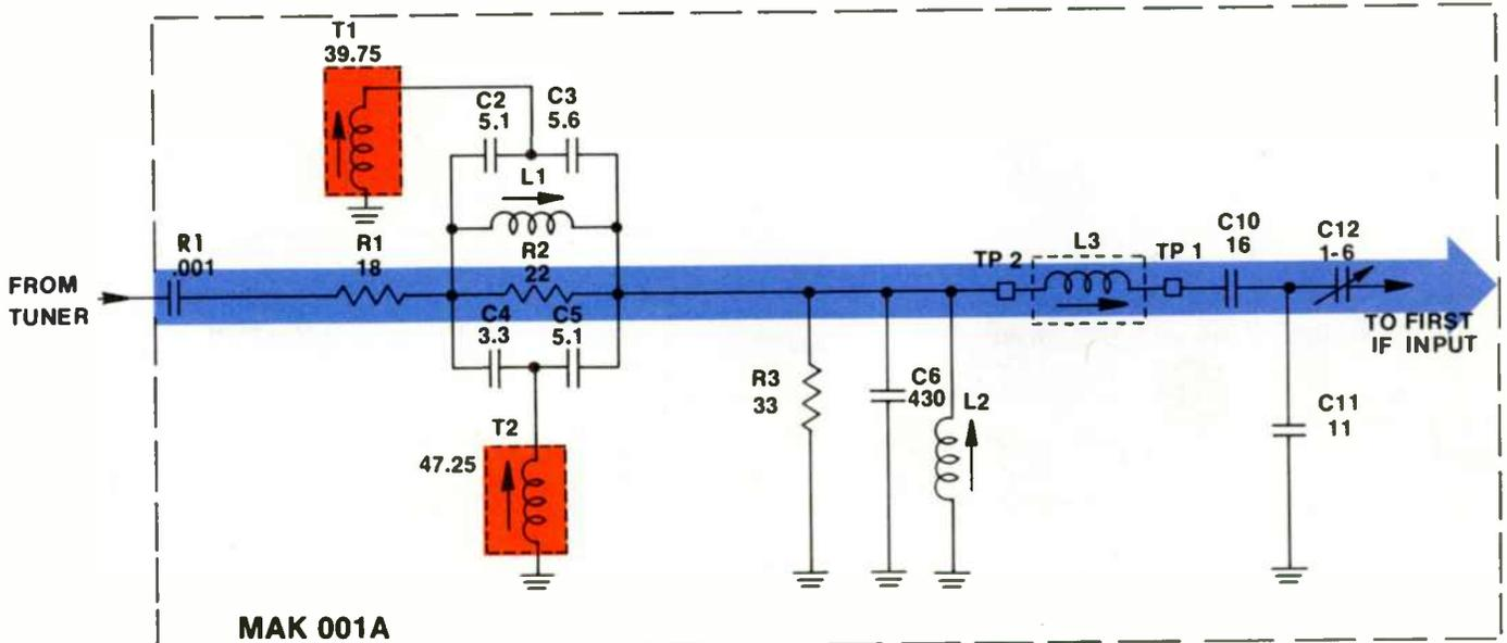
Figure 2-4 Traps and IF Input Tuned Circuits
