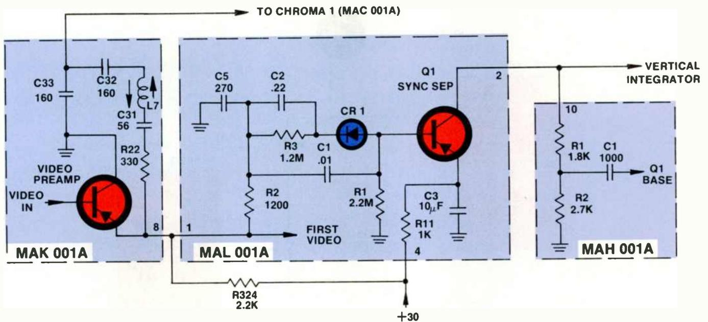
Figure 3-7 Sync Separator and Sync Distribution
