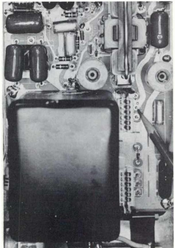
If the receiver is operated with Module MAH removed, there will be no bleeder for the 160-volt power supply. To discharge this supply after the receiver is turned off, ground stake X of PW 400.
