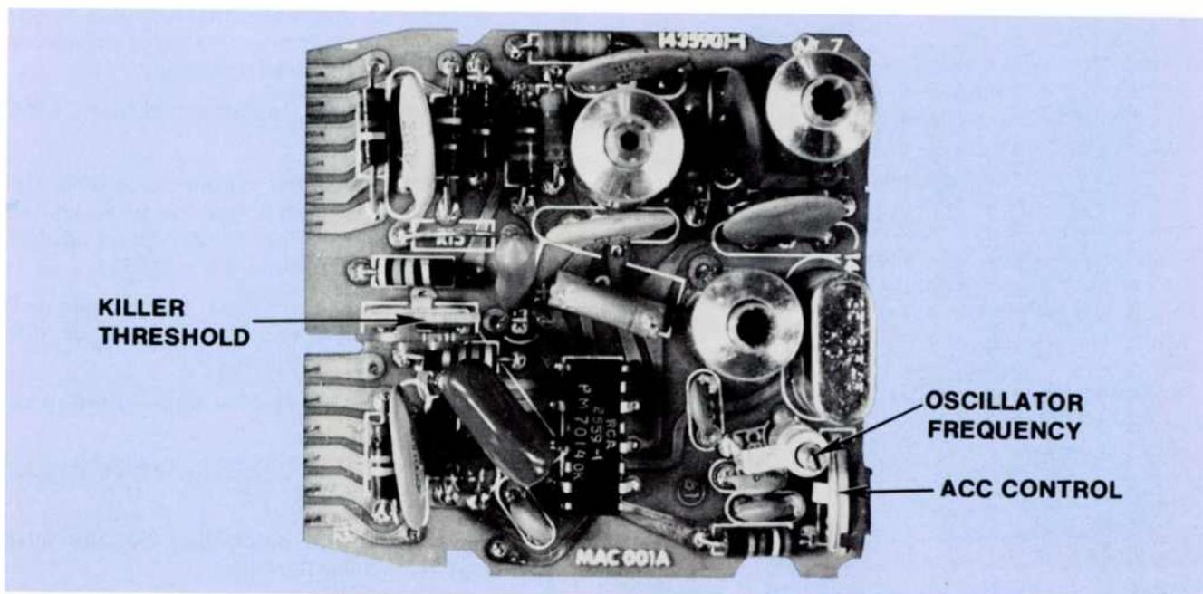
*Module MAC (Chroma-I module) functions as a bandpass amplifier and 3.58-MHz reference oscillator. It also has the ACC and color-killer circuits.*
