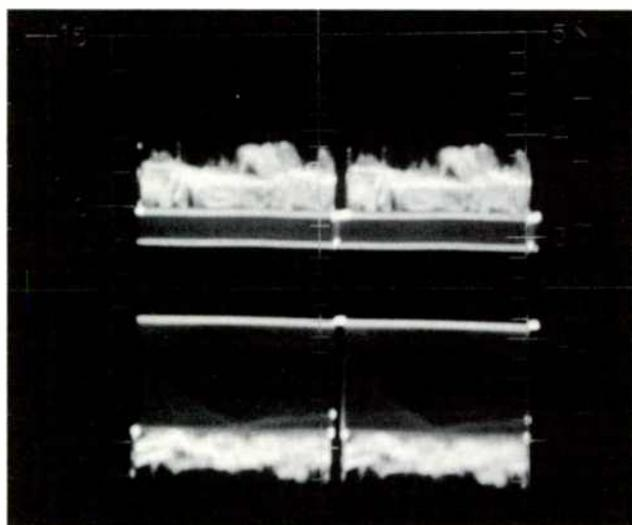
Base (Top) and Collector Waveforms of First Video Amplifier at Vertical Rate and Constant Scope Gain
