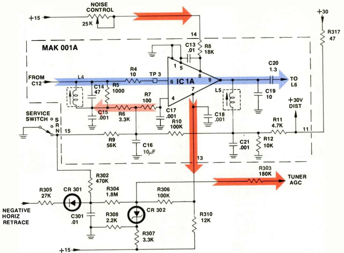
Figure 7-2 First and Second IF Amplifiers and AGC Circuit
