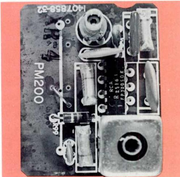
Sound module PM 200. The edge connections are on the rear. The input transformer is at the top.
