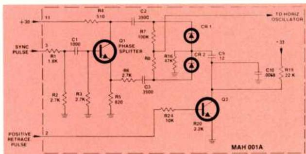
Figure 7-9 Horizontal AFC Circuit
