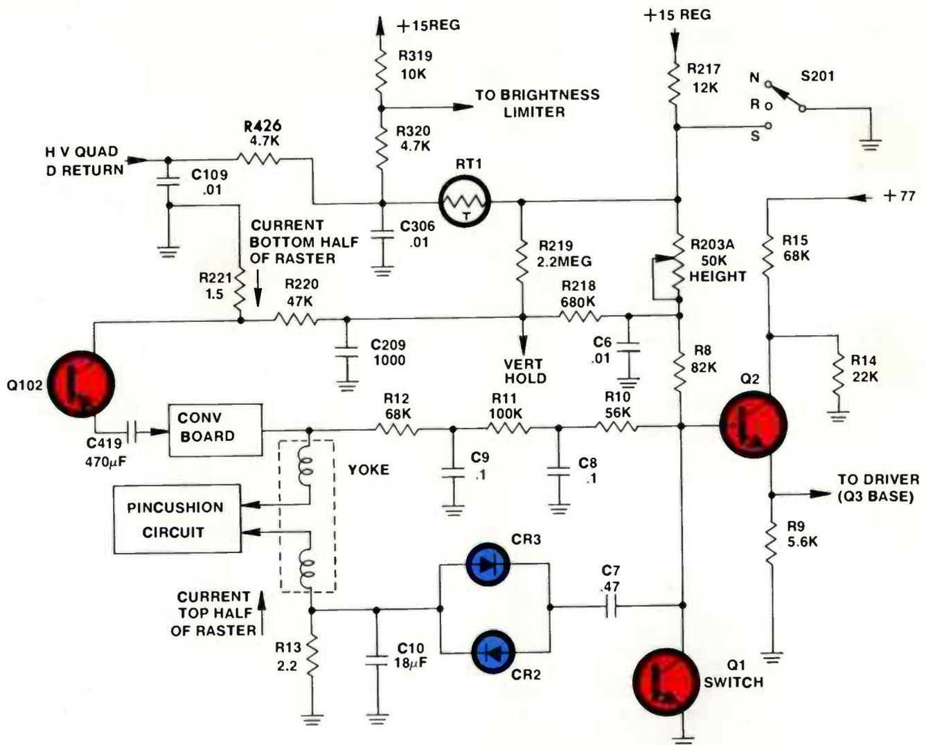
Figure 5-4 The Vertical Predriver With Its Inputs
