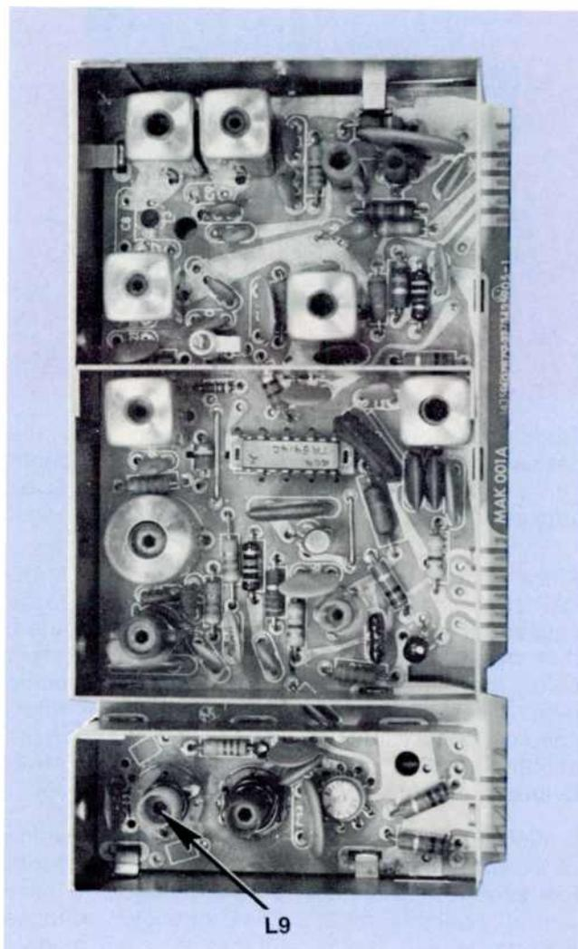
Module MAK (IF/AFT module) with the top shield off. L9 is also accessible from the opposite side.
