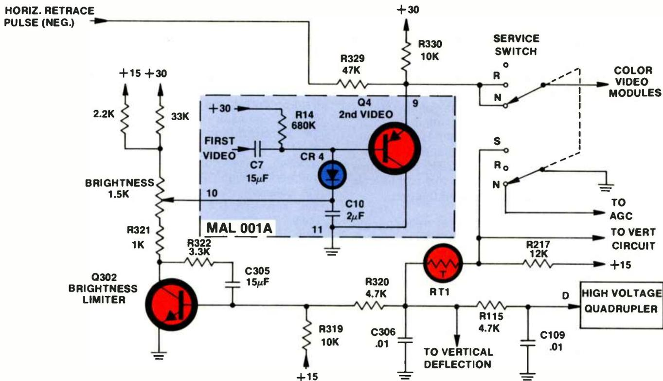
Figure 3-10 Second Video Amplifier and Brightness Limiter
