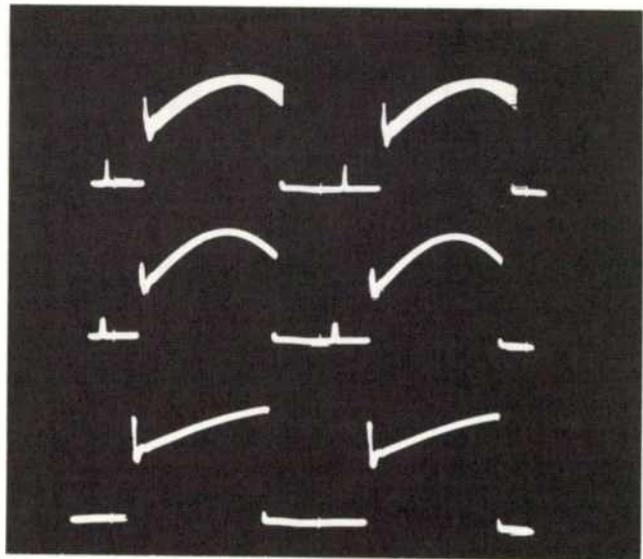
*Waveform At Anode of CR 102. Top Is Normal, 320 Volts P-P. Center Caused by Shorted Q401 or Open Q402; Bottom by Open Q401 or Shorted Q402.*
