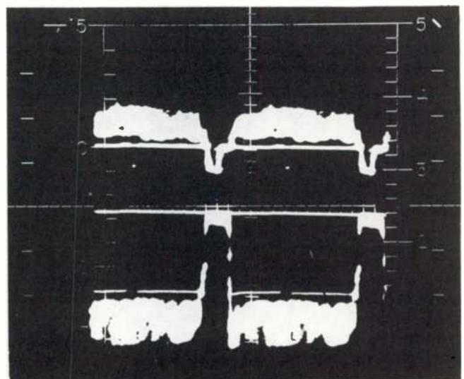
Base (Top) and Collector Waveforms of First Video Amplifier. Same Photo Conditions As in Figure 7-6
