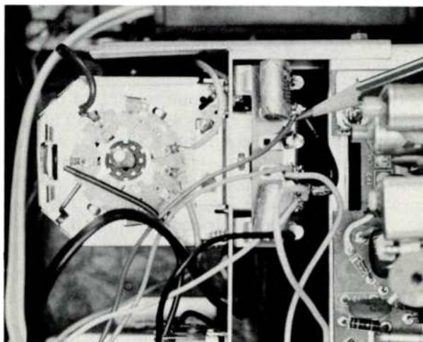
Rear view of the KRK 165C tuner. The test point for tuner AGC voltage is indicated by the pencil.
