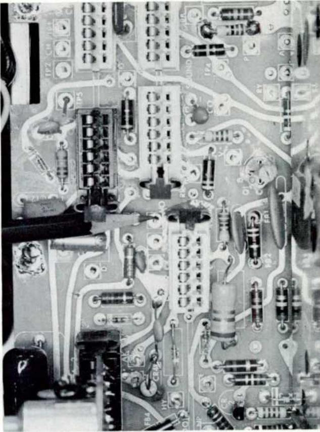
*The luminance video output from Module MAK appears at stake VO of PW 300. When they are inserted, Module MAL is to the right of this test point and the sound Module, PM 200, is above it.*
