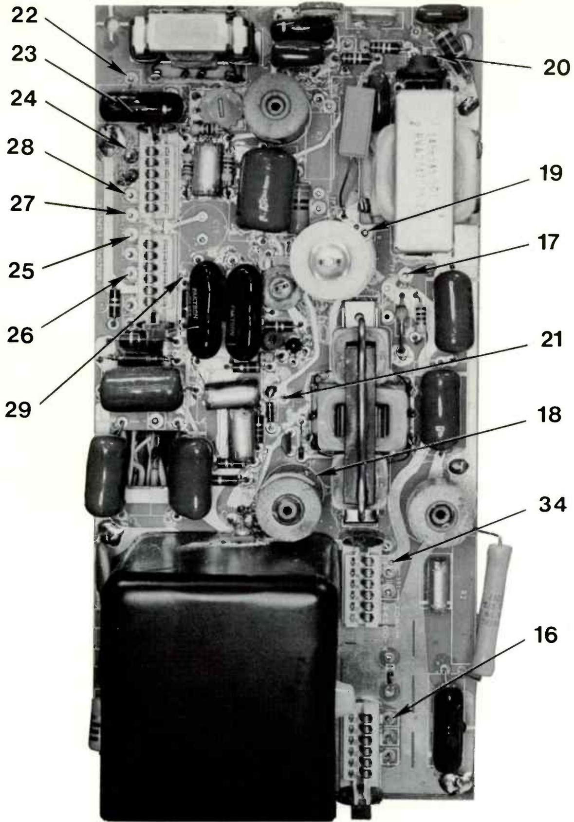
*Test-Point Location for Schamtic Diagram, PW 400*
