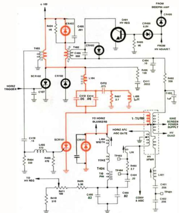
Figure 4-3C Power-Input Resonant Circuit
