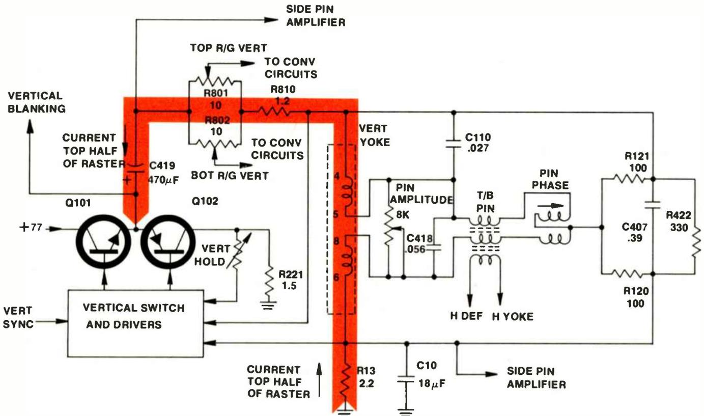
Figure 5-3 Yoke Circuit of the RCA CTC 49
