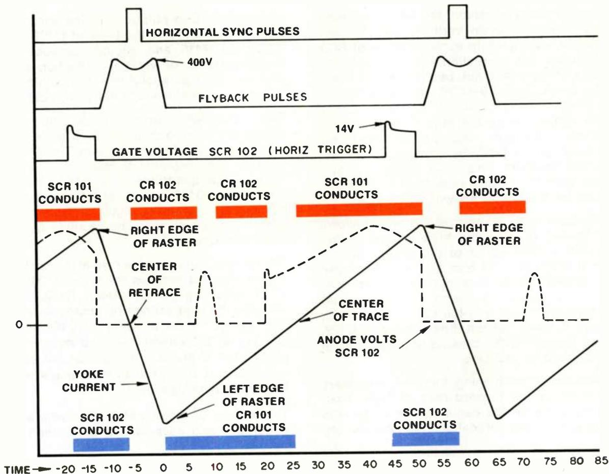
Figure 4-4 Timing Diagram of Horizontal Deflection System
