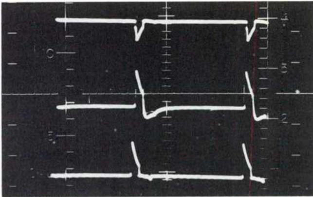
Waveforms of MAH-Q1—Collector, Base Emitter (Top to Bottom). Base Voltage Is 1.8 Volt, P-P.
