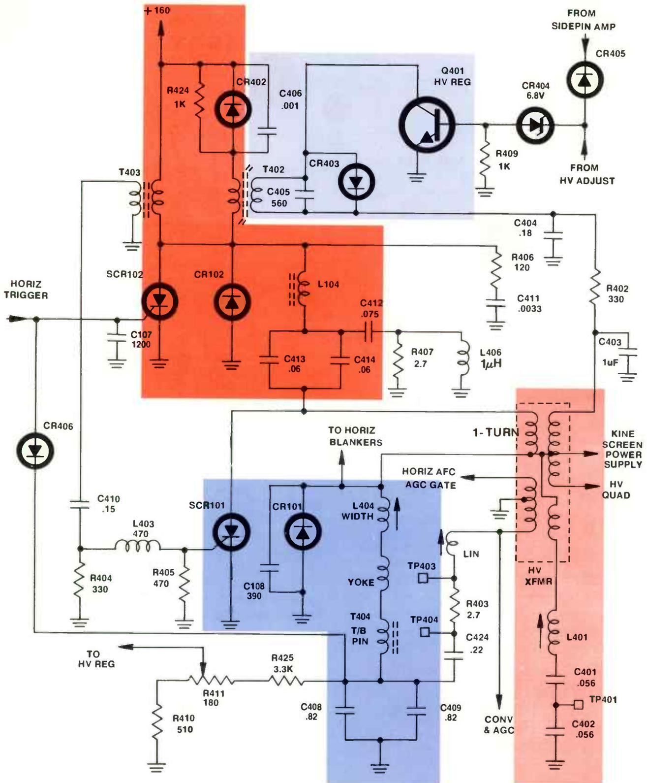
Figure 7-11 Horizontal Deflection Circuit and High-Voltage Regulator
