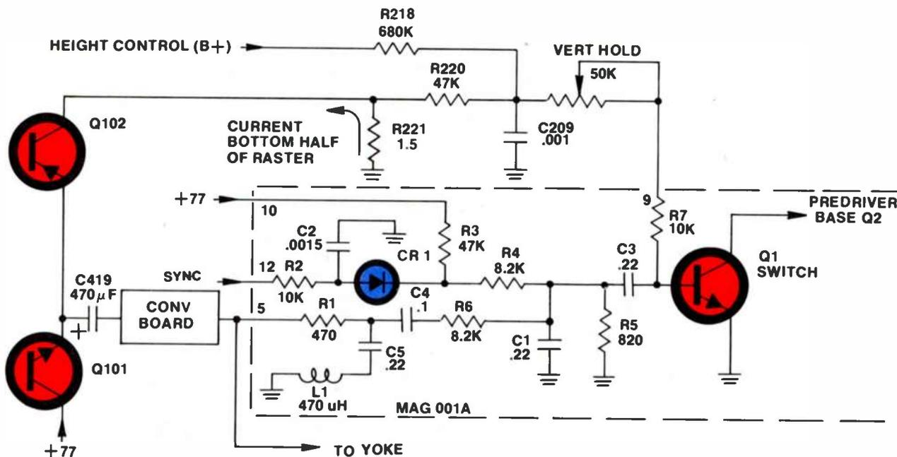
Figure 5-5 Vertical Switch Circuit
