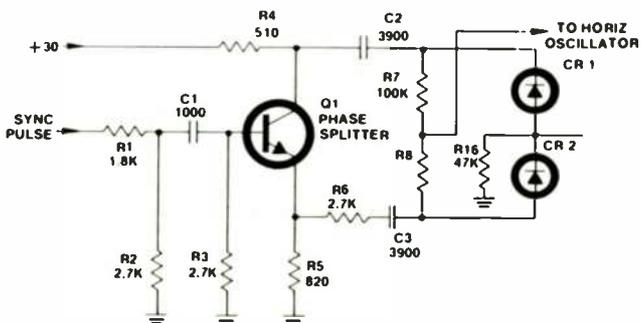
Figure 7-1 Horizontal AFC Circuit
