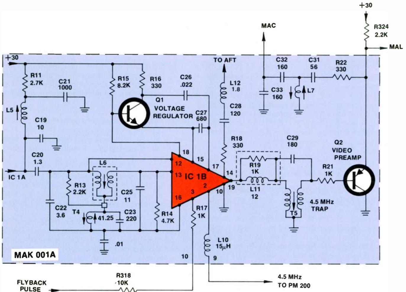
Figure 2-6 IF Output and Video Preamplifier
