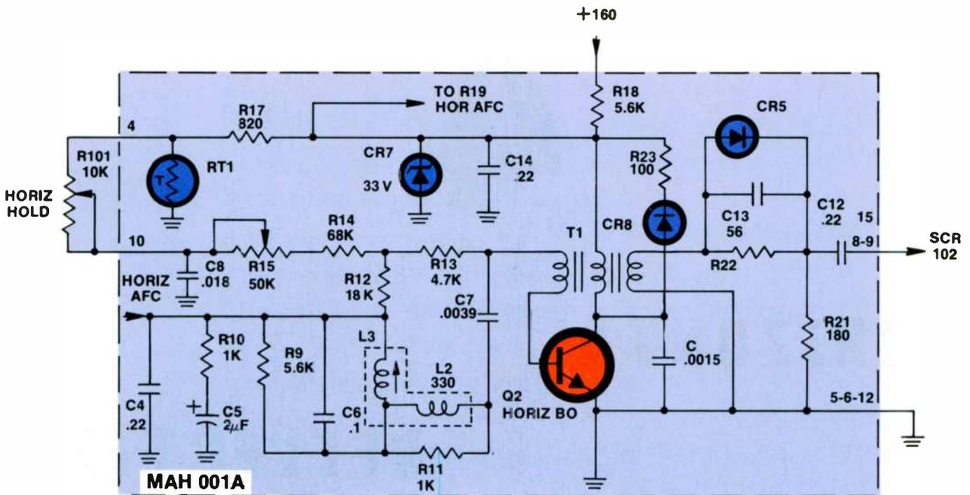
Figure 4-2 The Horizontal Oscillator
