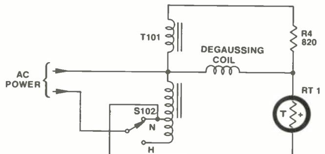
Figure 1-2 Simplified Degaussing Circuit
