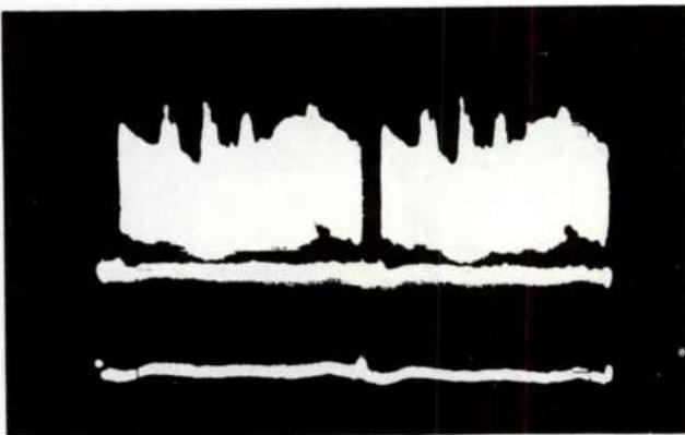
Composite Video at Tuner Output—Vertical Rate
