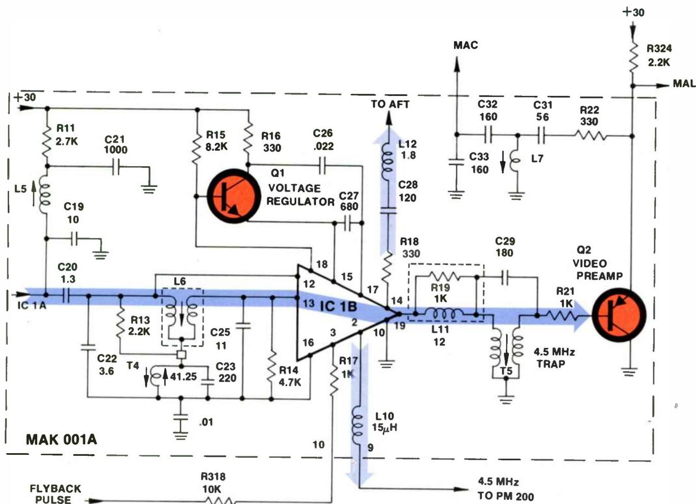
Figure 7-3 Final IF Amplifier, Video Preamp, and Voltage Regulator
