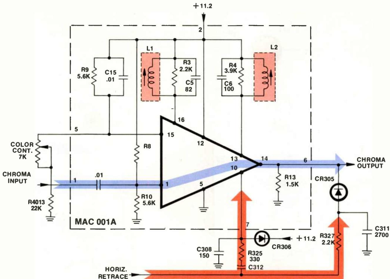
Figure 7-4 Bandpass Amplifier Circuits of Module MAC
