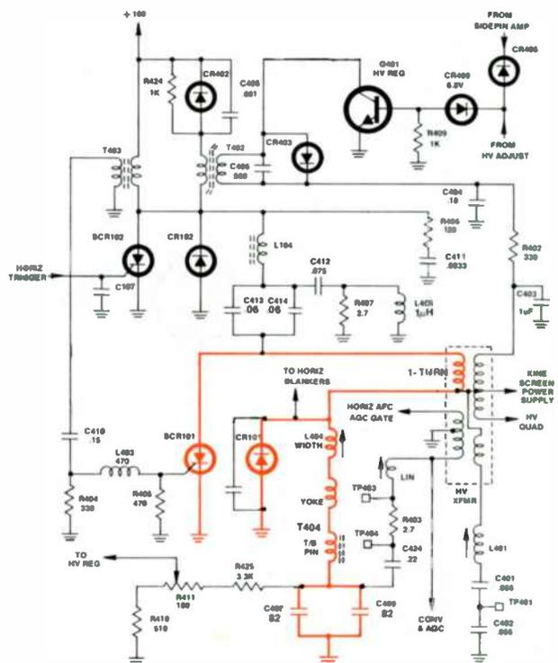
Figure 4-3A Trace Resonant Circuit
