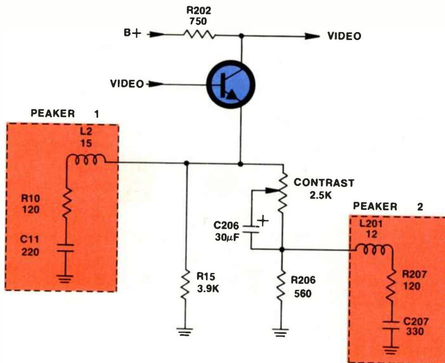
Figure 3-9 Simplified Peaking Circuits
