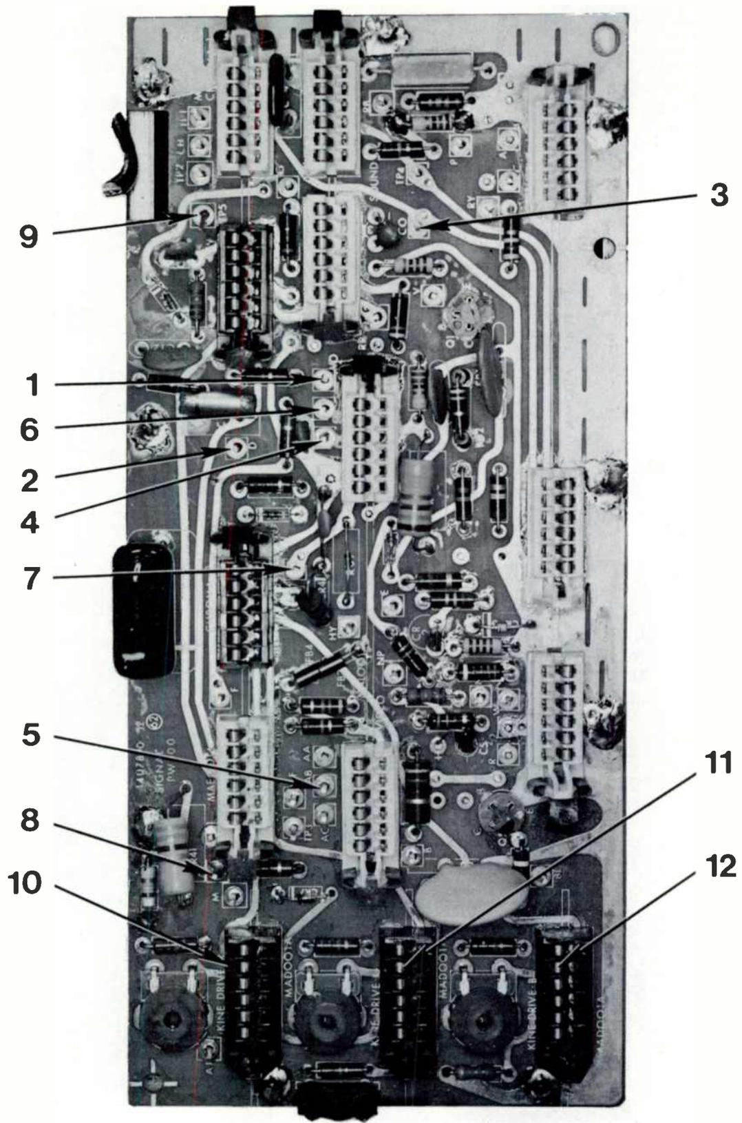
*Test-Point Location for Schematic Diagram, PW 300.*
