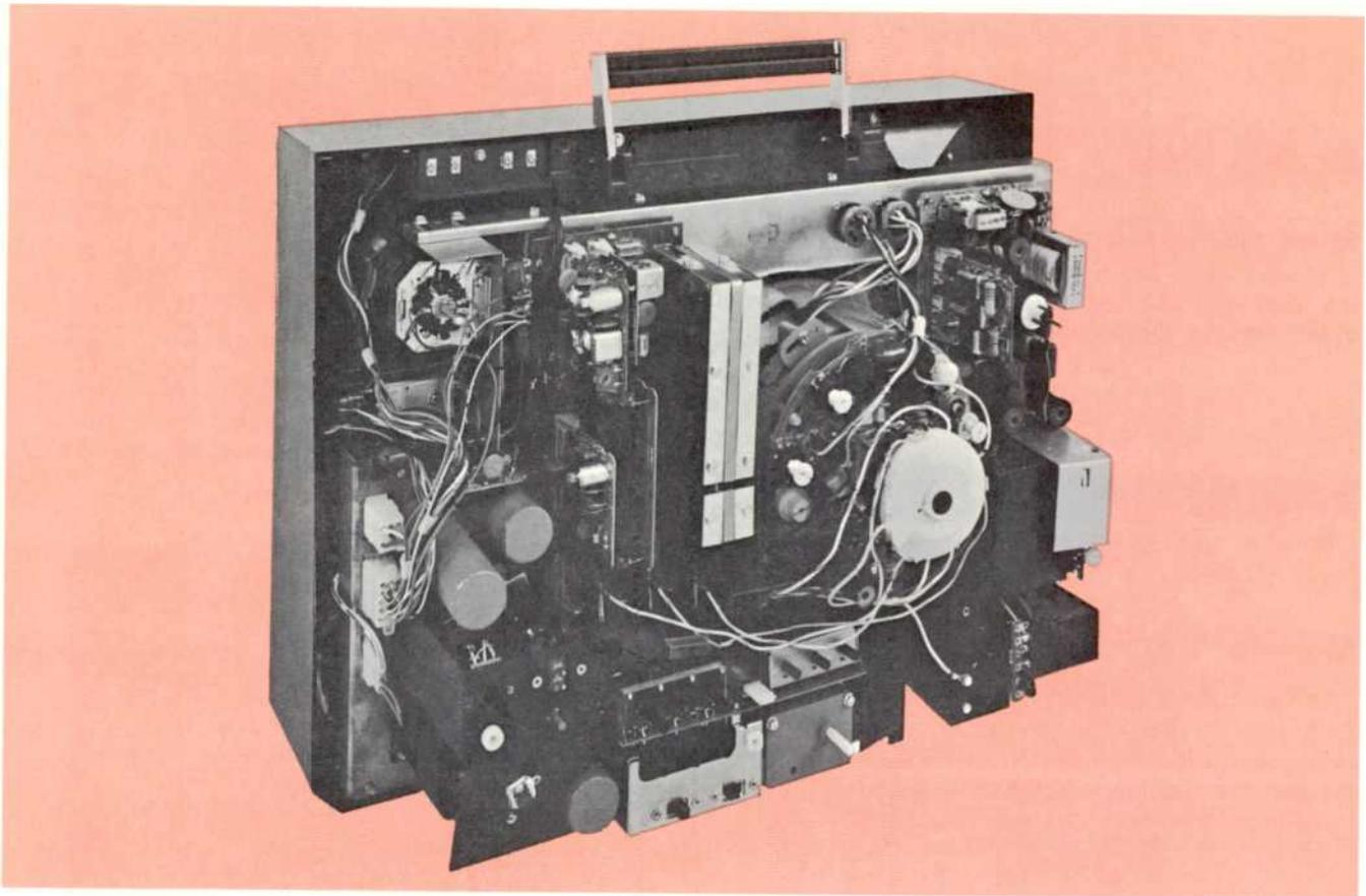
The main chassis mounts the power transformer, power-supply filters, the audio-output transistor, two vertical-output transistors, high-voltage quadrupler and focus bleeder, and the SCR's and diodes of the horizontal-deflection system. The power supply utilizes a transformer; however, one side of the AC line is connected to the chassis. The DC outputs and their principal uses are as follows:
