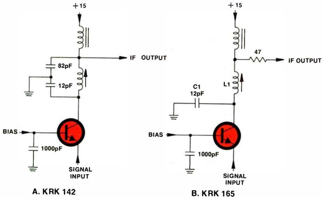
Figure 2-2 Mixer Output Circuit of the KRK 142 and KRK 165 Tuners
