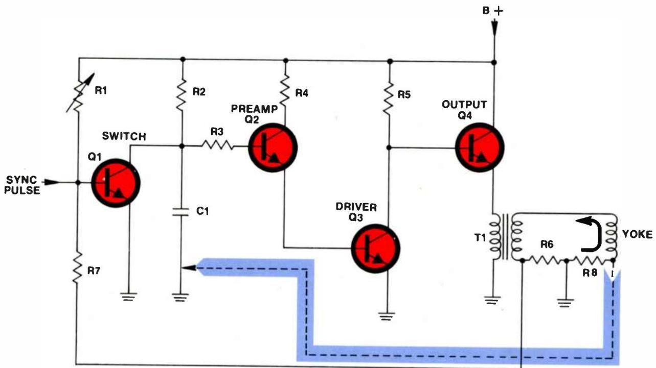
Figure 5-1 Simplified Vertical Deflection Circuit
