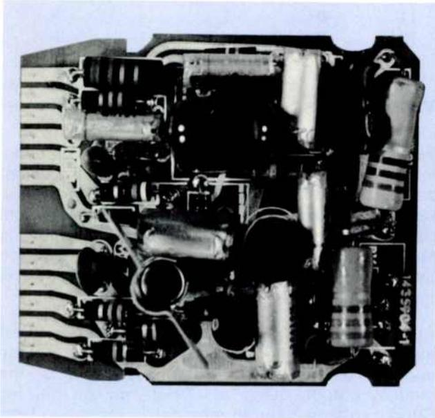
Module MAG. The vertical switching transistor is located near the lower edge below the predriver and the vertical driver is identified by its heat sink.
