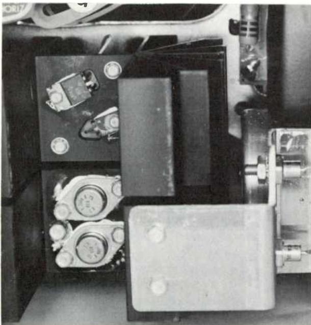
*This photo of the rear of the chassis shows the location of the deflection output devices. At the left from top to bottom are Q101, and Q102 (vertical output), then SCR 102 and SCR 101 (horizontal output). To the right are CR 102 (top) and CR 101 (bottom), the horizontal retrace and trace diodes.*
