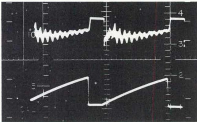
Waveforms of MAH-Q3—Base (Top) and Collector. Horizontal Time Base, Base Signal Is .9 Volt P-P.
