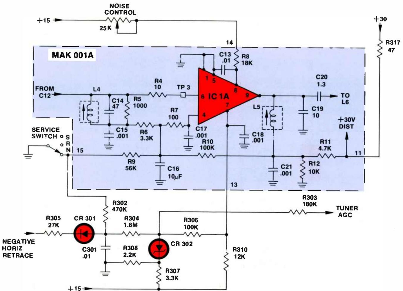
Figure 2-5 First and Second IF Amplifiers and AGC Circuits
