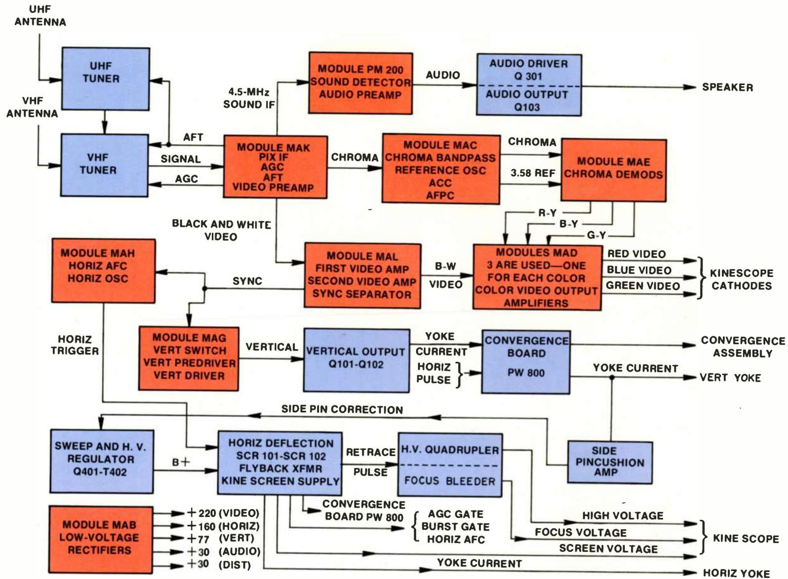
Figure 1-1 Functional Diagram of the RCA CTC 49
