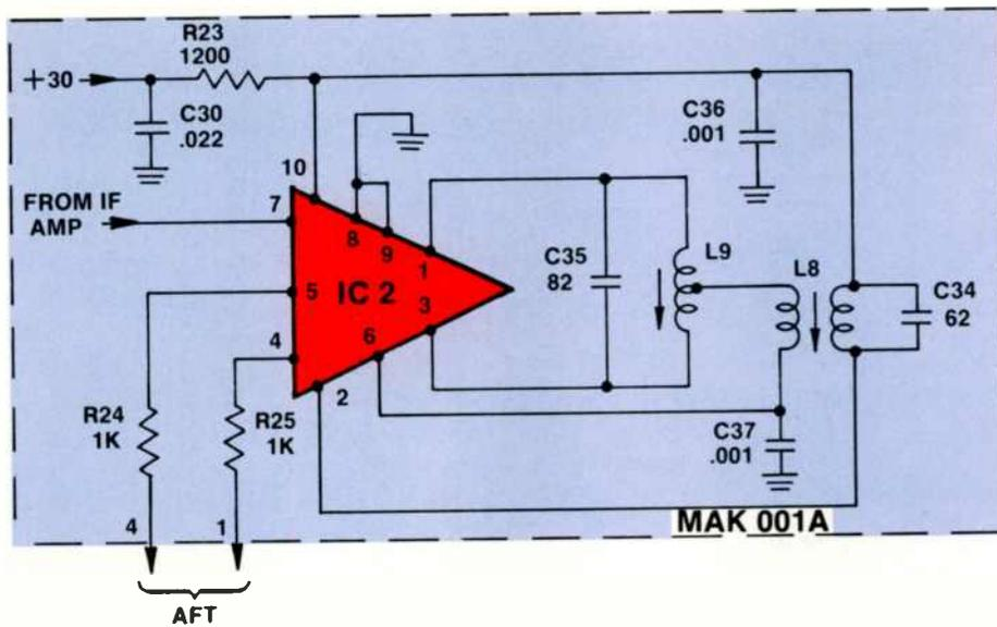
Figure 2-7 AFT Integrated Circuit and Discrete Components
