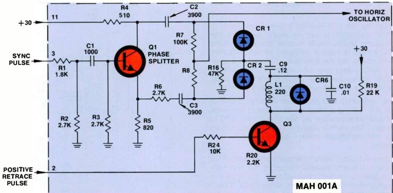
Figure 4-1 Horizontal AFC Circuit
