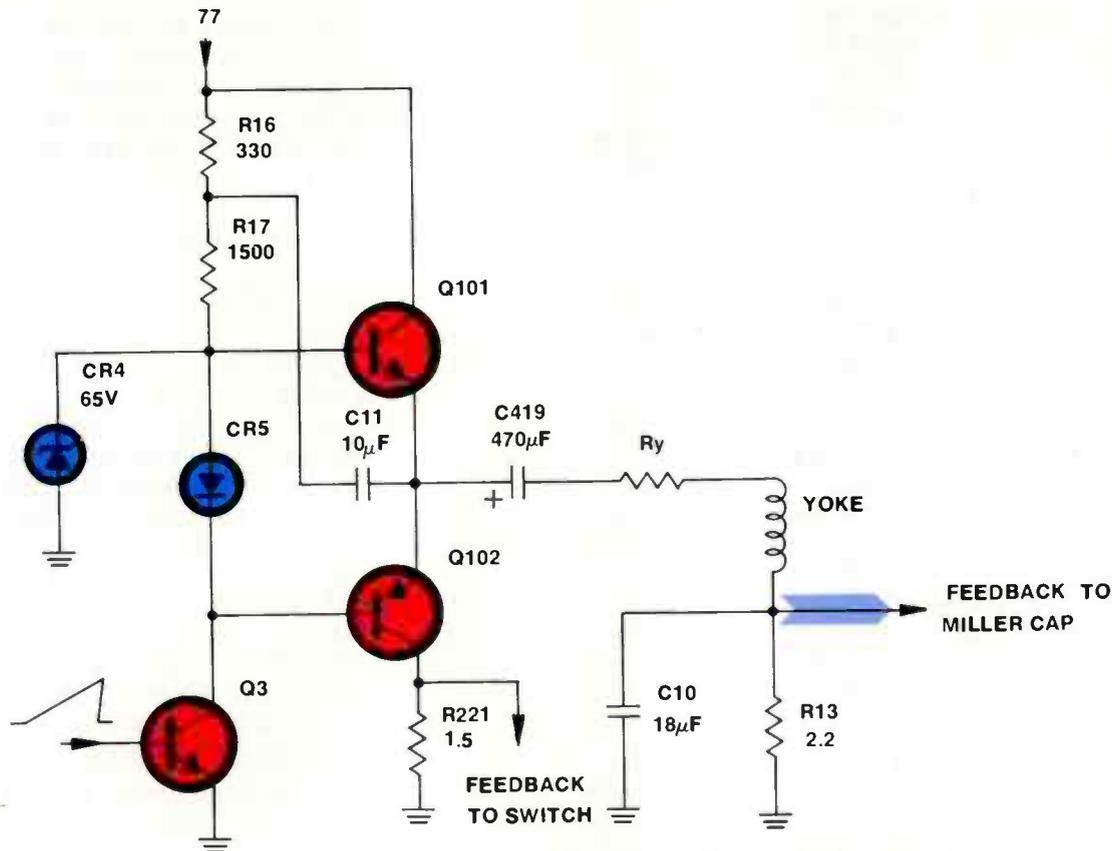
Figure 5-2 Vertical Driver, Output, and Simplified Yoke Circuit
