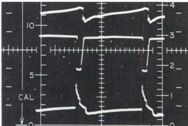
Waveforms of MAH-Q2 Base (Top), Collector, and MAH-5. P-P Volts Are 5, 30, and 9, Respectively
