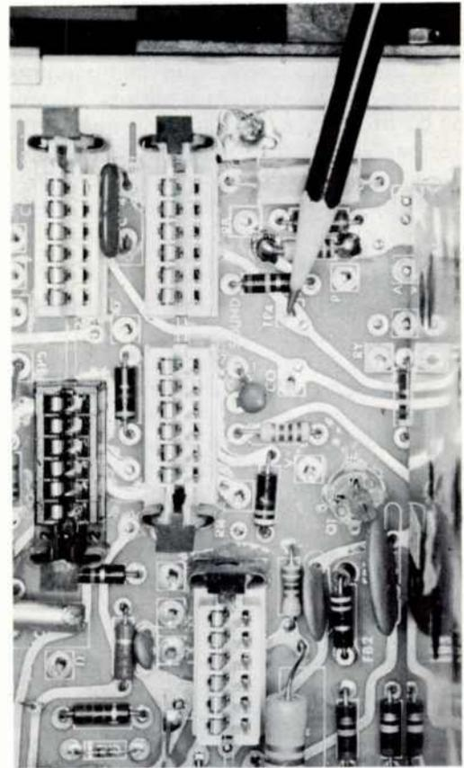
*The location of TP 304 is between Module MAK and PM 200. The DC level and the 4.5-MHz aural output from Module MAK may be checked here.*
