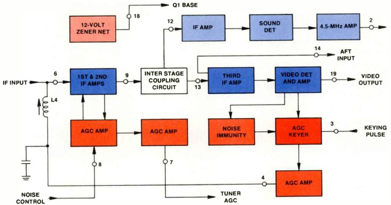
Figure 2-3 Functional Diagram of the IF/AGC Integrated Circuit
