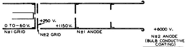
Fig. 4 - Electron gun used in type 1800.
