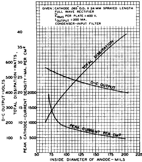
Fig. 12 - Effect of varying anode diameter in rectifier design.
