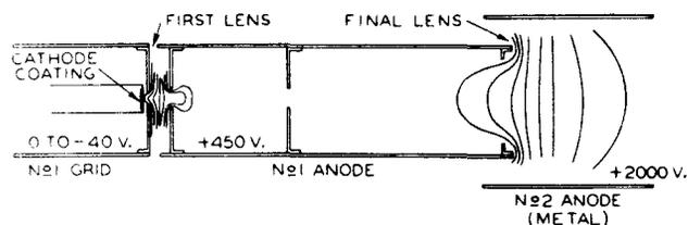
Fig. 1 - Electron gun used in type 905.
