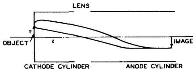
Fig. 17 - Cathode lens.
