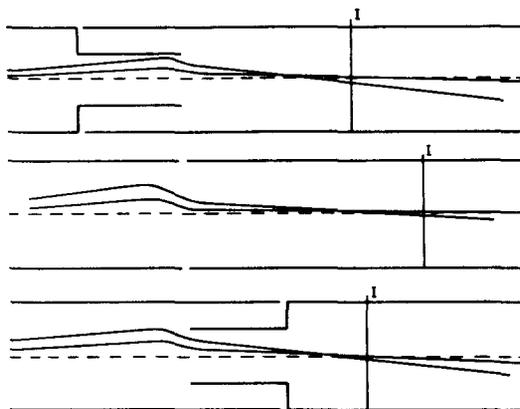
Fig. 9 - Aperture defect for cylinder lenses.
