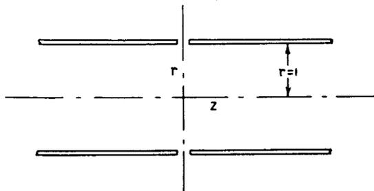
Fig. 14 - Coordinates for electrostatic cylinder lens.
