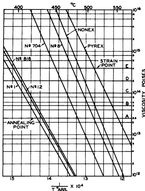
Fig. 4 - Viscosity of glasses between annealing and strain points. The intersection of lines A, B, C, D, and E with the viscosity curves for the various glasses indicate the temperature intervals at which the viscosities are doubled, as shown in the tabulation immediately preceding Table II.
