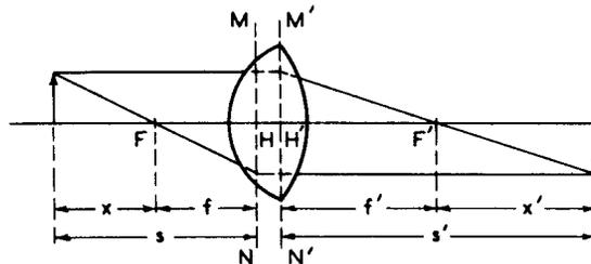
Fig. 5 - Image formation by a thick lens.
