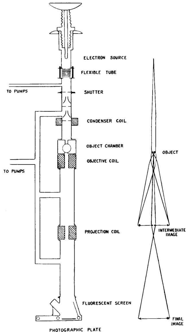
Fig. 1 - Electron microscope utilizing magnetic electron lenses.
