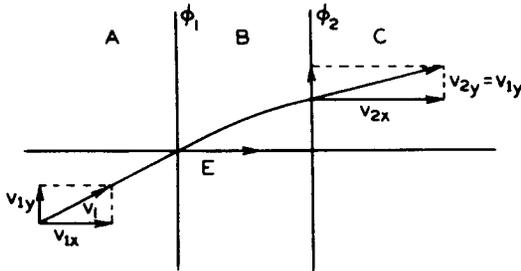
Fig. 7 - Refraction by potential double layer.
