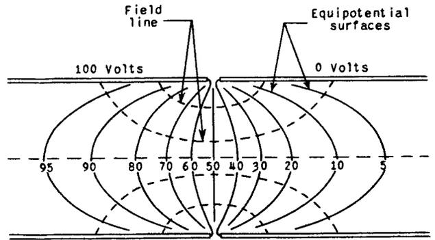
Fig. 2 - Potential distribution between two cylinders.
