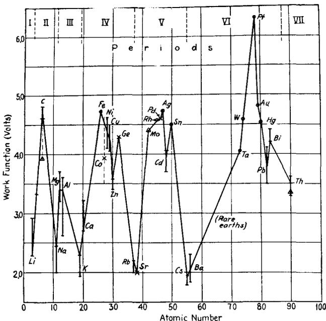
Fig. 5 - Variation of photoelectric work function throughout the periodic table. ○, values for clean surfaces. ×, single values of uncertain precision. △, reliable thermionic value (indicated only when photoelectric value is uncertain. |, vertical lines indicate approximate range covered by various reported values.
