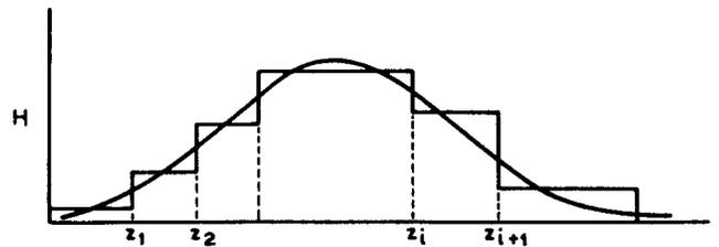
Fig. 22 - Approximate representation of axial magnetic field.
