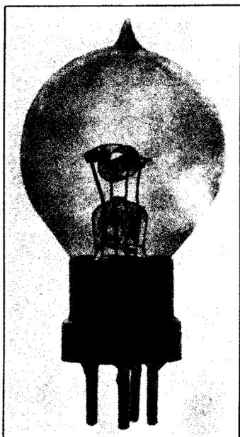
Fig. 7 - Three-electrode tube used by the French Army.
