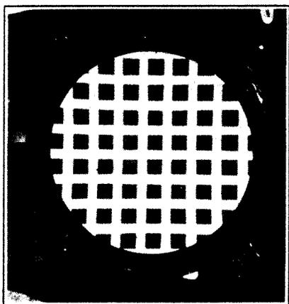
Fig. 11b - Image field of curved-cathode image tube.
