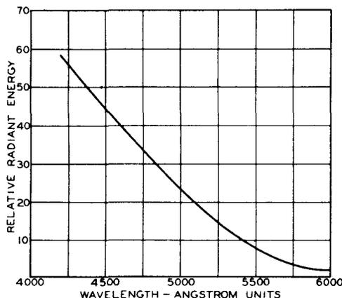
Fig. 9 - Spectral energy characteristic of phosphor No.5.
