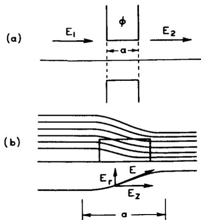
Fig. 9 - Idealized field distribution in simple aperture lens.
