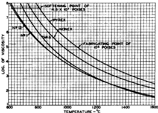
Fig. 3 - Viscosity curves of several glasses.
