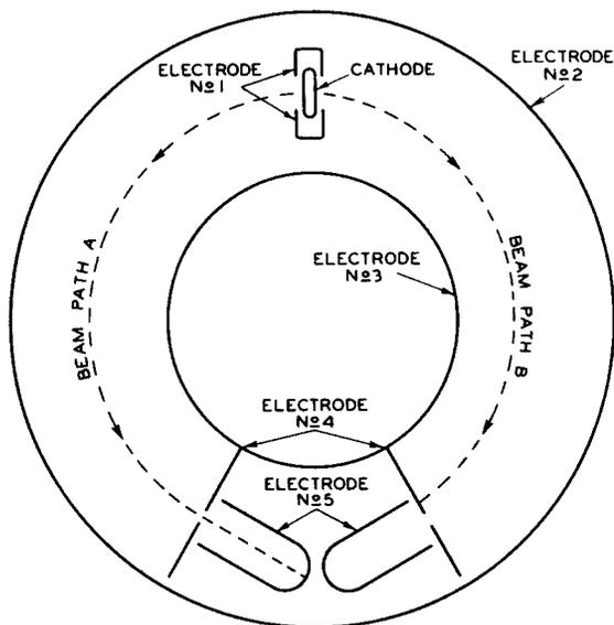
Fig. 14 - Orbital-beam-deflection amplifier.
