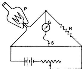
Fig. 11 - Electrical diagram of the Pirani gauge.
