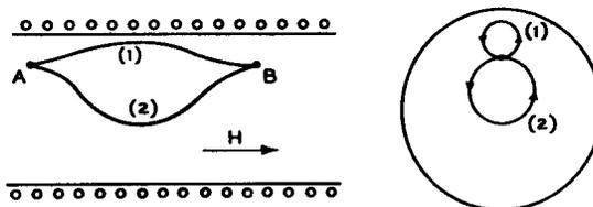
Fig. 21 - Electron paths in a uniform magnetic field.
