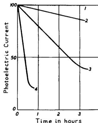
Fig. 12 - Decrease of current for a given  $Ag:Cs_2O, Ag-Cs$  cathode: 1, in infra-red light; 2, in red light; 3, in green light; 4, in blue light.
