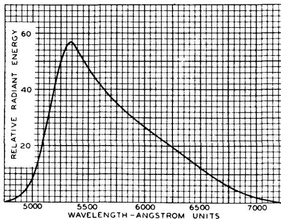
Fig. 5 - Spectral energy characteristic of phosphor No.3.
