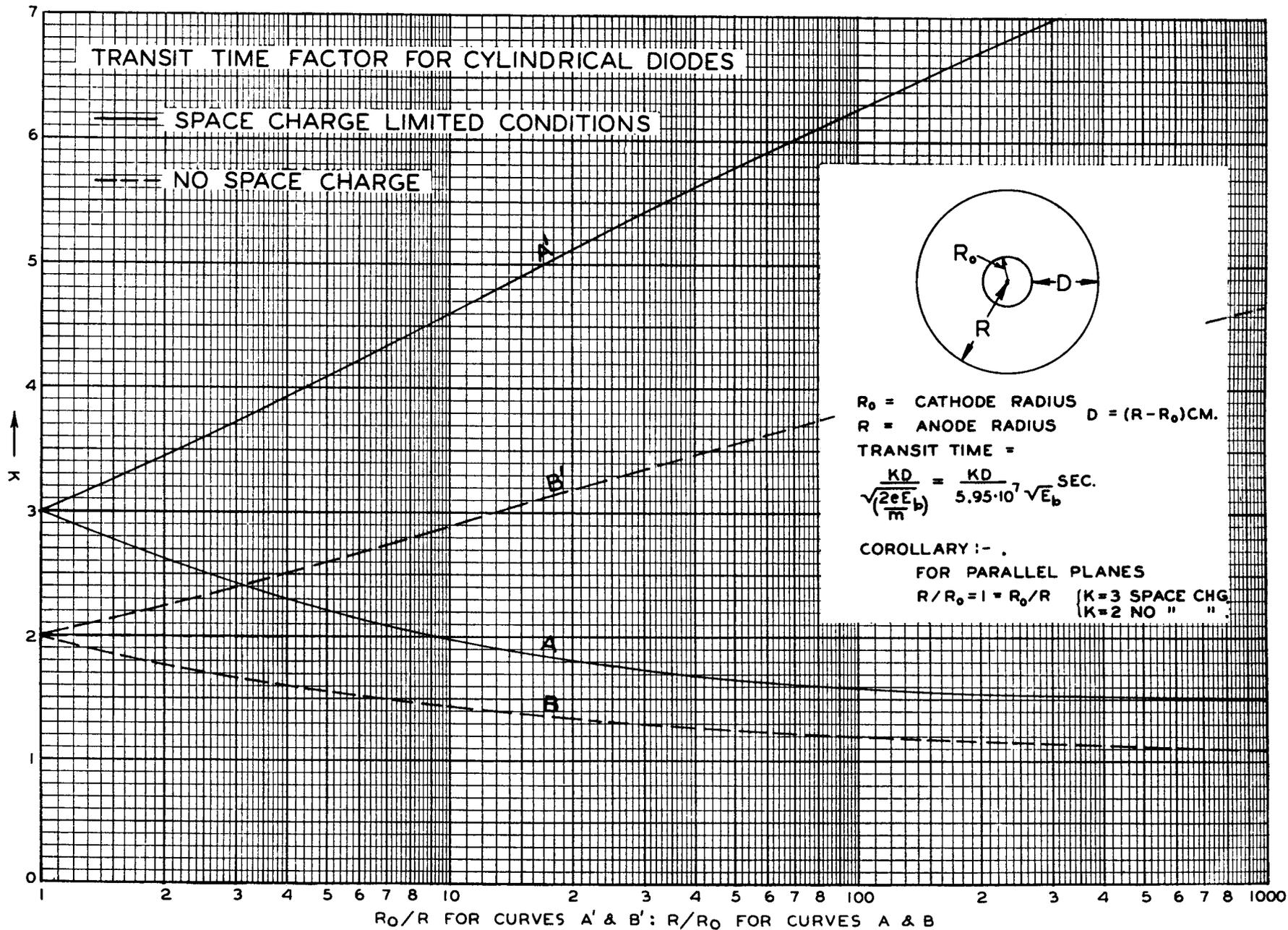
ting angle and plate swing. The minimum transit angle is determined with the aid of curves in Fig. 13.
