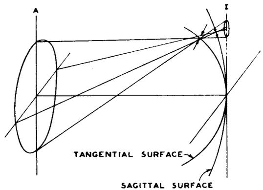
Fig. 4 - Curvature of field and astigmatism.
