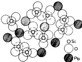
Fig. 2 - Atomic arrangement in lead-oxide silica glass.
