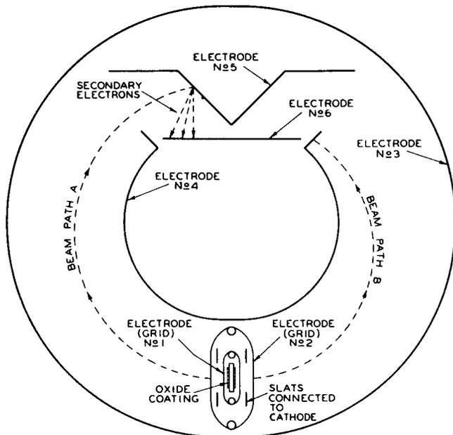
Fig. 16 - Orbital-beam frequency converter with secondary-electron multiplication.
