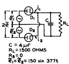
Fig. 13 (left) - Half-wave, condenser-input circuit without series resistance.
