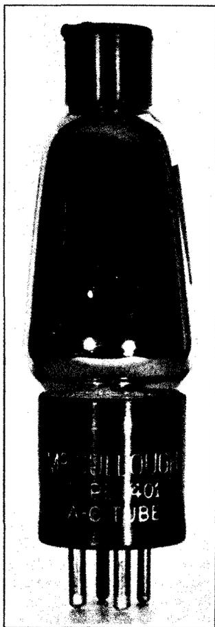
Fig. 17 - McCullough tube type with indirectly heated cathode.
