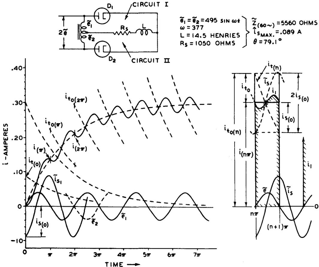
Fig. 9 - Full-wave choke-input circuit and its operation.
