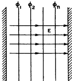
Fig. 1 - Potential and field between plates.
