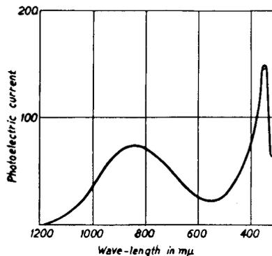
Fig. 20 - Representative spectral distribution curve of a Ag: Cs<sub>2</sub>O, Ag-Cs cathode with a surplus of Ag in the layer. S. Asao, Physics, 2, p. 19 (1932). Courtesy of American Physical Society.
