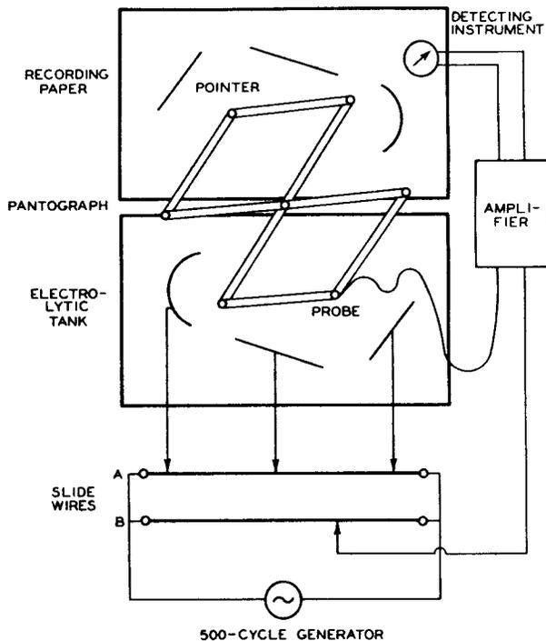
Fig. 3 - Diagram of potential plotting tank.
