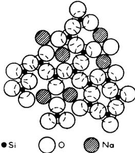
Fig. 1 - Schematic arrangement of atoms in a soda silica glass.
