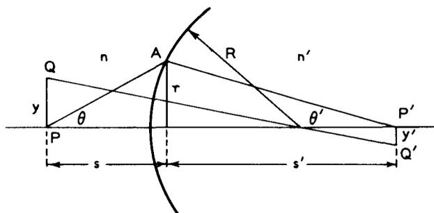
Fig. 3 - Refraction at a curved surface.
