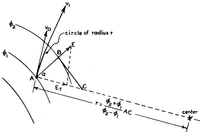
Fig. 5 - Circle method of graphical ray tracing.
