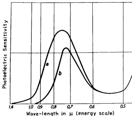
Fig. 13 - Spectral distribution curve of a Ag:Cs<sub>2</sub>O, Ag-Cs cathode: (a) in a fresh state; (b) after fatigue has set in.
