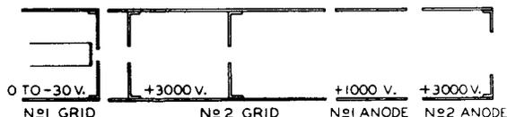
Fig. 5 - Electron gun with zero anode No.1 current.
