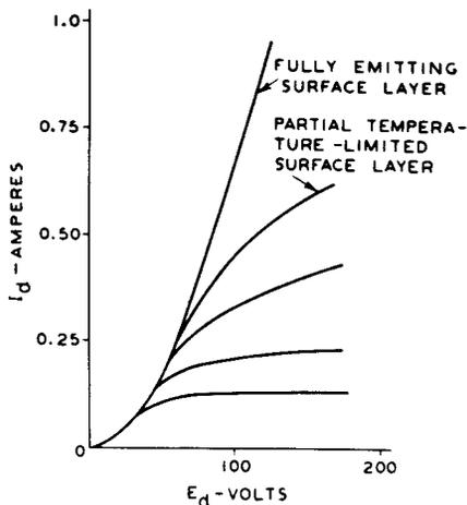
Fig. 5 - Single-valued saturation characteristic of diode with high coating conductance.
