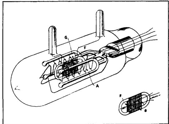
Fig. 4 - Tube constructed with filamentary electrodes.
