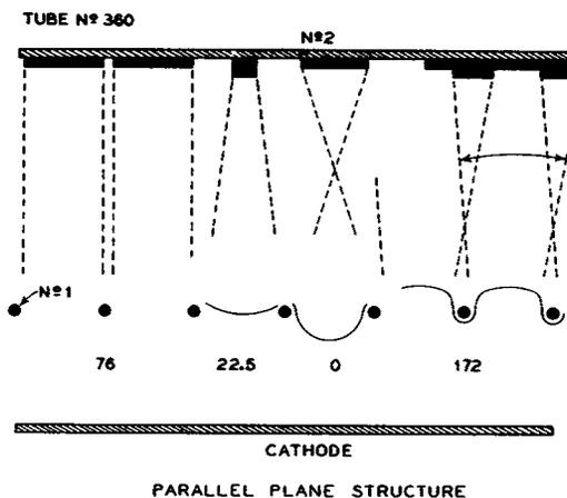
Fig. 9 - Beam formation by grid openings. No.2 volts = 250
