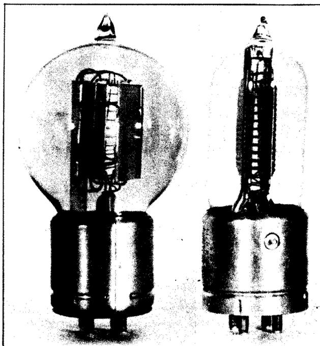
Fig. 8 - (left) Signal Corps tube type VT-1. (right) Signal Corps tube type VT-2.
