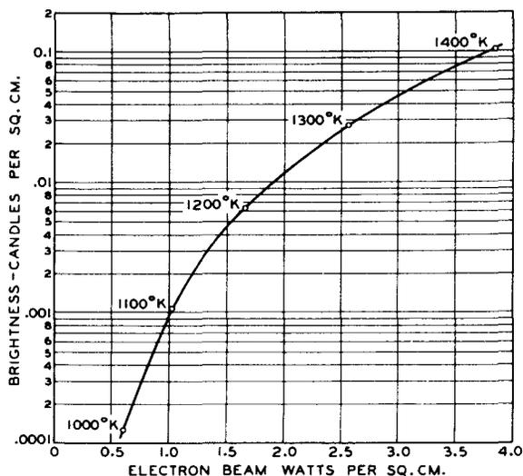
Fig. 1 - Indication of beam traces by incandescence of tungsten foil.
