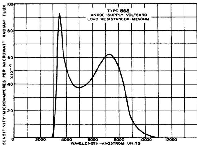
Fig. 17 - Spectral distribution curve for Type 868 caesium-oxide phototube.
