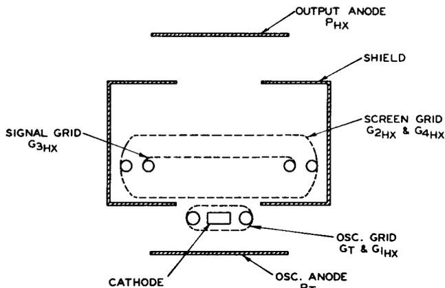
Fig. 9 - Cross-section of triode-hexode converter type 6K8.
