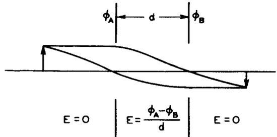
Fig. 10 - Ray paths in double-aperture lens (schematic).
