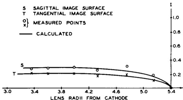
Fig. 10 - Curvature of field of image tube.
