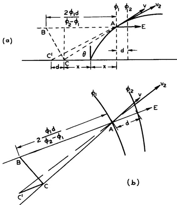
Fig. 6 - Parabola method of ray tracing.
