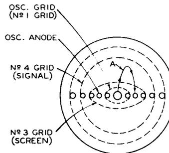
Fig. 8 - Cross-section of pentagrid converter (6A8).
