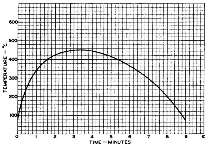
Fig. 8 - Typical annealing curve for glass stems.
