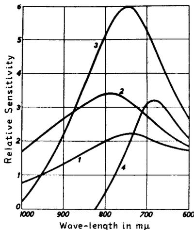
Fig. 19 - Several spectral distribution curves of Ag: Cs<sub>2</sub>O, Ag-Cs photocathodes with different amounts of adsorbed Cs atoms. The amount of Cs increases from curve 1 to curve 4. C. H. Prescott, Jr. and M. J. Kelly, Bell System Tech. Jour. 11, 334 (1932). Courtesy of American Telephone & Telegraph Company.
