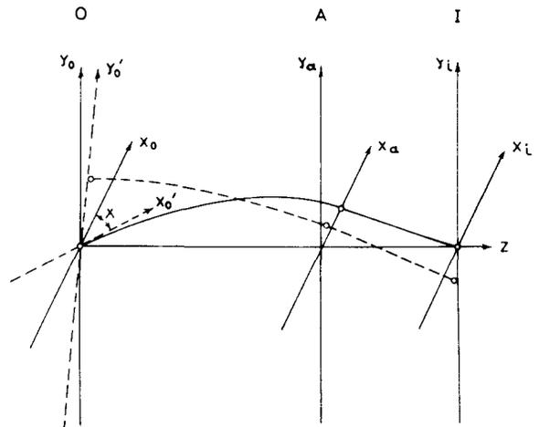
Fig. 1 - Object, aperture, and image planes.
