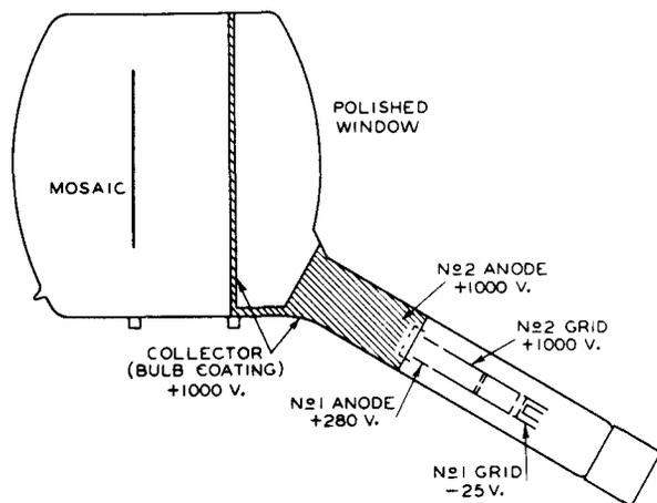
Fig. 7 - Iconoscope outline and electron gun.
