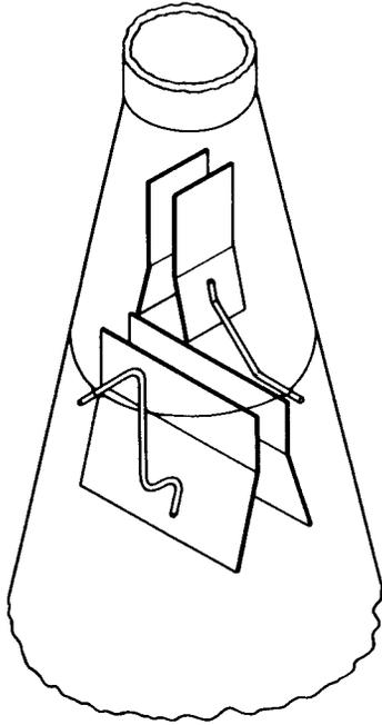
Fig. 2 - Deflecting-plate structure of type 905.
