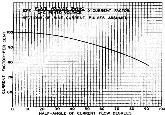
Fig. 7 - Class B and C amplifier efficiency.
