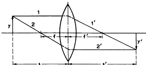
Fig. 4 - Properties of a thin lens.
