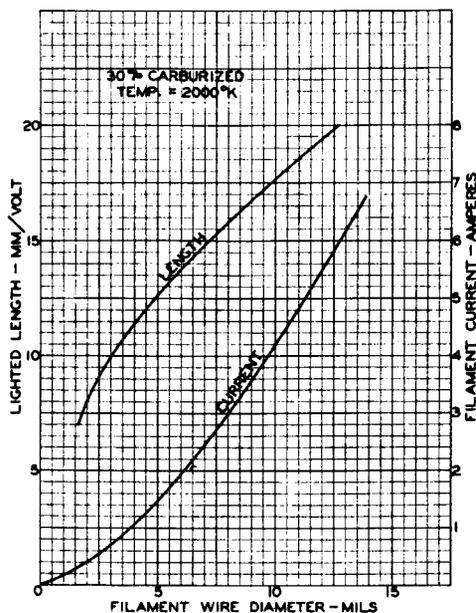
Fig. 15 - Design curves of thoriated-tungsten filaments.
