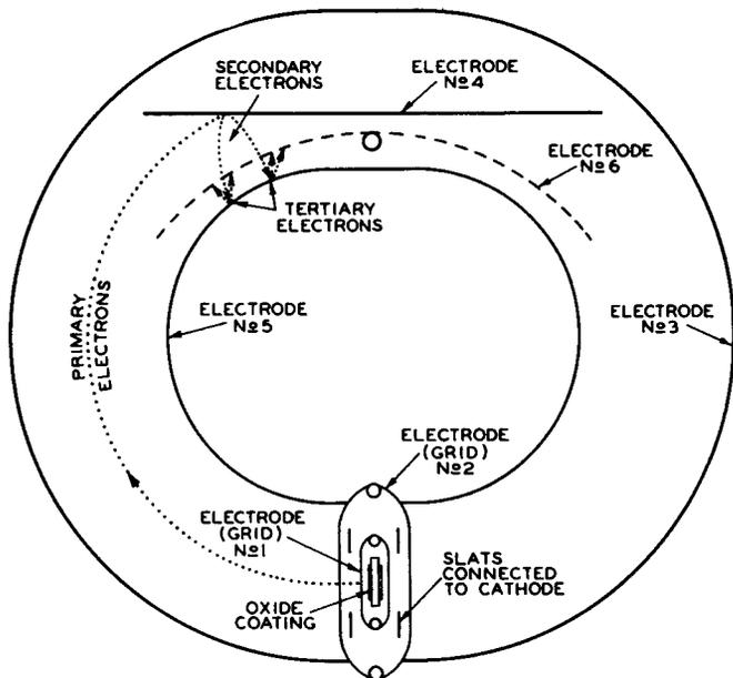
Fig. 15 - Two-stage, orbital-beam, electrostatic-type, electron multiplier.
