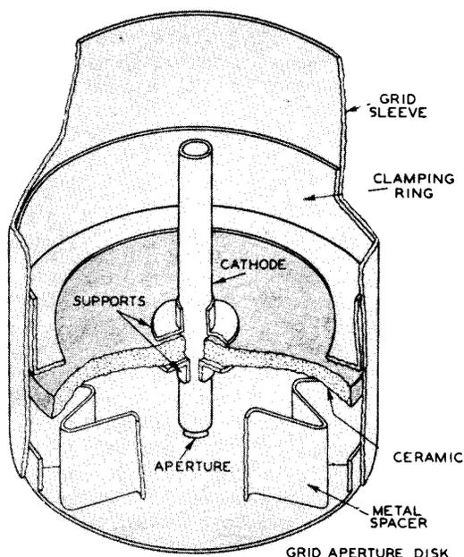
Fig. 9 - Ceramic-supported cathode.
