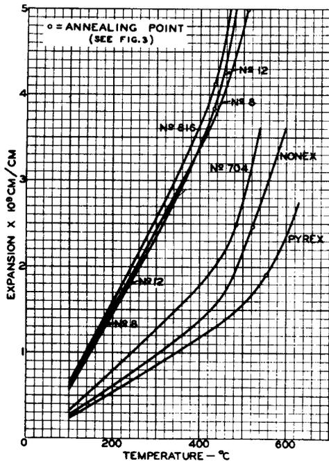
Fig. 9 - Expansion curves of various glasses.
