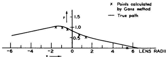
Fig. 13 - Electron trajectory through cylinder lens.
