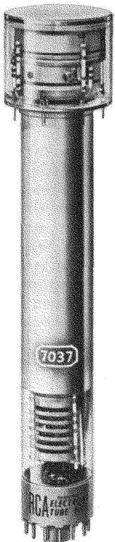
grid (grid No.6) to provide an electrostatic accelerating field, and a target which consists of a thin glass disc with a fine mesh screen very closely spaced to it on the photocathode side. Focusing is accomplished by means of a magnetic field produced by an external coil, and by varying the photocathode voltage.
