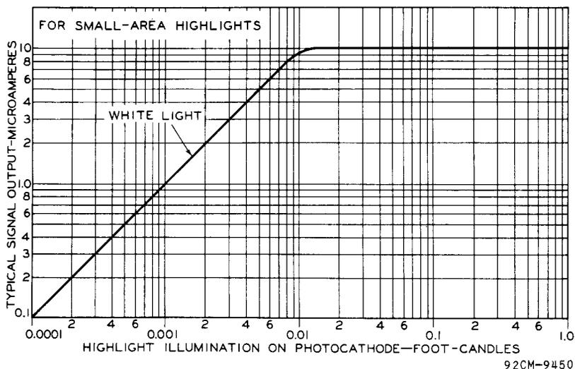
Fig. 4 - Basic Light Transfer Characteristic of Type 7037.
