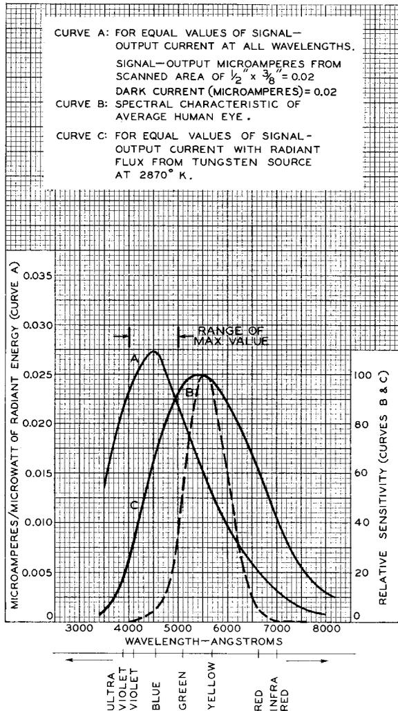
Fig. 12 - Spectral Sensitivity Characteristics of Type 7038.
