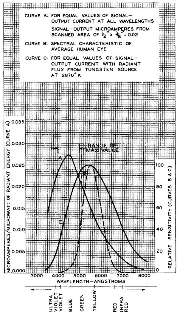
Fig. 7 - Spectral Sensitivity Characteristic of Type 6198.
