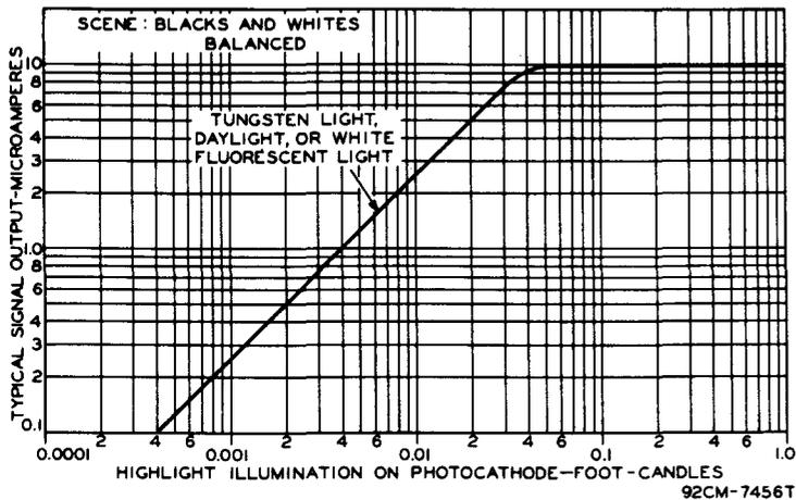
Fig. 5 - Typical Signal Output of Type 5826.
