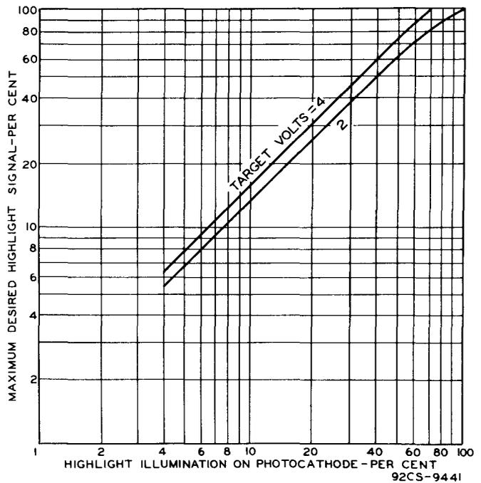
Fig. 5 - Light Transfer Characteristics of Type 7037.
