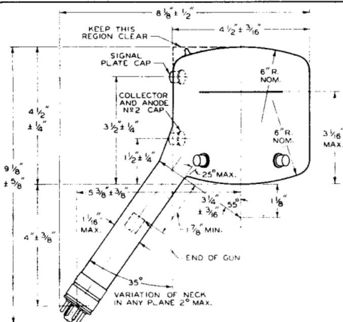
CAPS A,B,C & D — MAKE NO CONNECTIONS TO THESE CAPS—USED ONLY DURING MANUFACTURE OF TUBE
