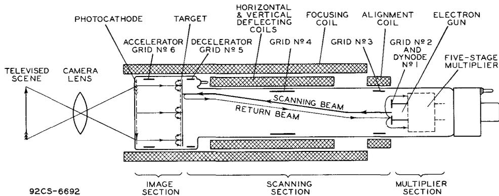
Fig. 2 - Schematic Arrangement of Type 7037.
