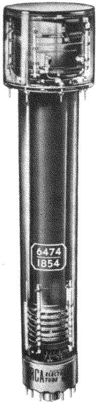
The 6474 has exceptional sensitivity combined with a spectral response approaching that of the eye, and good resolution capability. With a color camera employing a suitably designed optical system and utilizing efficient color filters, commercially acceptable color pictures can be obtained with about 350 foot-candles of incident incandescent illumination on the scene and a lens stop of f:5.6.
