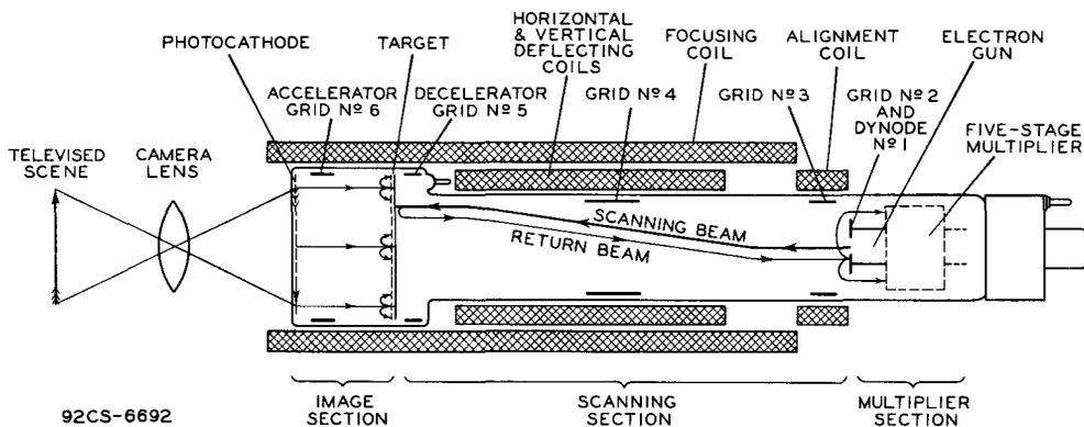
Fig. 1 - Schematic Arrangement of Type 6474.
