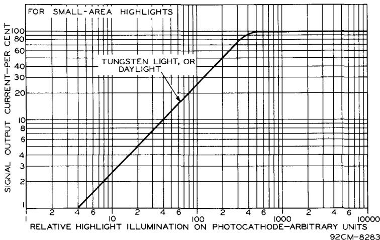
Fig. 6 - Basic Light Transfer Characteristic of Type 6474.
