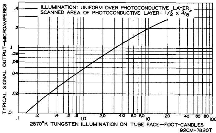
Fig. 5 - Typical Signal Output of Type 6198.
