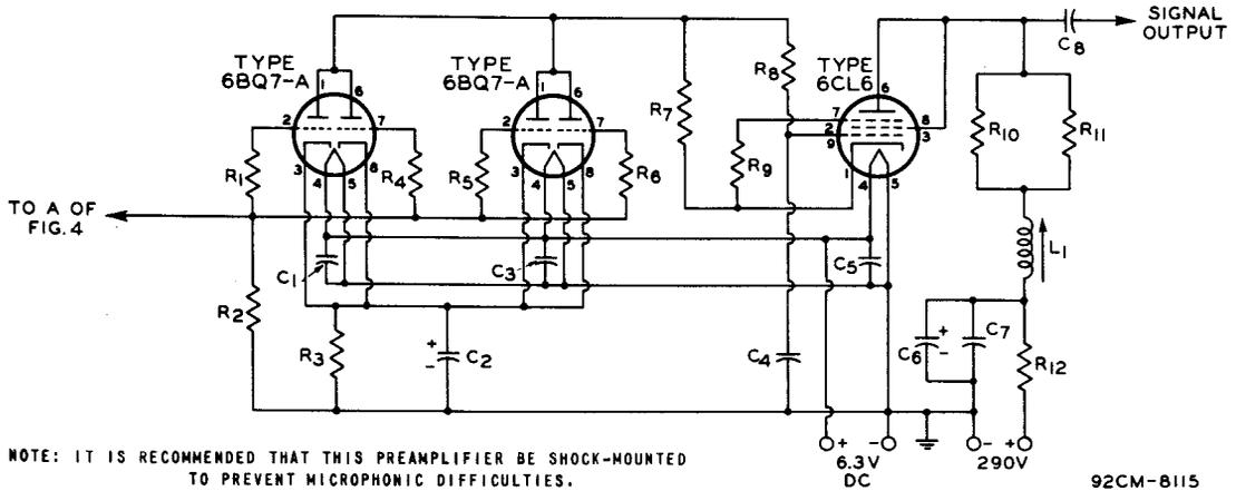
NOTE: IT IS RECOMMENDED THAT THIS PREAMPLIFIER BE SHOCK-MOUNTED TO PREVENT MICROPHONIC DIFFICULTIES.
