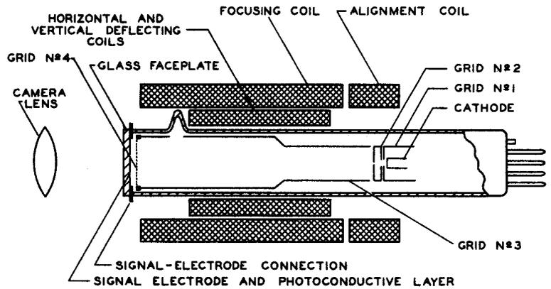
Fig. 1 - Schematic Arrangement of Type 6198.
