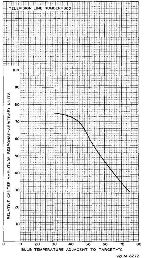
Fig. 5 - Temperature Effect on Amplitude Response of Type 6474.
