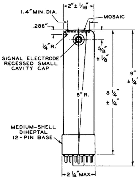
☉ OF BULB WILL NOT DEVIATE MORE THAN  $2^\circ$  IN ANY DIRECTION FROM THE PERPENDICULAR ERECTED AT THE CENTER OF BOTTOM OF THE BASE.
