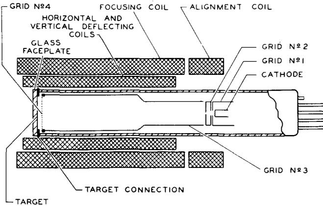
Fig. 1 - Schematic Arrangement of Type 7038.
