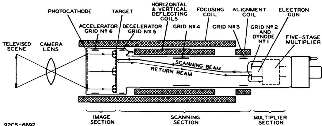
Fig. 1 - Schematic Arrangement of Type 5826.
