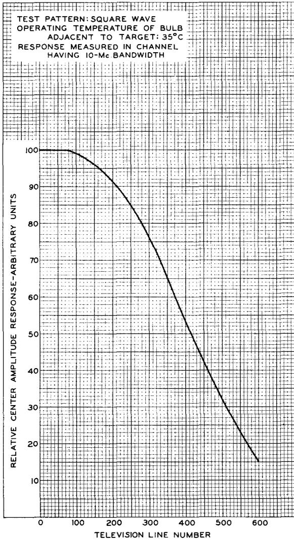
Fig. 4 - Amplitude Response Characteristic of Type 6474.
