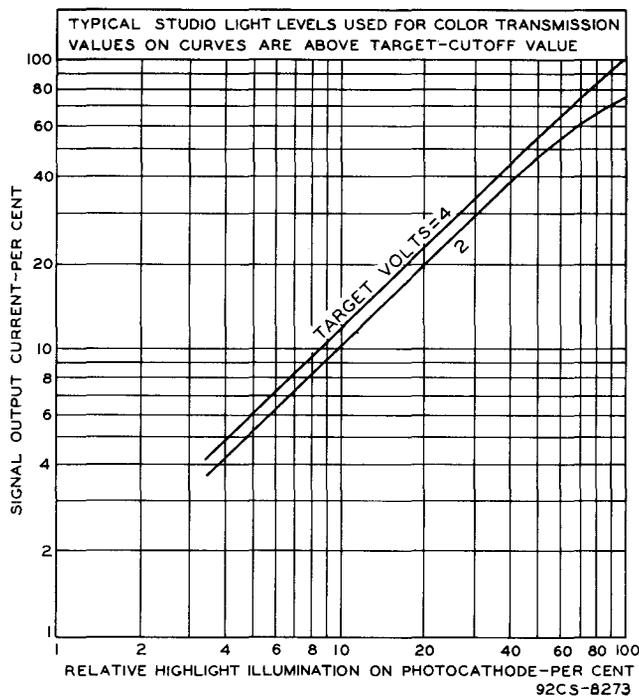
Fig.7 - Light Transfer Characteristics of Type 6474.
