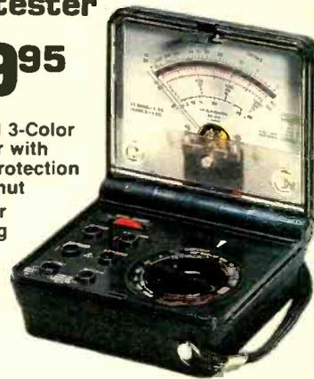
Fuse/surge-absorber protected. Sensitivity: 20,000 ohms per volt DC. Measures to 1200 volts DC in seven ranges, 1200 volts AC in five ranges, DC current to 300 mA in four ranges. Resistance to two megohms. dB: -20 to +63 in five ranges. Accuracy ±3% DC, ±4% AC. Open 7<sup>1</sup>/<sub>4</sub> x 4<sup>5</sup>/<sub>16</sub> x 1<sup>1</sup>/<sub>4</sub>". Requires "AA" battery. 22-211 ..... 29.95
