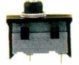
Mounts in single 3/8" hole. Rated 2 amps at 120 VAC. Trips within 120 seconds at 3 1/2 amps. 1 3/16 x 1/2 x 1 1/16" U.L. recognized. 270-1310 1.99
