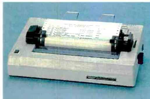
**DMP 106.** Ideal for data processing and general-purpose use. Bi-directional—prints 80 upper and lowercase letters per line (8 x 9 matrix) at 43 lines per minute (at 10 characters per inch). Elongated and condensed modes. Removable adjustable tractor. Parallel and Color Computer-compatible serial interfaces. UL listed AC. 26-2802 ..... **219.95**
