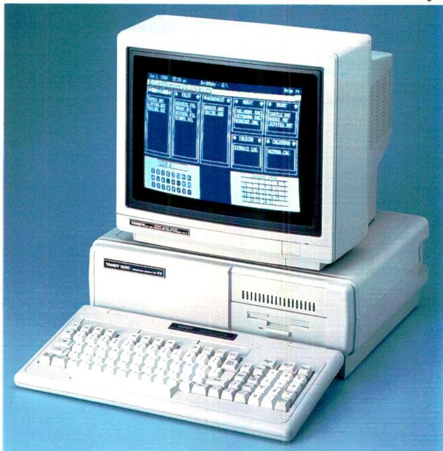
**Tandy 1000 TX.** Features an 8 MHz 80286 microprocessor for far greater processing power than ordinary PCs. This brings true 16-bit technology, previously found only in "AT" class machines, to an affordable PC—you'll fly through your applications!
