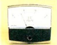
Just right for monitoring car electrical system or power supply voltage. Jeweled movement. Accuracy, ± 5% full scale. 2 3/4 x 2 1/4 x 1 1/4" 17/8" round mtg. hole. 270-1754 7.95
